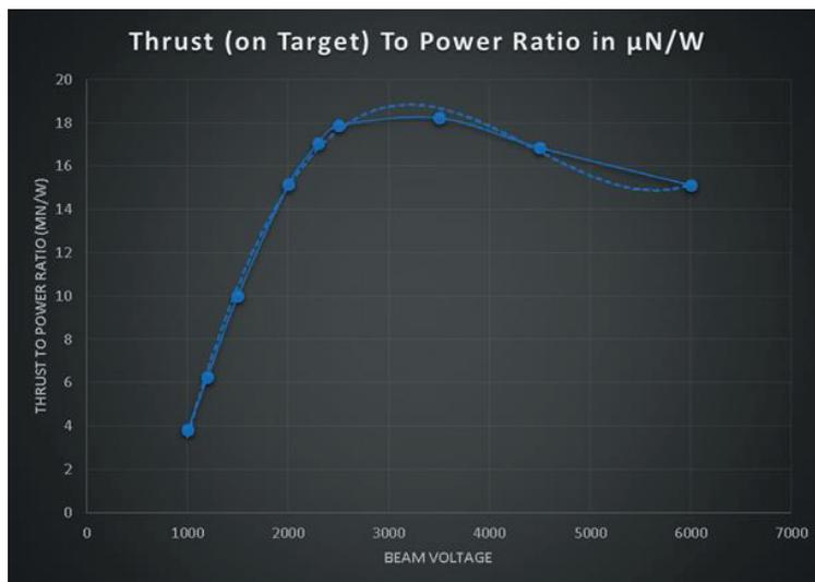
Figure 5. the ratio of transferred thrust to Power ratio as a function of the beam voltage
