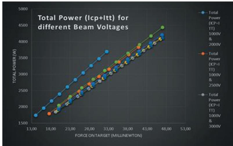
Figure 3. The total power consumption of the propulsion system (ITT and ICT) as a function of transferred thrust to the target for different beam voltages
