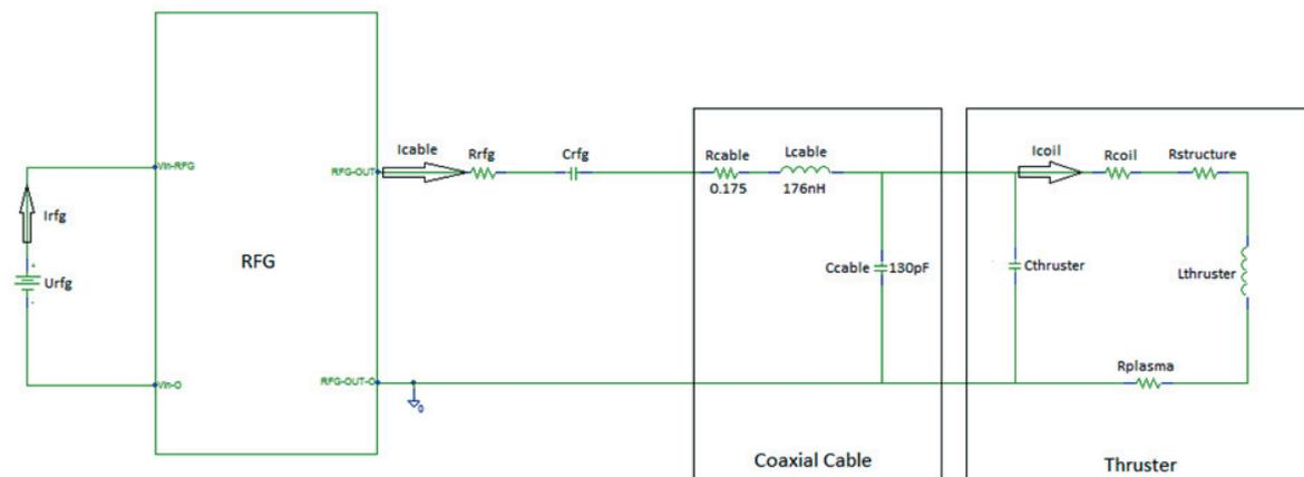
Figure 7: RF circuitry schematics including coaxial cable and thruster.
