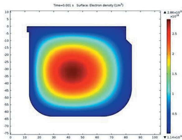
Figure 6: Plasma density distribution inside the thruster.
