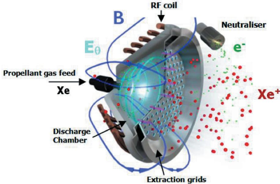
Figure 1: Operating principle of a Radio Frequency Ion Thruster<sup>10</sup>.
