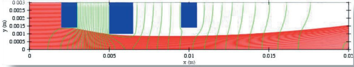
**Figure 1: Schematics indicating ion extraction through a grid aperture.**
