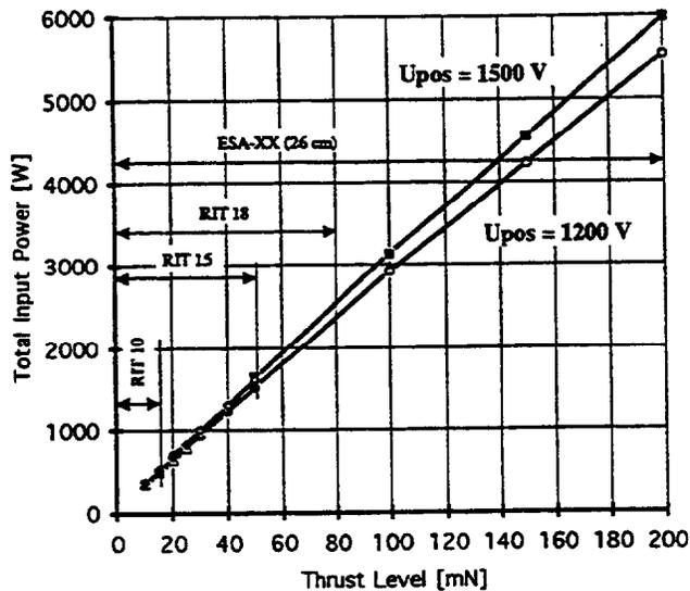
Fig. 6-1: Total Power Input for RITA Thrusters
