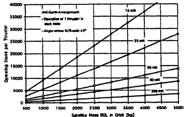
Fig. 4-2: Lifetime of thrusters
