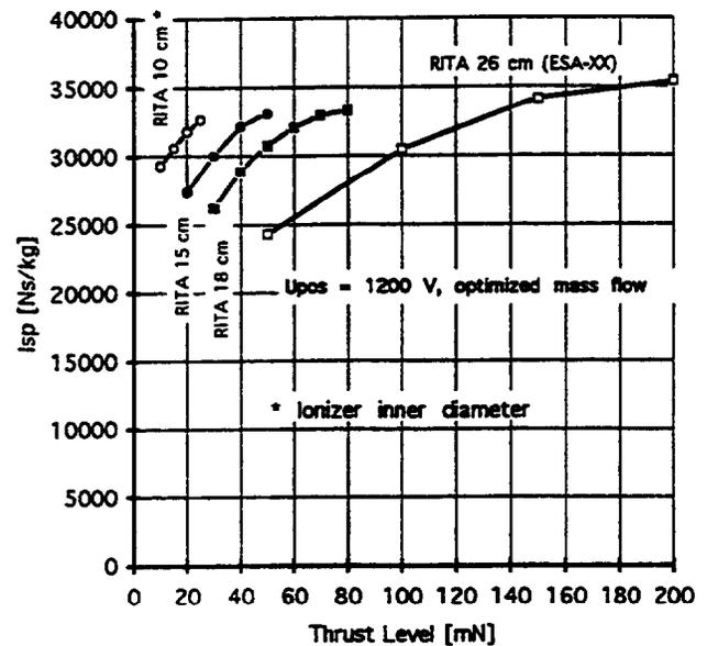
Fig. 6-2: Total Specific Impulse for RITA Thrusters
