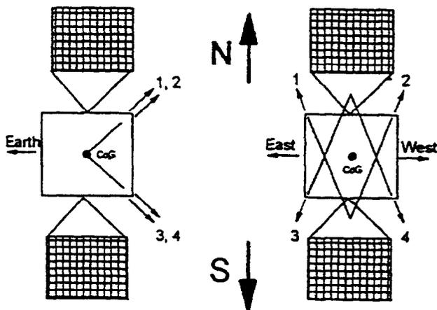
Fig. 4-1: Thruster Arrangements for NSSK
