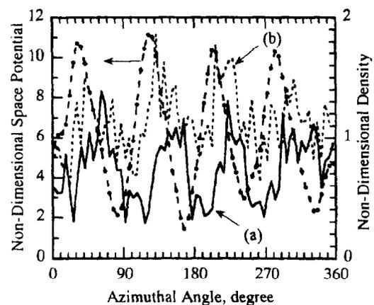
Fig. 5 Distributions of the space potential and densities of (a) electron and (b) ion obtained by the particle simulation on the same condition as Fig. 3(a).
