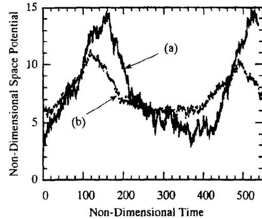
Fig. 4 Oscillation of the space potential at one position on the same condition as in Fig. 3 when the wall potential is (a) floating and (b) fixed.
