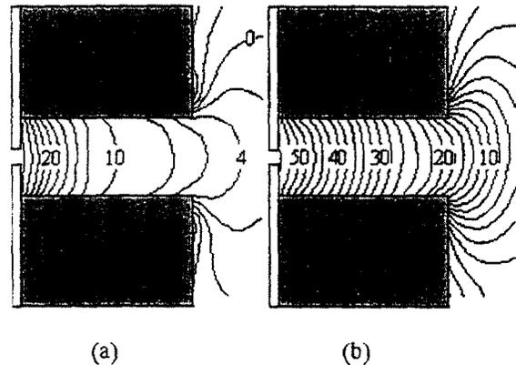
Fig. 9 Space potential distributions (in the dimensionless unit) obtained by the particle simulation when the channel walls are insulated ( $L=8$  mm,  $r_1=25$  mm,  $r_2=30$  mm,  $\gamma=0.2$ ,  $K_n=0.4$ , and  $\delta=0.6$ ): (a) with an oscillating electric field ( $\bar{\phi}_{1m}=6$ ,  $k_\theta \bar{r}=4$ ,  $\tilde{\omega}=2\pi/400$ ) and (b) without an
