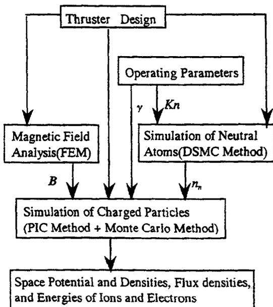
Fig. 1 Block diagram of the particle simulation.
