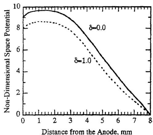
Fig. 11 Effect of the secondary-electron emission on the space potential distribution at  $r=\bar{r}$  ( $\bar{\phi}_{1m}=0$ ,  $L=8$  mm,  $r_1=19$  mm,  $r_2=25$  mm,  $\gamma=0.3$ ,  $K_n=0.3$ ).
