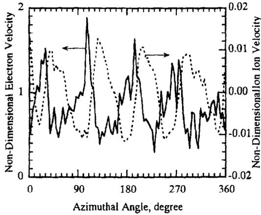
Fig. 6 Azimuthal velocity distributions of (a) electron and (b) ion obtained by the particle simulation on the same condition as Fig. 3(a).
