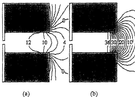
Fig. 10 Space potential distributions (in the dimensionless unit) obtained by the particle simulation when the channel walls are the anodes ( $L=8$  mm,  $r_1=25$  mm,  $r_2=30$  mm,  $\gamma=0.2$ ,  $K_n=0.4$ , and  $\delta=0.6$ ): (a) with an oscillating electric field ( $\bar{\phi}_{1m}=6$ ,  $k_\theta\bar{r}=4$ ,  $\bar{\omega}=2\pi/400$ ) and (b) without an oscillating field.
