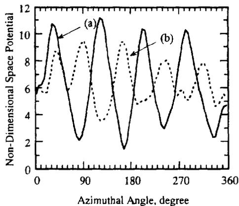
Fig. 3 Space potential distributions at  $r = \bar{r}$  obtained by the particle simulation ( $L=8$  mm,  $r_1=19$  mm,  $r_2=25$  mm,  $\gamma=1.0$ ,  $K_n=0.3$ , and  $V_a=50$  V), when the wall potential is (a) floating and (b) fixed.
