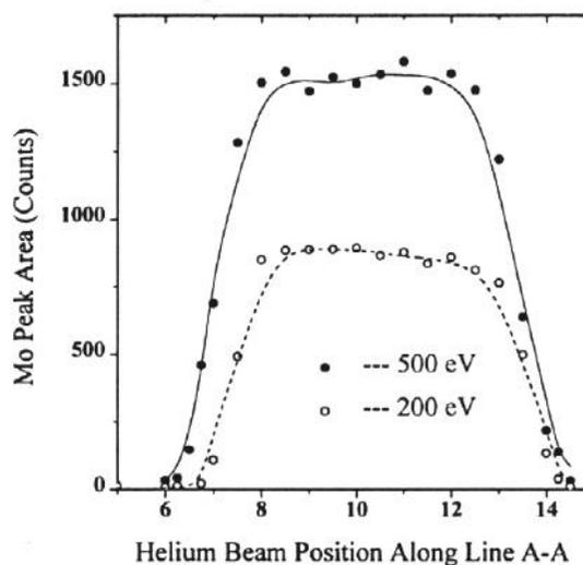
Fig. 4. Mo peak area as a function of He beam position across the foil at A-A.
