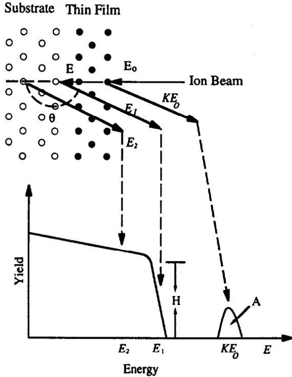
Fig. 1. Schematic diagram depicting the RBS technique.
