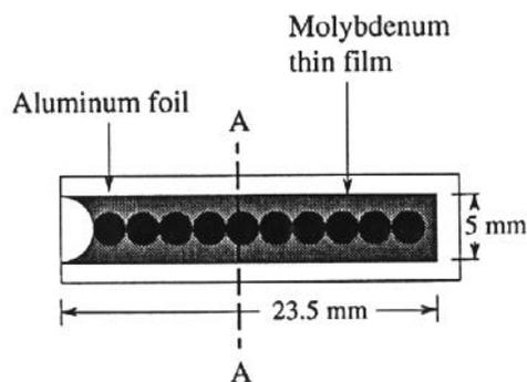
Fig. 3. Location of RBS measurements on the collector foil
