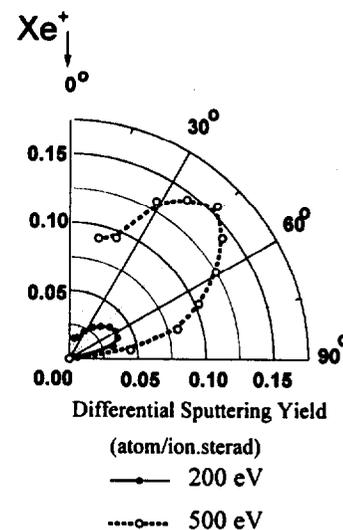
Fig. 6. Polar plot of the differential sputtering yield of Mo at 200 and 500 eV.
