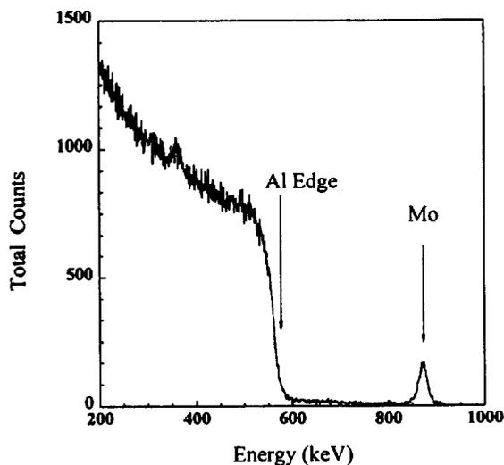
Fig. 5. A typical RBS spectrum from Mo deposited on Al foil.
