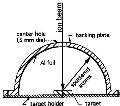
Fig. 2. Schematic diagram of the target-collector assembly.
