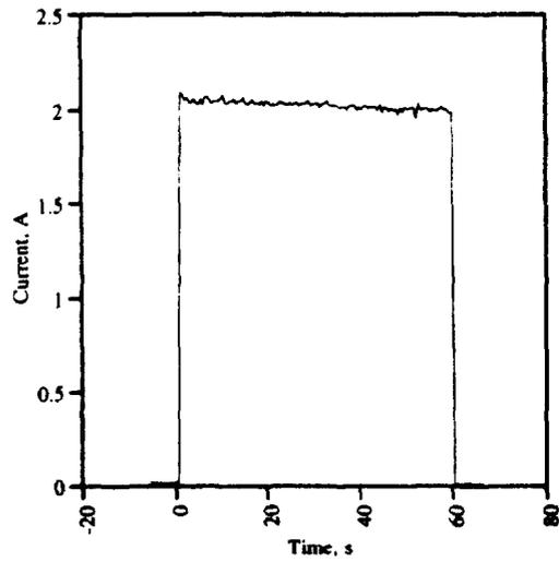
Figure 2. -Current as a function of time, 60 s duration.
