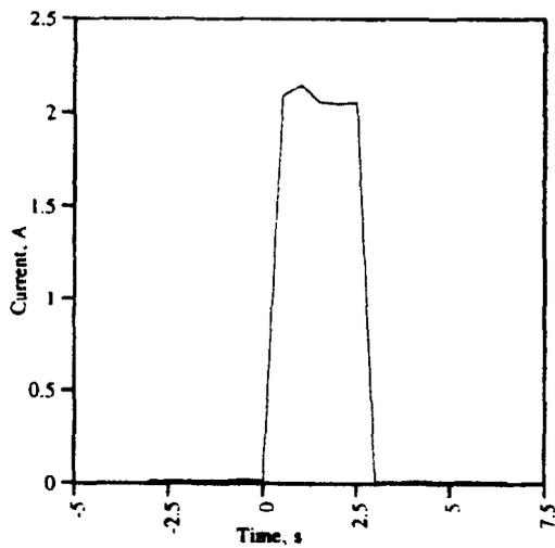
Figure 5. -Current as a function of time, 3 s duration.
