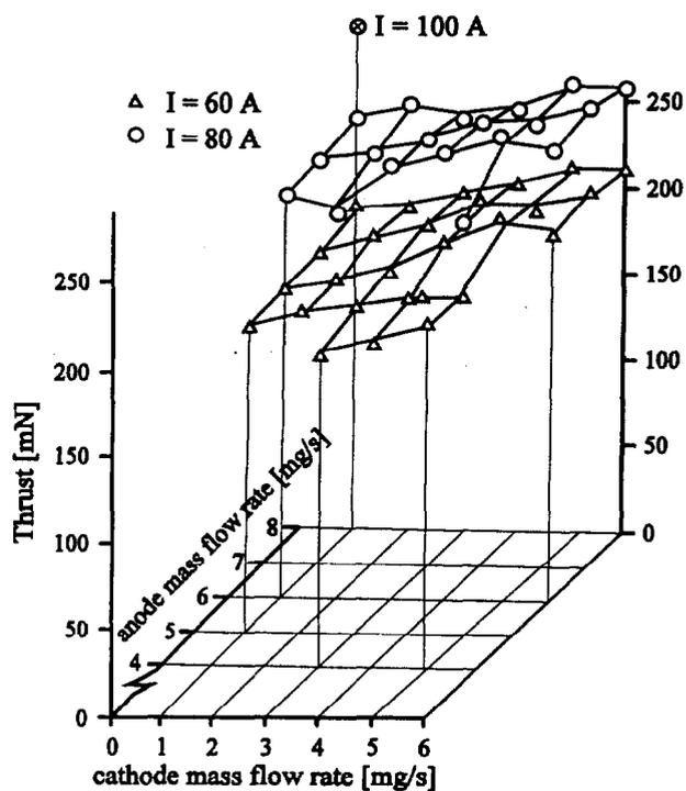
Fig. 3b: Thrust as a function of anode and cathode mass fractions (pre flight type X16<sup>12</sup>)
