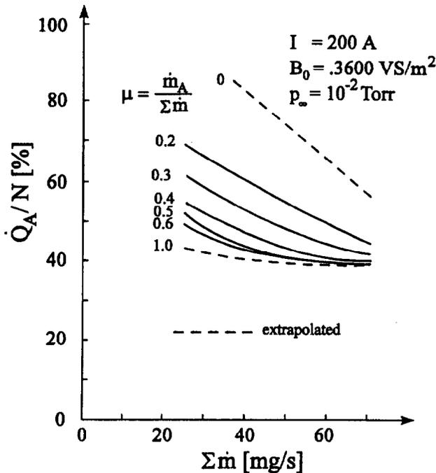
Fig. 4.: Relative anode loss as function of mass flow<sup>22</sup>
