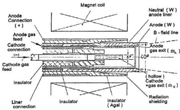
Fig.7: 12 kW radiat. cooled MPD thruster X16<sup>12</sup>
