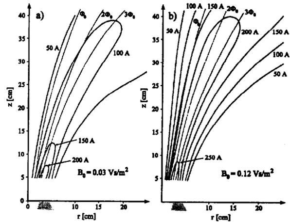
Fig. 5: Discharge current distribution at different magnetic field strength (X9, 100 mg/s Ar,  $p_{\infty} = 2$  Pa)<sup>24</sup>
