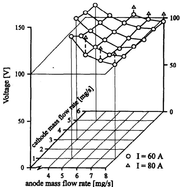
Fig. 3a: Voltage as function of anode and cathode mass fractions (preflight type X16, argon<sup>12</sup>)
