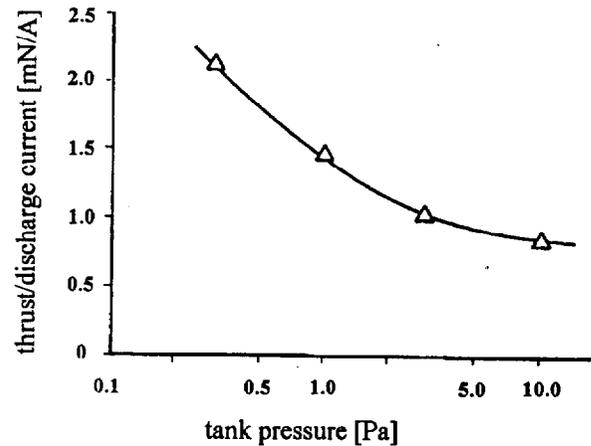
Fig. 6: Thrust per current as function of the tank pressure<sup>12,22</sup>
