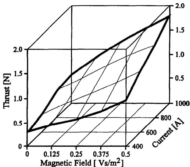
Fig. 2: Thrust as function of discharge current and magnetic field strength<sup>10</sup> (elevated power laboratory type X9, 100 mg/s argon,  $p_a = 3.0\text{Pa}$ )
