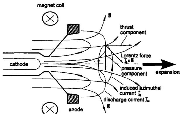
Fig. 1: Principle of an MPD thruster with applied magnetic field
