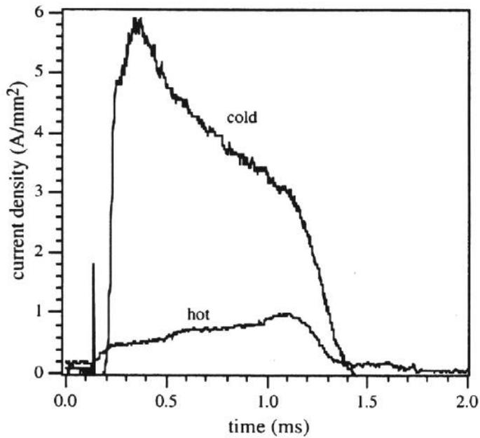
Fig. 2 Current density on the 1C zone (cathode tip) with and without cathode heating
