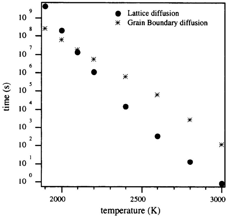
Fig. 7 Thorium coverage depletion time vs temperature in vacuum conditions
