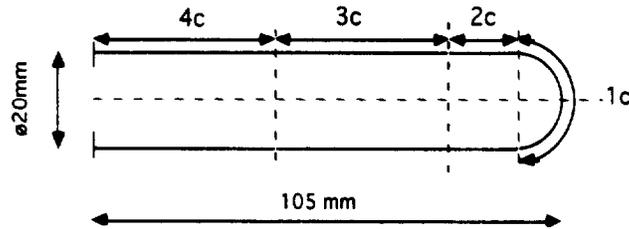
Fig. 6 Cathode zones (see Refs. 10 and 11 for details on current density measurements)
