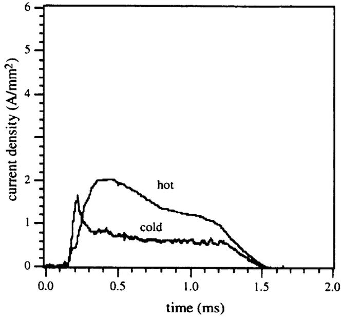
Fig. 4 Current density on the 3C zone with and without cathode heating
