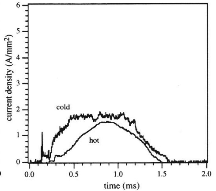
Fig. 3 Current density on the 2C zone with and without cathode heating
