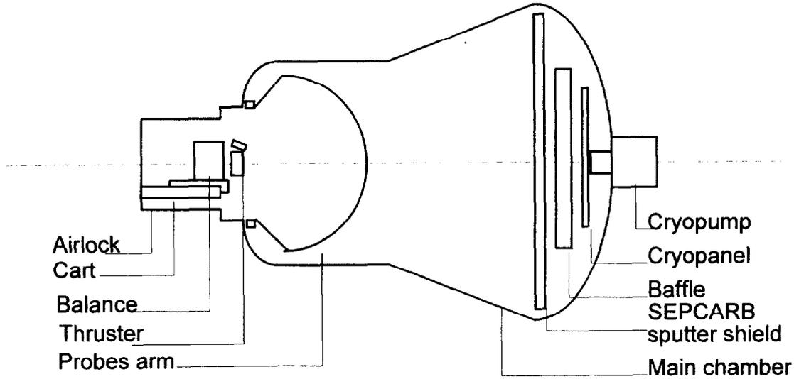
Figure 3: LIB test facility
