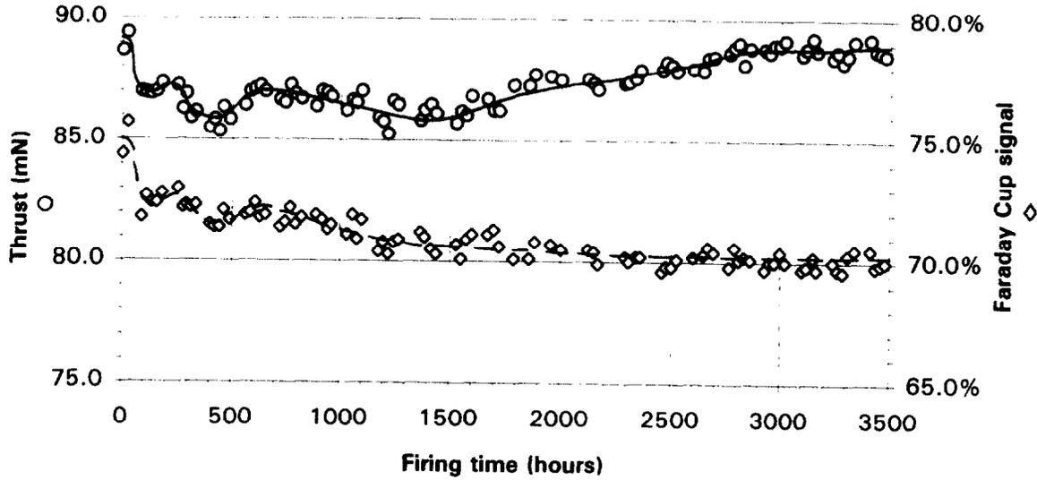
Figure 4: thrust versus time in hours (3500 h test) ↑
