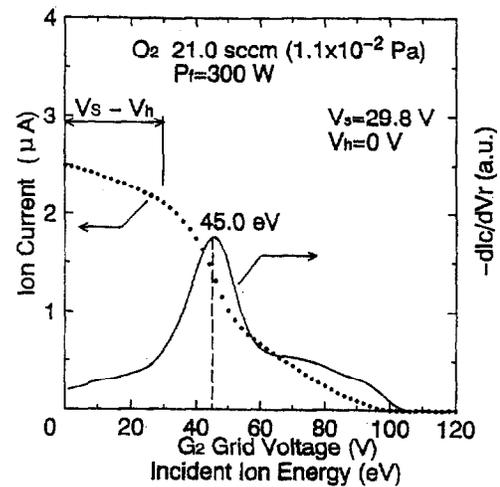
Fig.6 Typical ion collector current and its derivative of three-grids electrostatic ion energy analyzer. The closed circles represent the ion current  $I_c$  depending on the second-grid  $G_2$  reflecting voltage  $V_r$  corresponding to the incident ion energy. The solid line represent the derivative  $-dI_c/dV_r$ , corresponding to the ion energy distribution function. The space plasma potential and the sample holder potential are represented with  $V_h$  and  $V_s$ , respectively.
