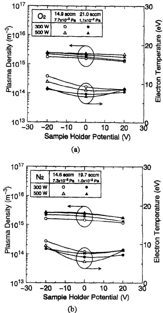
Fig.4 Plasma density and electron temperature vs sample holder potential characteristics for oxygen and nitrogen gases. (a) Oxygen gas. (b) Nitrogen gas.
