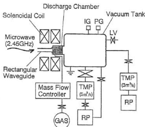
Fig.1 Schematic diagram of space plasma simulator with electron cyclotron resonance plasma accelerator.
