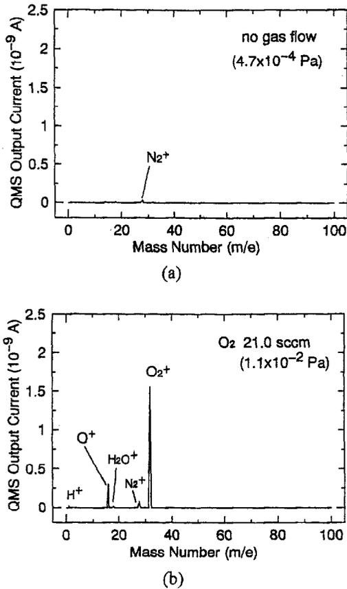
Fig.3 Typical mass spectra in space plasma simulator evacuated by 5-m<sup>3</sup>/s turbo-molecular pump. (a) Mass spectrum for no gas flow at ambient gas pressure of  $4.7 \times 10^{-4}$  Pa. (b) Mass spectrum for oxygen gas flow with flow rate of 21.0 sccm at  $1.1 \times 10^{-2}$  Pa.
