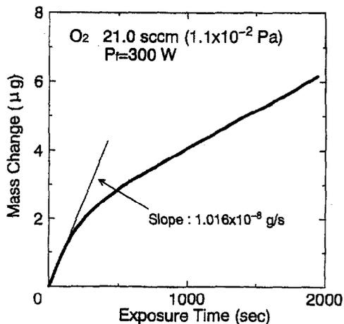
Fig.9 Typical dependence of exposure time on mass change of silver-coated sensor for quartz-crystal microbalance.
