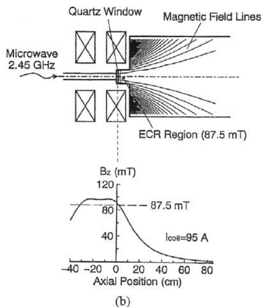
Fig.2 Cross section of electron cyclotron resonance plasma accelerator and calculated magnetic field lines and strength generated by solenoidal coils. (a) Cross section of electron cyclotron resonance plasma accelerator. (b) Calculated applied magnetic field lines and its strength on center axis.
