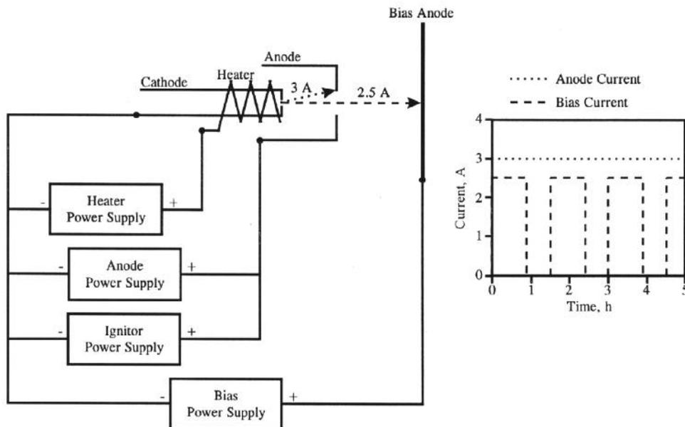
Fig. 2 Schematic of the HCA-bias anode arrangement and current profiles.
