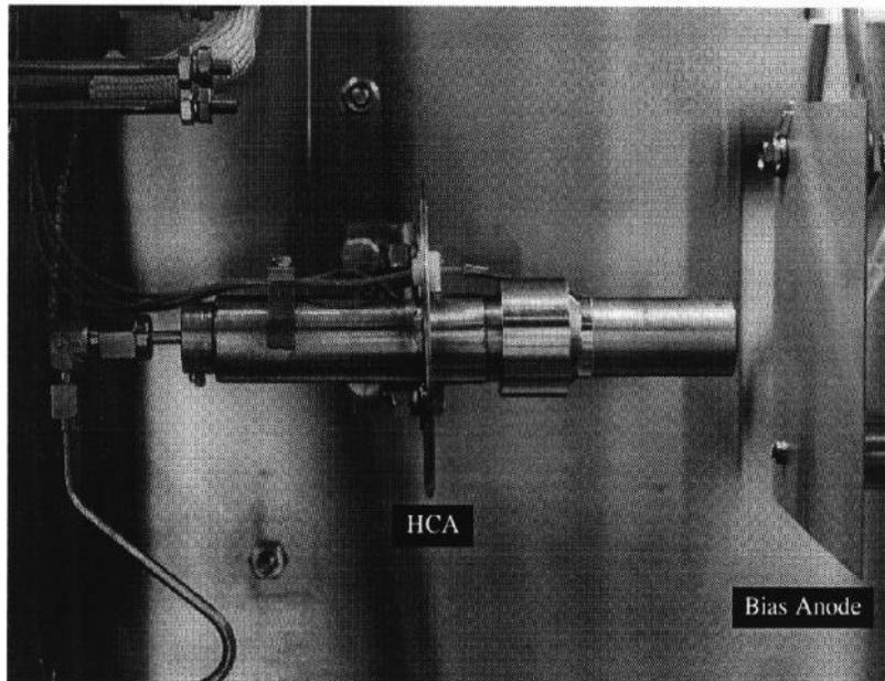
Fig. 1 Photograph of an HCA-bias anode arrangement.
