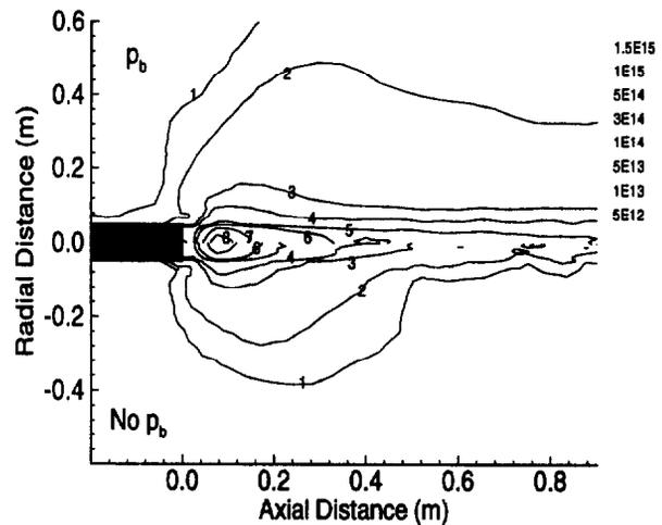
Figure 3: Contours of CEX Ions for constant velocity case with and without back pressure.
