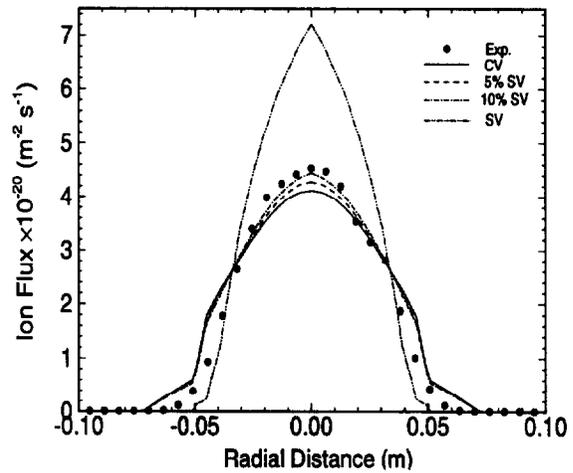
Figure 7: Comparisons of ion flux from various test cases to experiment at 5 cm from the exit.
