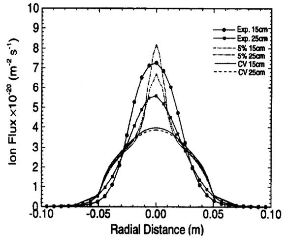
Figure 6: Comparisons of ion flux from various test cases to experiment at 15 cm and 25 cm from the exit.
