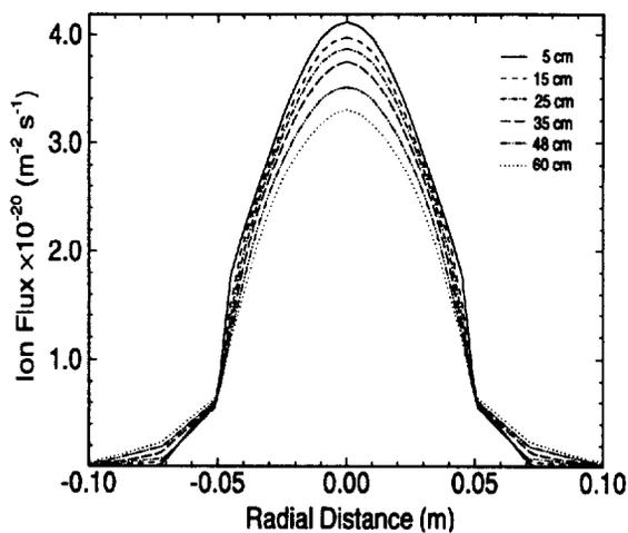
Figure 1: Radial profiles of ion flux at various axial locations for  $T_e = 1eV$ .
