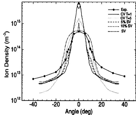
Figure 11: Comparisons of ion density to experimental measurements taken at various angles 122 cm from the center of the exit.
