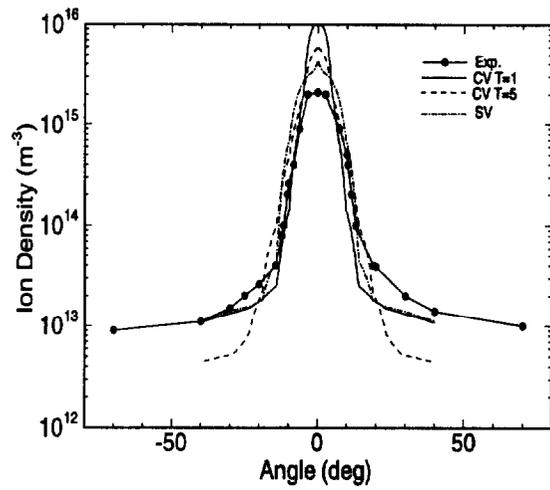
Figure 10: Comparisons of ion density to experimental measurements taken at various angles 61 cm from the center of the exit.
