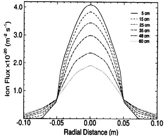
Figure 2: Radial profiles of ion flux at various axial locations for  $T_e = 5eV$ .
