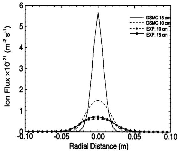
Figure 5: Comparisons of spherical test case with ion flux from experiment.
