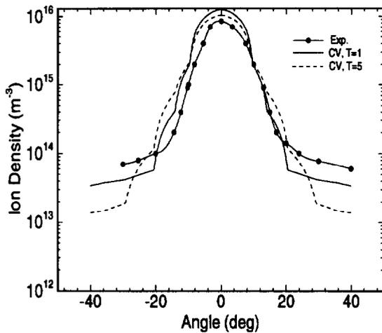
Figure 9: Comparisons of ion density to experimental measurements by Pollard taken at various angles 30 cm from the center of the exit.
