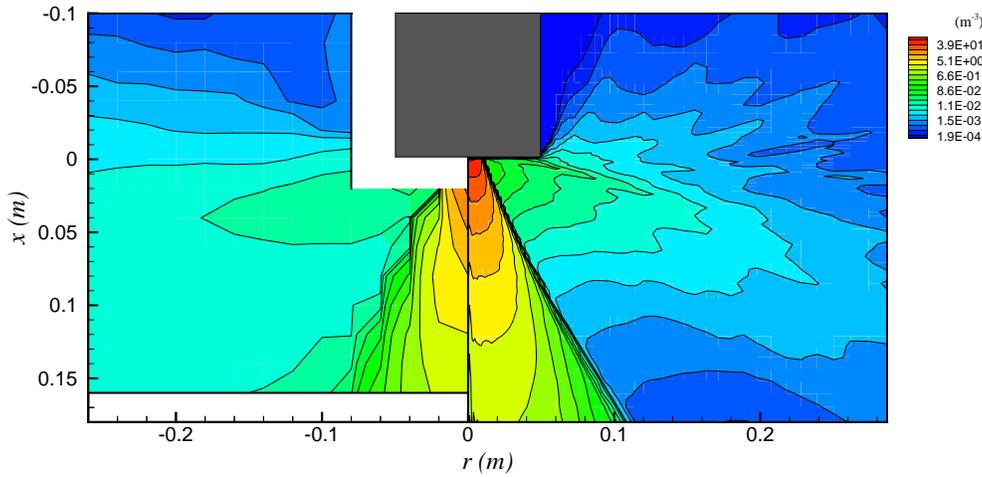
Figure 17. Contours of ion flux (left: experiment, right: simulation).
