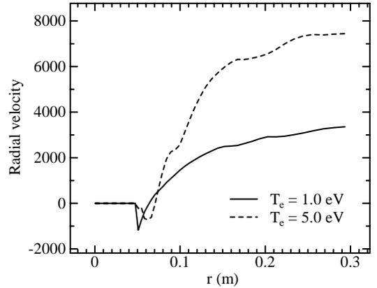
Figure 15. Radial velocity component of CEX ion at 0.08 m behind the thruster exit.
