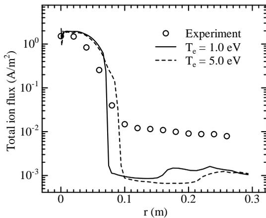
Figure 20. Comparisons of radial ion flux at 0.16 m downstream of the thruster exit.
