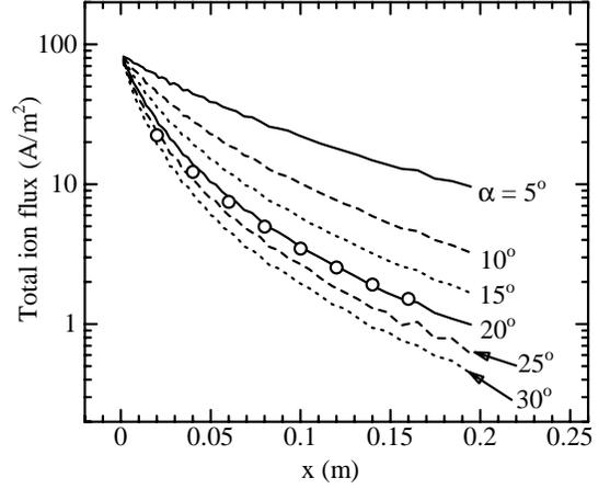
Figure 5. Comparisons of Xe ion flux on the axis.
