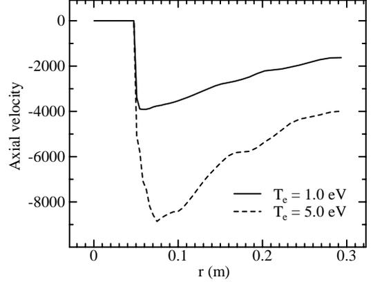
Figure 14. Axial velocity component of CEX ion at 0.08 m behind the thruster exit.
