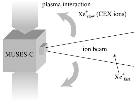
Figure 1. Plasma interaction of ion thruster plume.
