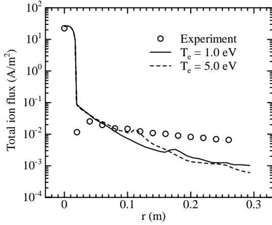
Figure 18. Comparisons of radial ion flux at 0.02 m downstream of the thruster exit.
