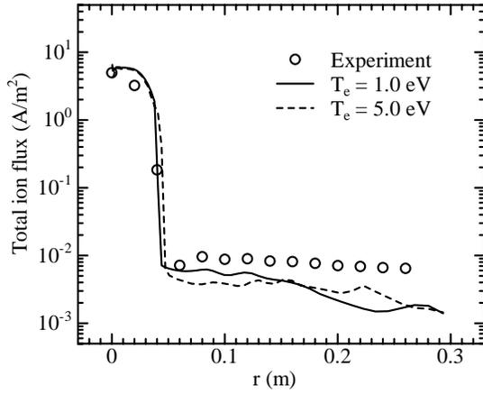
Figure 19. Comparisons of radial ion flux at 0.1 m downstream of the thruster exit.
