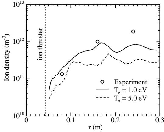
Figure 12. Comparisons of radial ion density at 0.08 m behind the thruster exit.
