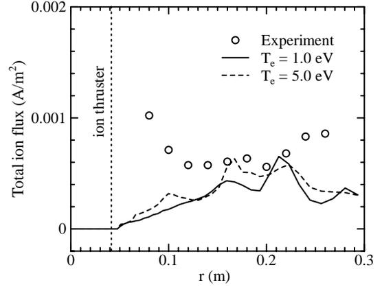
Figure 21. Comparisons of radial ion flux at 0.08 m behind the thruster exit.
