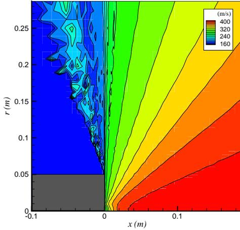
Figure 4. Velocity contours of Xe neutral atoms.
