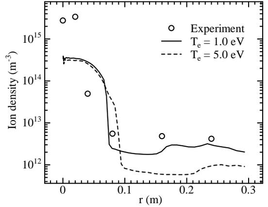
Figure 11. Comparisons of radial ion density at 0.16 m downstream of the thruster exit.
