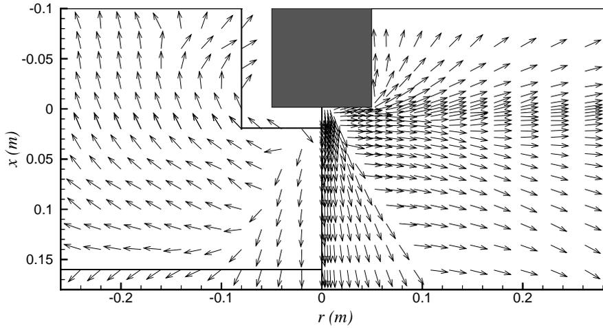
Figure 16. Velocity directions of ion (left: experiment, right: simulation).
