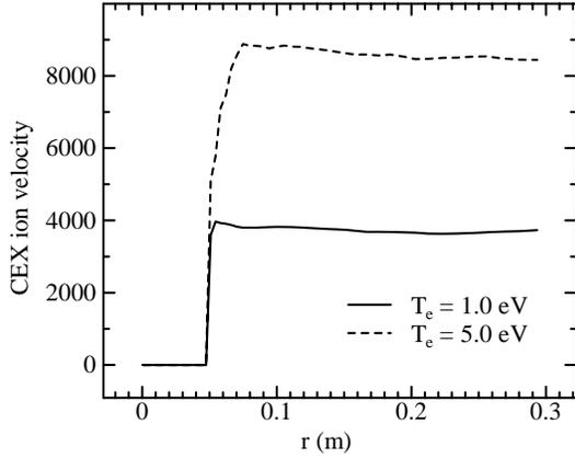
Figure 13. CEX ion velocity at 0.08 m behind the thruster exit.
