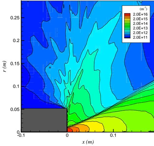
Figure 8. Ion density contours for  $T_e = 5.0$  eV.
