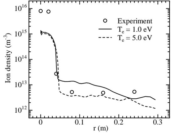
Figure 10. Comparisons of radial ion density at 0.1 m downstream of the thruster exit.
