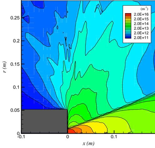
Figure 7. Ion density contours for  $T_e = 1.0$  eV.
