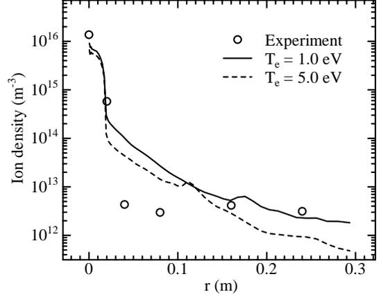
Figure 9. Comparisons of radial ion density at 0.02 m downstream of the thruster exit.
