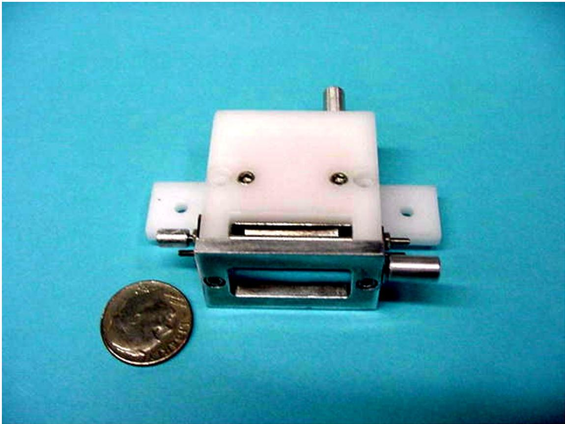
Fig.6 Assembled linear slit colloid microthruster
