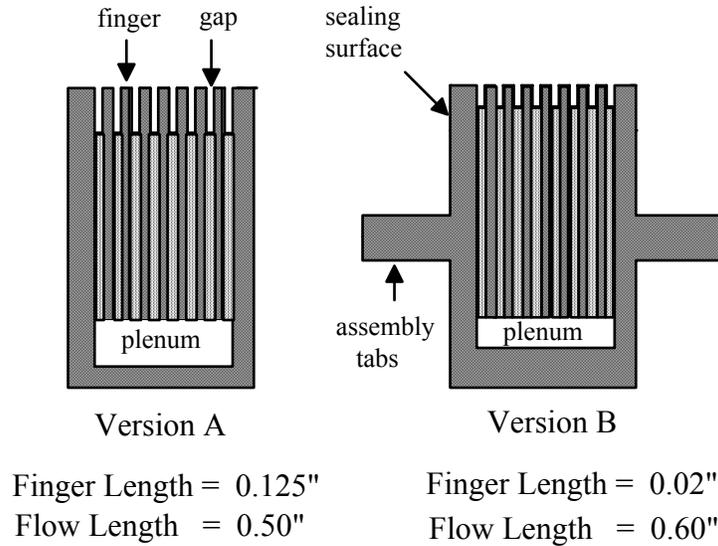
Fig. 5. Photochemically etched rake configurations.
