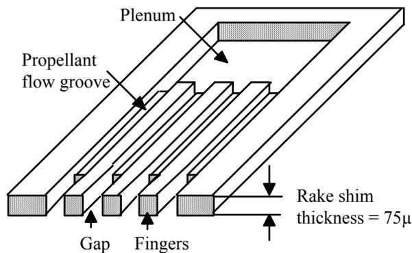
Fig. 3. Photochemically etched rake (shim) concept.
