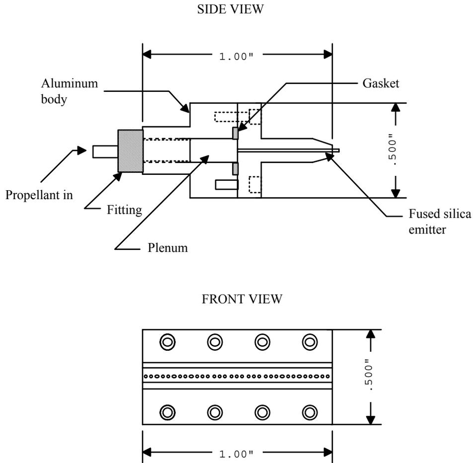
Fig. 12. Fused silica based colloid microthruster design (not to scale).
