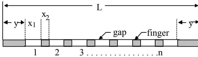
Fig.4 Linear slit rake design elements.
