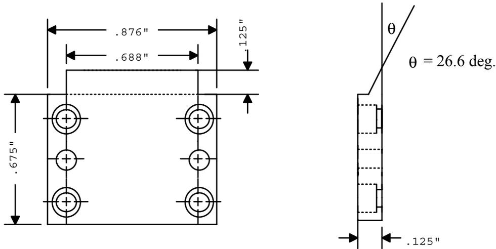
Fig. 2 Linear slit body dimensions (shown on 2:1 scale).
