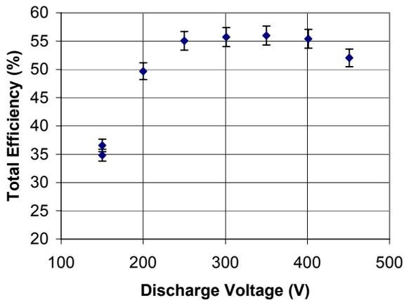
**Figure 8:** Total Efficiency vs Voltage at 2.25 kW
