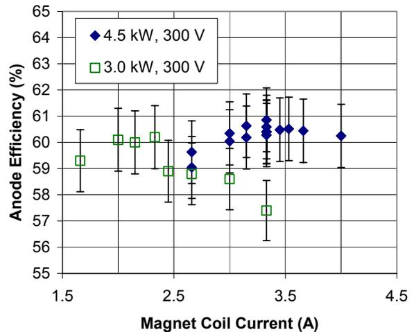
**Figure 10:** Anode Efficiency vs Magnet Coil Current
