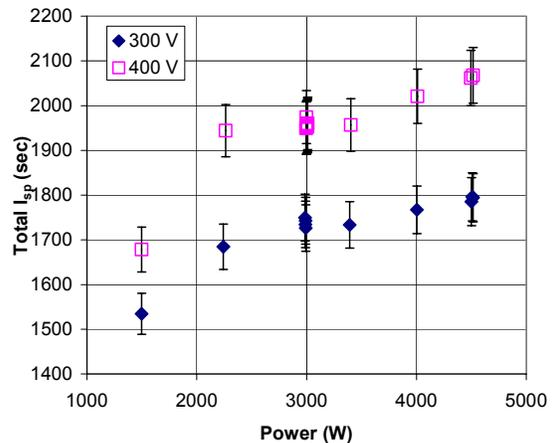
**Figure 7:**  $I_{sp}$  vs Power (300 and 400 V traces)
