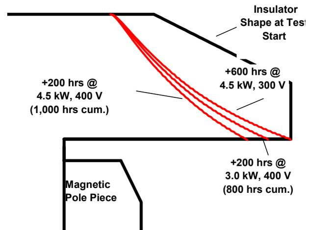
**Figure 12:** Predicted Insulator Erosion Profiles Over 1,000 Hr Life Test
