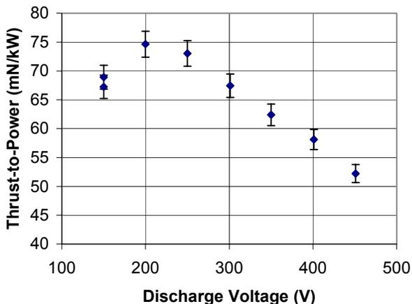
**Figure 9:** Thrust to Power vs Voltage at 2.25 kW
