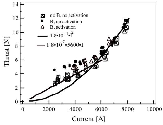
Fig. 17 – Thrust vs Current (660 mg/s, argon).
