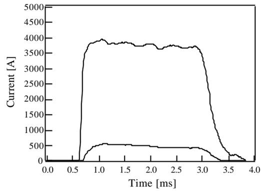
Fig.5 - Current signals (high: primary current, low: ionization chamber current) (Centrosazio).
