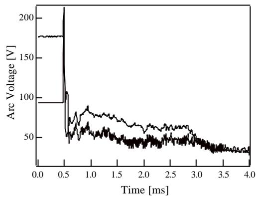
Fig. 6 – Voltage signals (high: primary voltage; low: ionization chamber voltage) (Centrosazio).
