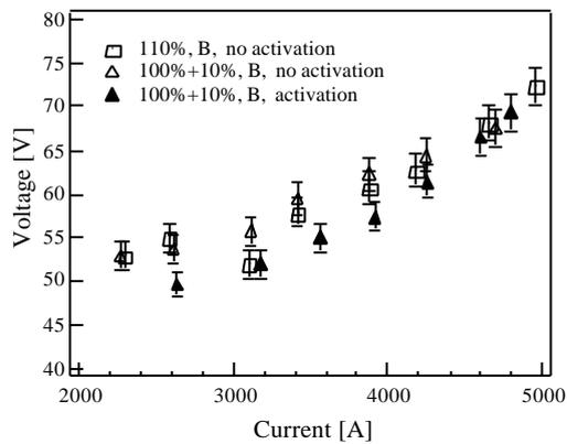
Fig.16 – Electrical Characteristics (660 mg/s, argon, zoom).
