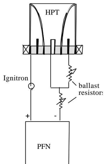
Fig.4 – Main electric circuit arrangement (Centrosazio).
