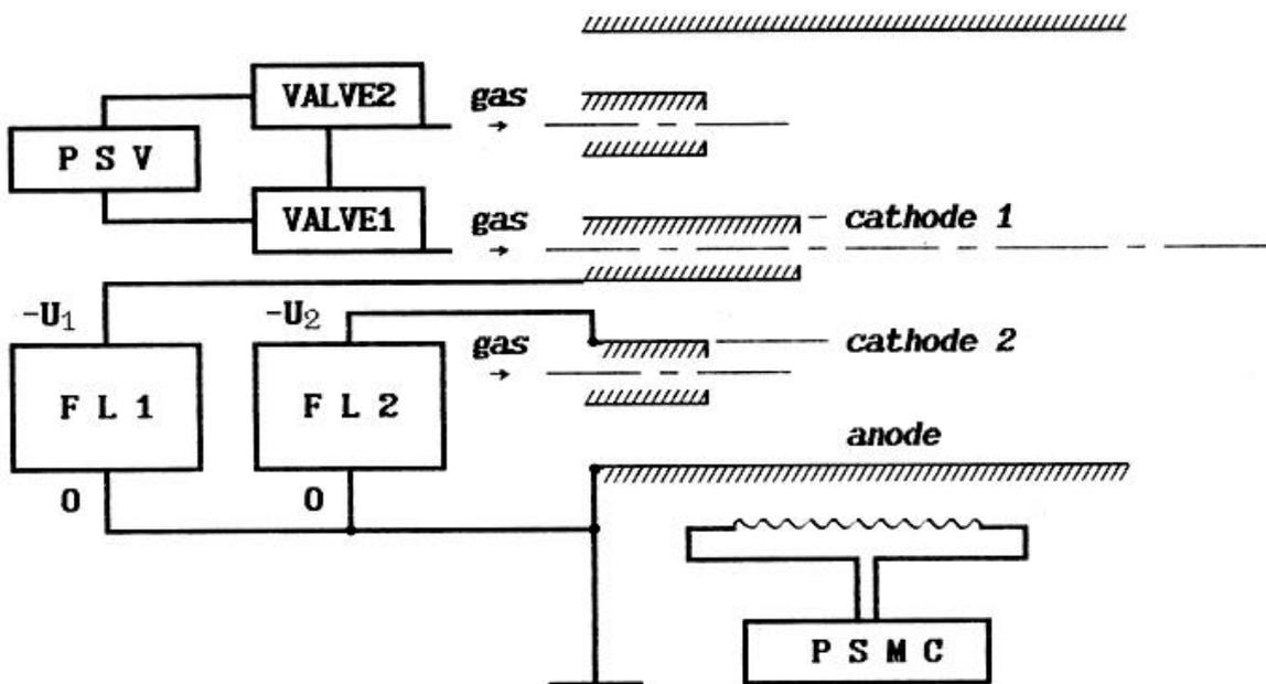
Fig. 2 – Main electric circuit arrangement (RIAME)
