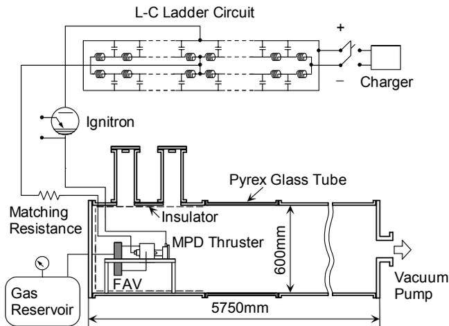
Figure 2 Experimental system with pulse forming network, fast acting valve and MPD thruster.
