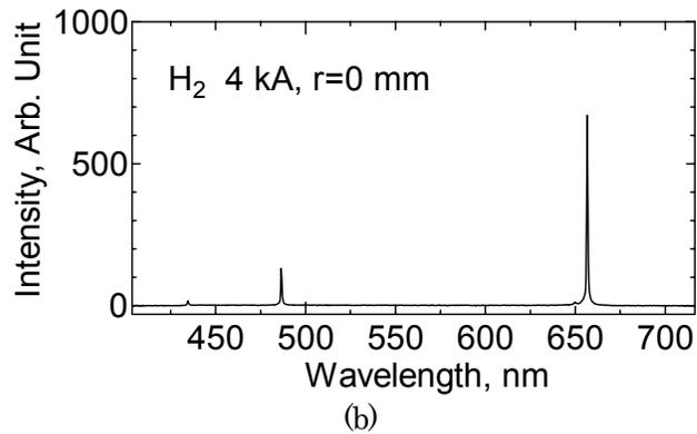
Figure 3 Typical spectra emitted from MPD plasma at nozzle exit. (a) Ar, 1.37 g/s, 4 kA; (b) H<sub>2</sub>, 0.40 g/s, 8 kA.
