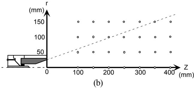
Figure 7 Measurement points for rotatable double probe. (a) near divergent nozzle exit; (b) downstream region.
