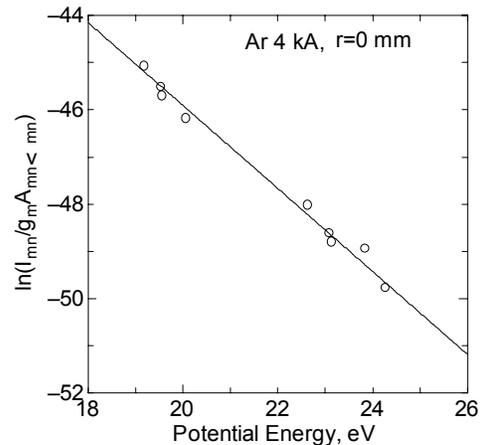
Figure 4 Typical Boltzmann plotting for determination of electronic excitation temperature with ArII lines at Ar, 1.37 g/s and 4 kA.
