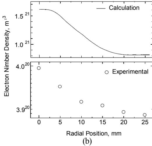
Figure 14 Calculated and experimental results of radial distributions of electron temperature and plasma number density on arcjet nozzle exit with Ar and 4 kA. (a) electron temperature; (b) plasma number density.
