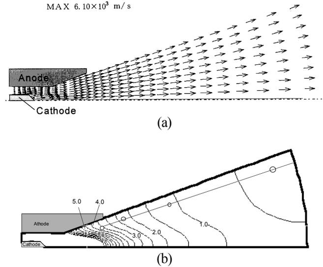
Figure 15 Calculated patterns of plasma velocity vector and ion flux with Ar and at 4 kA. The dashed line represent an equi-ion-flux-line of 90 % on the total flux. (a) plasma velocity vector; (b) ion flux.
