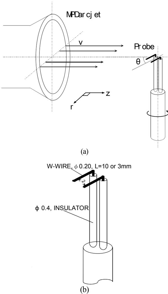
Figure 5 Rotatable electrostatic double probe system for measurement of plasma flow direction, electron temperature and plasma number density. (a) probe and plasma flow arrangement; (b) probe structure.
