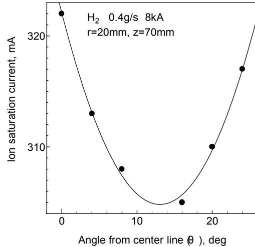
Figure 6 Typical characteristics of ion saturation current of rotatable double probe dependent on angle of probe line to plasma flow.
