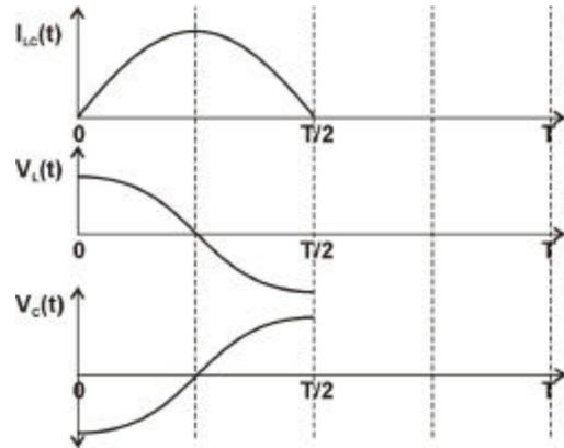
Figure 6: Waveforms of LC resonant circuit.
