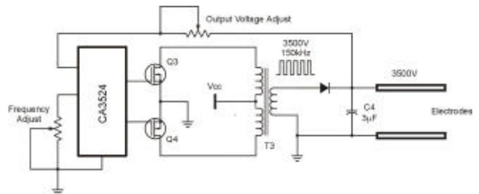
Figure 3. High voltage power supply scheme.
