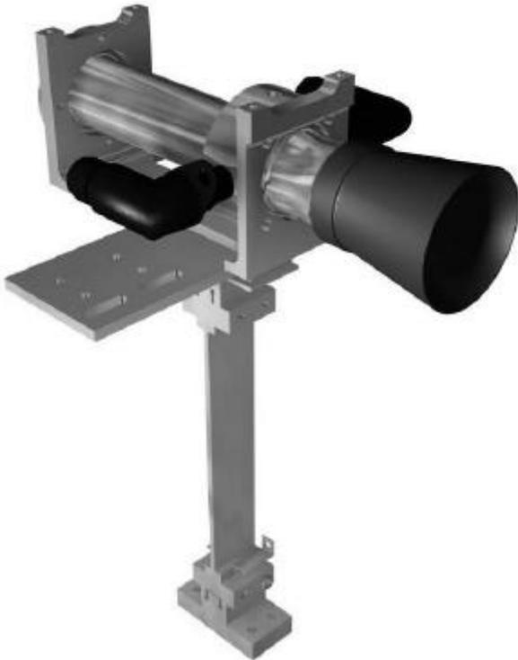
Figure 2. APPT on the test stand
