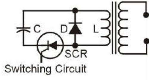
Figure 5: Proposed LC resonant circuit.
