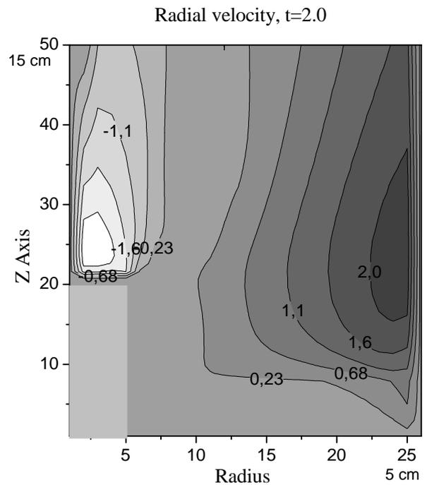
Figure 8. Radial velocity distribution in APPT accelerating channel ( $t= 4 \mu s$ ).
