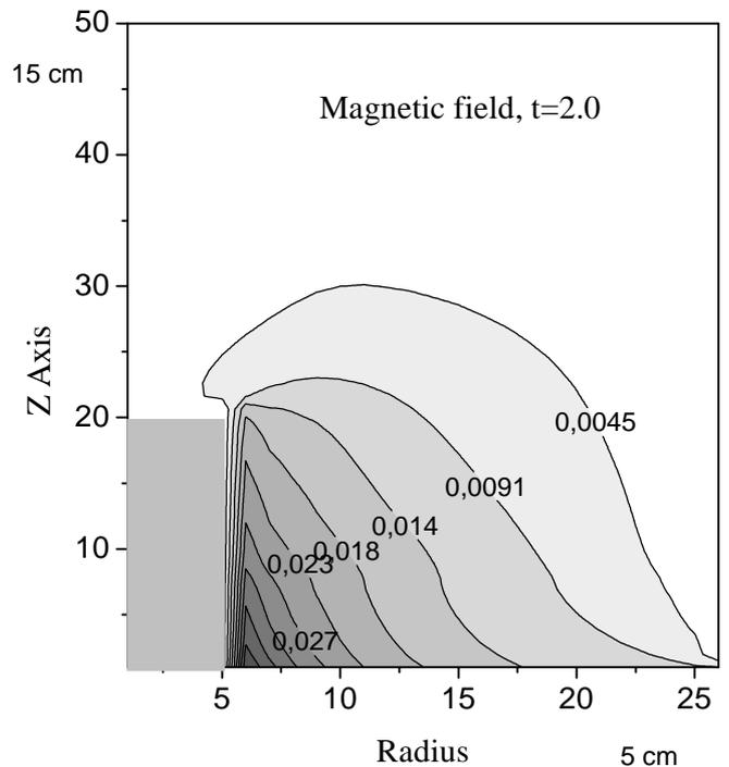
Figure 5. Magnetic field distribution in APPT accelerating channel ( $t= 4 \mu\text{s}$ ).
