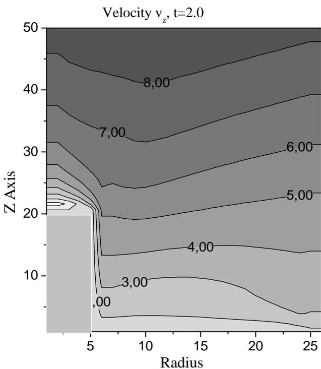
Figure 7. Axial velocity distribution in APPT accelerating channel ( $t= 4 \mu s$ ).
