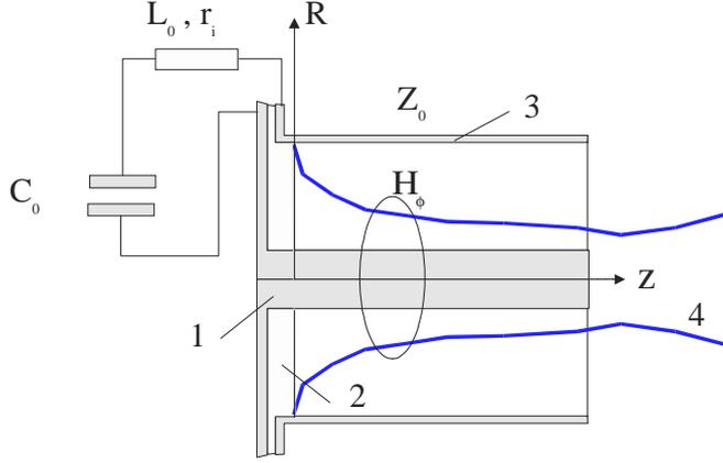
Figure 1. APPT and the electric circuit diagram; 1- internal electrode, 2 – solid propellant, 3 - external electrode, 4 -plasma.
