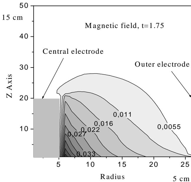
Figure 3. Magnetic field distribution in APPT accelerating channel ( $t= 3.5 \mu\text{s}$ ).
