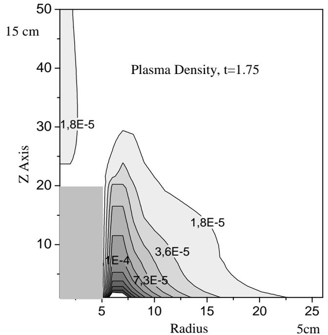
Figure 4. Plasma density distribution in APPT accelerating channel ( $t= 3.5 \mu\text{s}$ ).
