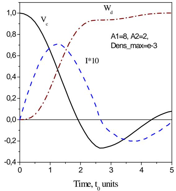
Figure 2. Time dependencies of a current and bank voltage in APPT;  $t_0= 2 \mu$ s.
