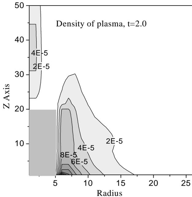
Figure 6. Plasma density distribution in APPT accelerating channel ( $t= 4 \mu s$ ).
