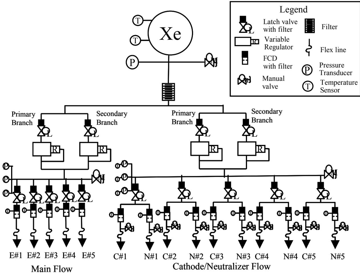
*Fig. 8 Xenon feed system for the TEMPO ion propulsion system.*
