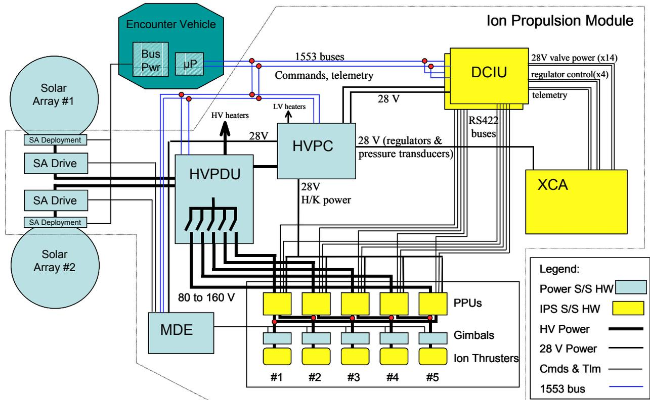
**Fig. 9** Simplified block diagram of the power and data system for the TEMPO IPM.
