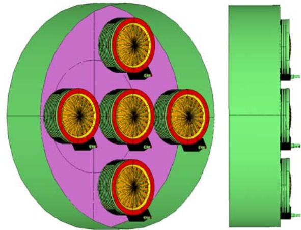
**Fig. 7 Ion engine thermal model configuration showing engines partially buried in the launch vehicle adapter.**
