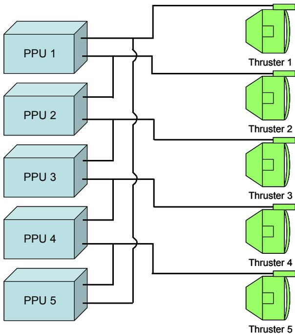
**Fig. 6 PPU to engine cross strapping.**
