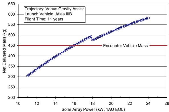
**Fig. 4** Increasing solar array power increases the net delivered mass capability at a fixed flight time. The net delivered mass is everything that is not the ion propulsion system or solar array.
