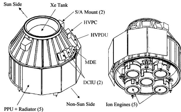
**Fig. 5** Ion Propulsion Module (IPM) Configuration (without the solar arrays).
