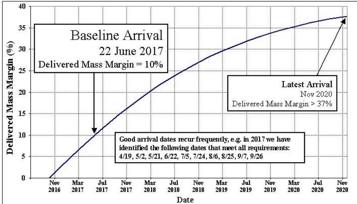
*Fig. 2 Delivered Mass Margin increases rapidly with flight time*
