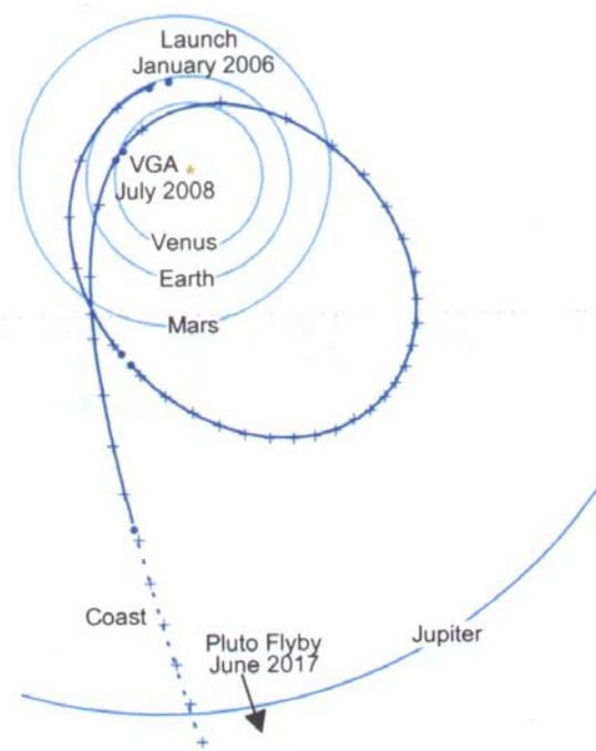
*Fig. 3 Venus gravity assist trajectory for an ion propulsion mission to Pluto.*
