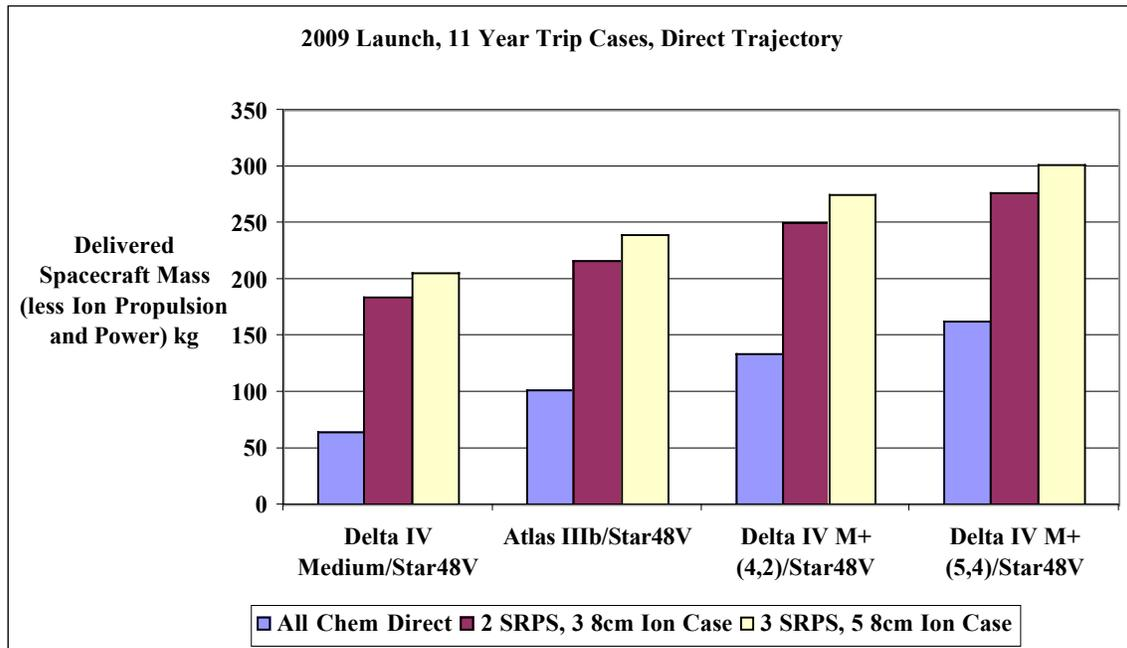
**Figure 6. Pluto Flyby Net Mass vs Launcher**
