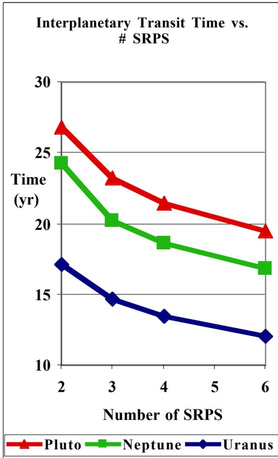
**Figure 10. Interplanetary Transit Time vs. Number of SRPS**
