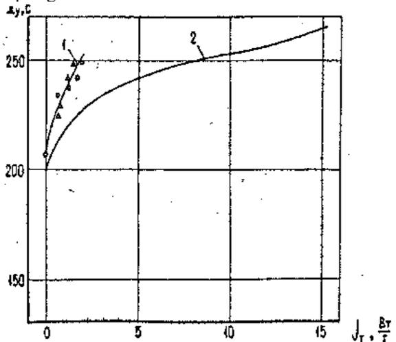
Rice 6 Dependence of a specific impulse of thrust  $I_{sp}$  from the price of thrust  $J_t$  of thrusters 1 - K10PG N05 and N11 and 2 - TK10/3000.
