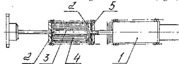
Pic 4. Drawing of a thruster of modification 3. 1 - the chamber of the thruster, 2 - a grid, 3 - a core, 4 - needles made from a wire, 5 - fibrous heat insulation linings
