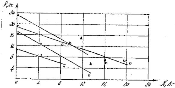
Pic 2 Dependence of thrust of K10PG thruster from input power.  $\blacktriangle$  -  $P_{in}=6$  kgf/cm<sup>2</sup>,  $\blacksquare$  -  $P_{in}=7$  kgf/cm<sup>2</sup>,  $\bullet$  -  $P_{in}=4$  kgf/cm<sup>2</sup>,  $\blacklozenge$  -  $P_{in}=3$  kgf/cm<sup>2</sup>
