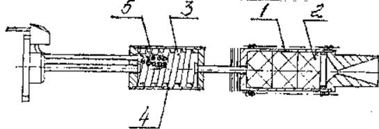
Pic 1 Drawing of a thruster of modification 1. 1 - the thruster chamber, 2 - the metal catalyst, 3 - auger, 4 - the case of a steam generator, 5 - heater.
