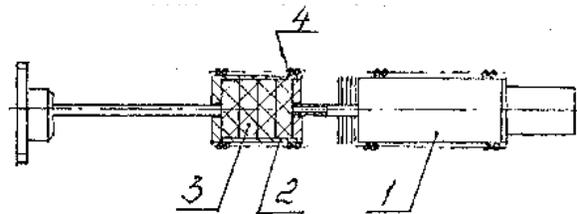
Pic 3. Drawing of a thruster of modification 2. 1 - the chamber of the thruster, 2 - the vapor-generator body, 3 - wire briquettes, 4 - heater.
