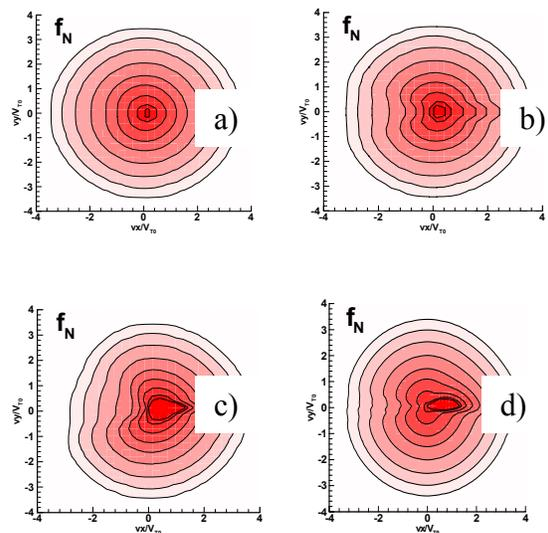
Figure 15 – Gas distribution function at 3 locations in Fig.12: a) – inside q.tube, b) – at the open end of q.tube, c) –  $(L_X, L_Y/2)$ , and d) – at the marked position in Fig. 14
