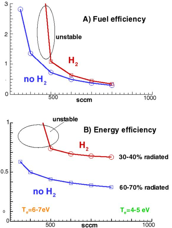
Figure 27 – Mass scans of “fuel” (A) and energy (B) efficiencies for with (no H<sub>2</sub>) and without (H<sub>2</sub>) catalytic brake of molecules
