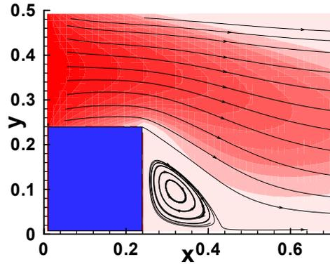
Figure 8 - Back step flow structure
