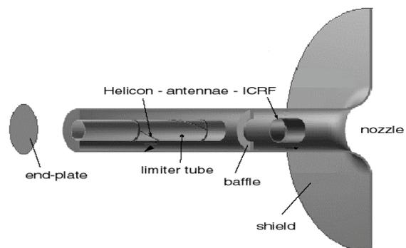
Figure 1 – Gas/plasma facing section of VASIMR thruster
