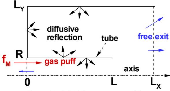
Figure 7 – Model geometry used in a rarified gas flow simulation
