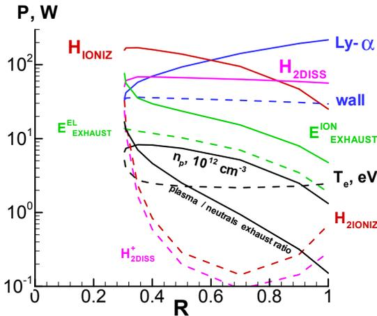
Figure 29 – Helicon hydrogen discharge parameters vs fraction, R, lost due to Ly- $\alpha$  radiation. 1-R part is re-captured by plasma
