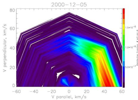
Figure 31 – IDF as measured by RPAs in the VX-10 VASIMR configuration
