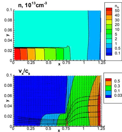
In Fig.15 a) and b) we present contours of the gas distribution function right at the symmetry plane inside (1/2 length) the quartz tube (a) and just outside it (Figure 12 - Results for 100sccm flow rate inside, but starts to deviate from the equilibrium outside the pipe. It is even more non-Maxwellian at half-height of the system, as shown in the Fig.15c. Such strong deviation of the core of the gas distribution function
