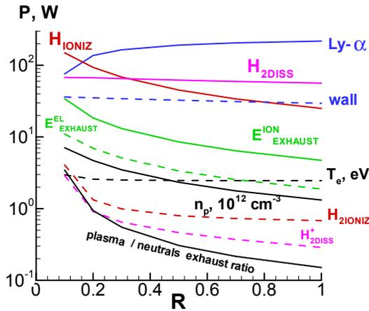
Figure 28 – Helicon hydrogen discharge parameters vs fraction, R, lost due to Ly- $\alpha$  radiation (electron impact excitation).
