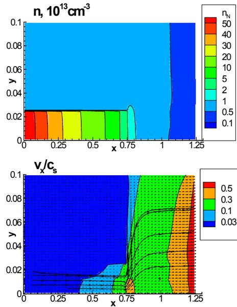
The numerical result for a baffle, blocking 70% of the gas flow are shown in Fig.13. They have to be compared with the results for a conical-shaped tube. As we can see, gas density outside the tube dropped twice. Note that the radial baffle is located at the very end of the quartz tube. (We think that conical-shaped tube works as an extended baffle, but may bring other benefits).
