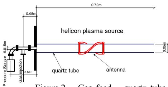
Figure 2 – Gas feed – quartz tube of VX-10 VASIMR configuration
