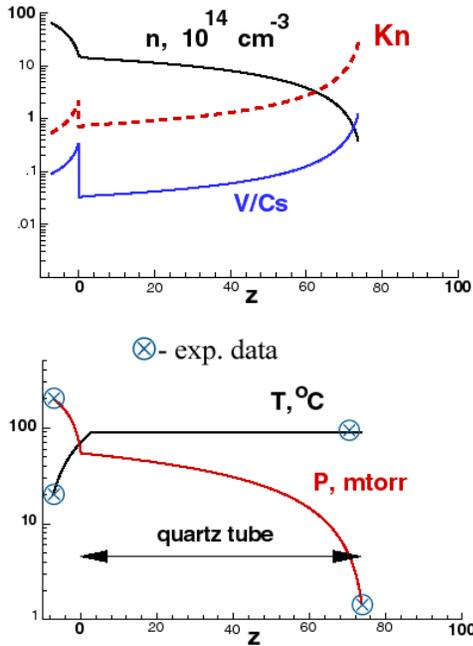
Figure 4 – Profiles of helium gas flow parameters for the VX-10
