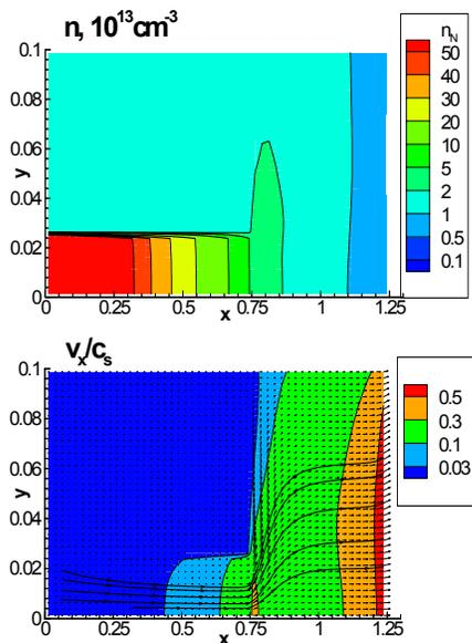
The simulation results for a 50 sccm H flow rate are shown in Figs.11. As one can see these results are in agreement with the 1D semi-analytical model, considered above. Indeed, gas accelerates to  $M \sim 1$  at the both boundaries. Also these results verify the need for gas pumping from the outside of the quartz tube. Otherwise, the discharge will occur here due to relatively high residual gas pressure around the helicon antenna, that can cause its damage.
