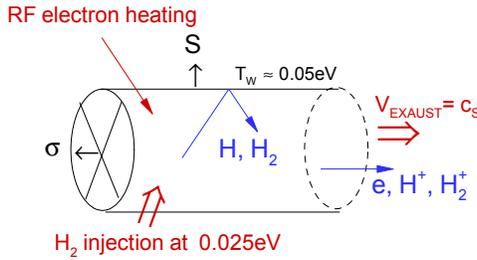
Let's accept the following physical model of a helicon plasma source, as shown in Fig.16. Next, we consider the ac Fig.16. Helicon discharge model taking
