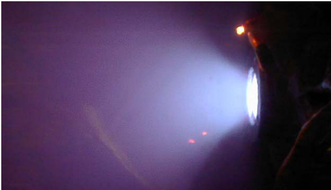
Fig.3 Operation of Microwave Engine in Vacuum Chamber
