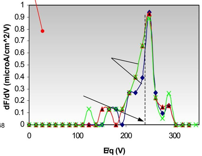
Figure 8. Computed value of the main beam ion energy and measured energy spectra onboard the Express A#3 spacecraft. RPA values obtained during firings of the T4 SPT100 on 6/7/2000.
