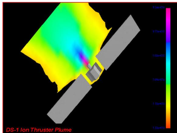
Figure 13. Ion particle density (in  $m^{-3}$ ) from a 30-cm ion thruster. The spacecraft is the EWB-generated model of DS-1.
