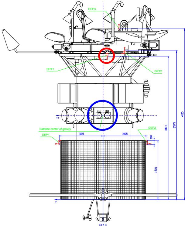
Figure 3. Side view of the Express A#2 spacecraft. Circled are the ion flux sensor (small circle) and SPT100 unit (large circle).
