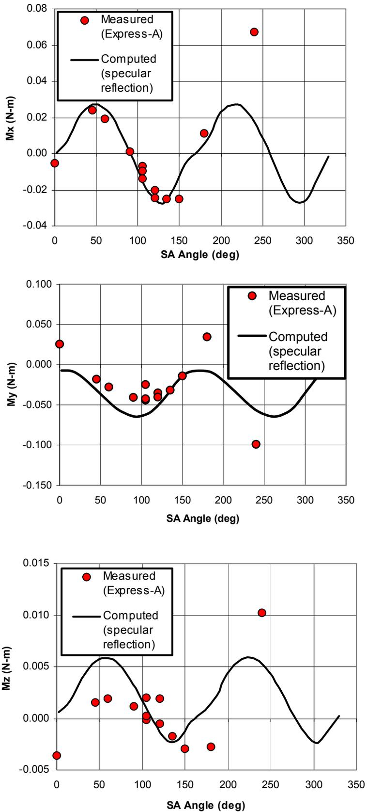
Figure 14. Comparison between computed and measured torques induced by firings of the RT4 SPT100 onboard the Express-A spacecraft. The data was acquired during a rotation of the solar array.
