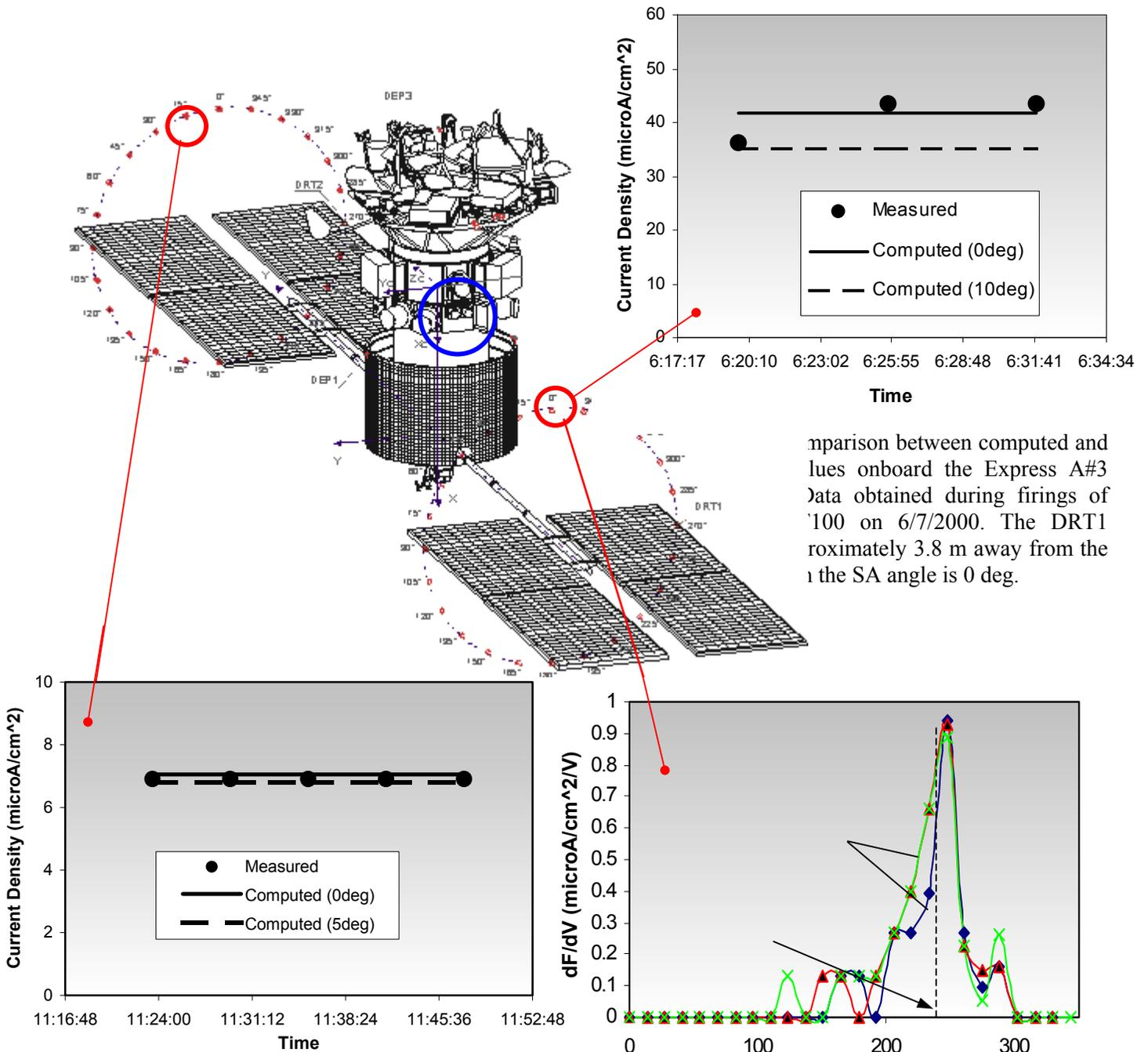
Comparison between computed and measured values onboard the Express A#3 spacecraft. Data obtained during firings of the RT3 SPT100 on 6/7/2000. The DRT1 sensor is approximately 3.8 m away from the thruster when the SA angle is 0 deg.
