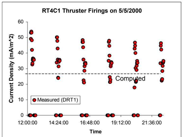
Figure 4. Comparison between computed and measured current densities as registered onboard the Russian Express A#2 spacecraft.
