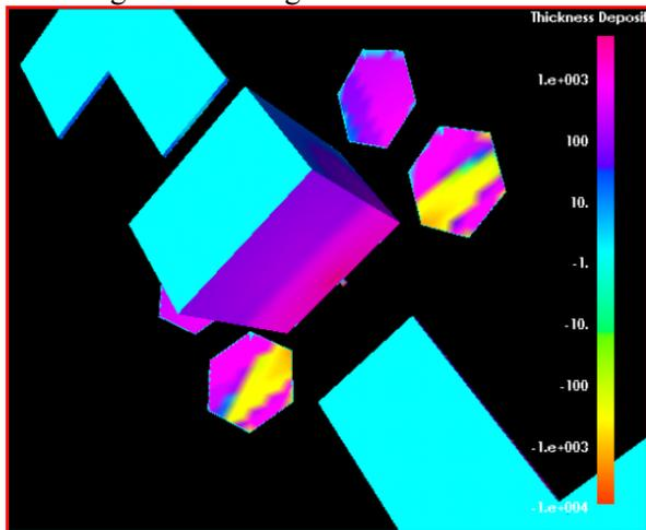
Figure 10. Sputtered erosion depth and redeposition thickness on typical satellite.
