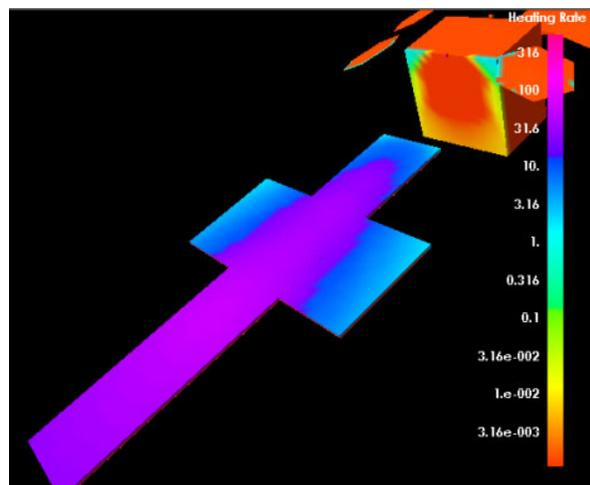
Figure 11. Surface heating due to thruster plume impingement and ionization.
