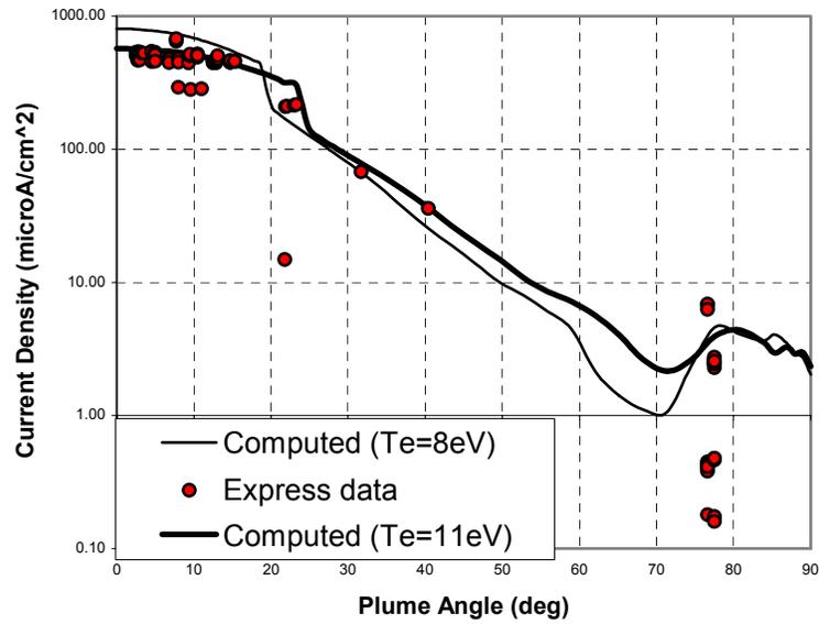
Figure 9. Comparison between current density measurements on board the Express-A spacecraft and computed values using the 2-D plume code at a radius of 1 m. Measurements taken at different locations were scaled down to 1-m using a  $1/r^2$  scaling.
