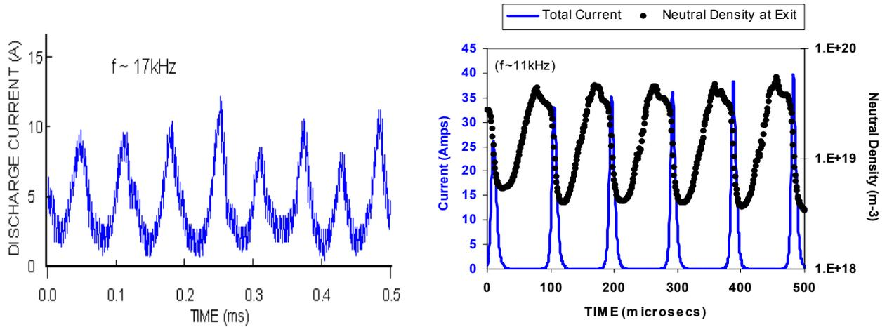
Figure 1. Left: Measured evolution of the discharge current for the SPT-100 (data taken during tests at NASA/GRC). Right: Computed evolution of the discharge current and neutral density (at exit) using the 1-D, Hall thruster computer model.
