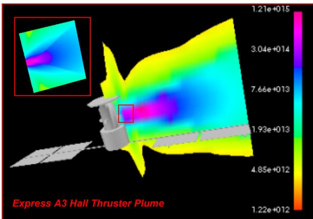
Figure 12. Ion particle density (in  $m^{-3}$ ) from an SPT100. The spacecraft is the EWB-generated model of the Express satellite.
