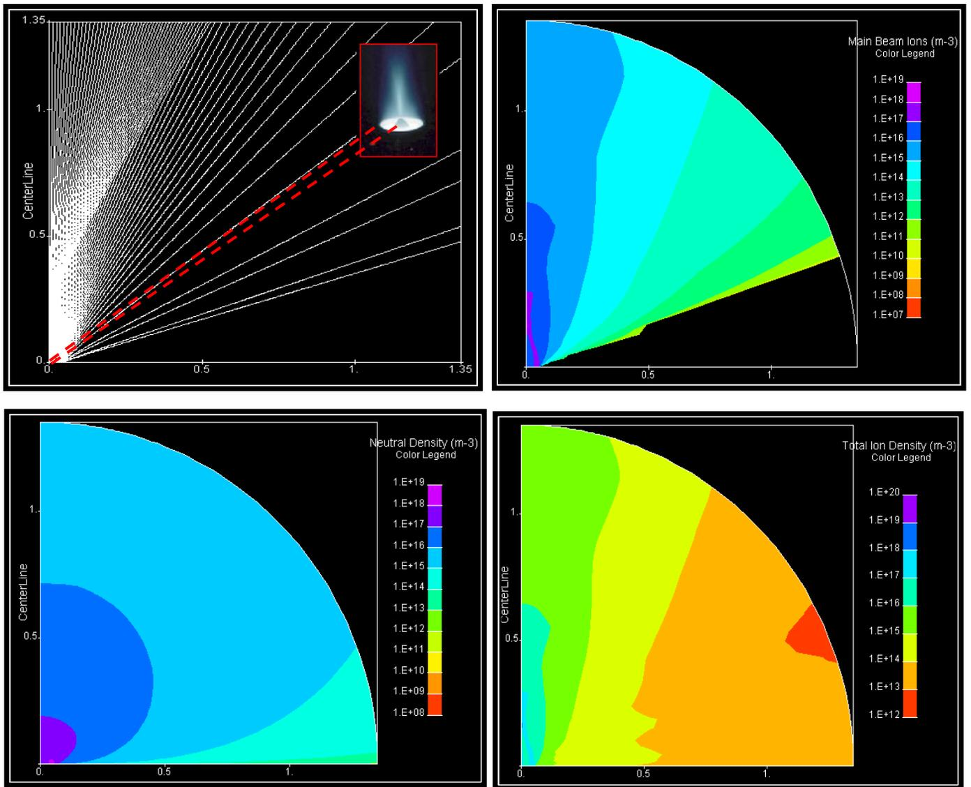
Figure 2. Results of 2-D plume simulation of SPT100 showing ion trajectories (top left), main-beam ion density (top right), neutral density (bottom left) and total ion density (bottom right).
