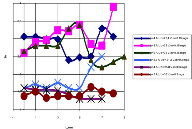
Fig. 10 Distribution of temperature electron components of plasma
