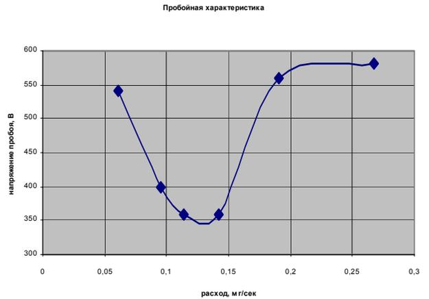
Fig. 9 Breakdown characteristic M1.07 cathode specification
