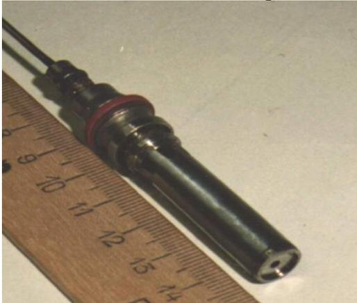
Fig. 7 Photo of the cathode M1.07
