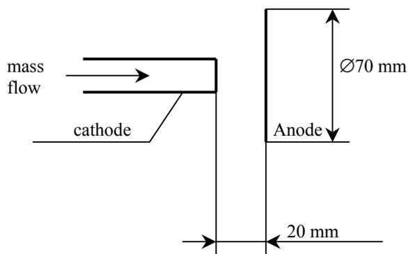
Fig. 2 The scheme of measurement of current-voltage characteristic.
