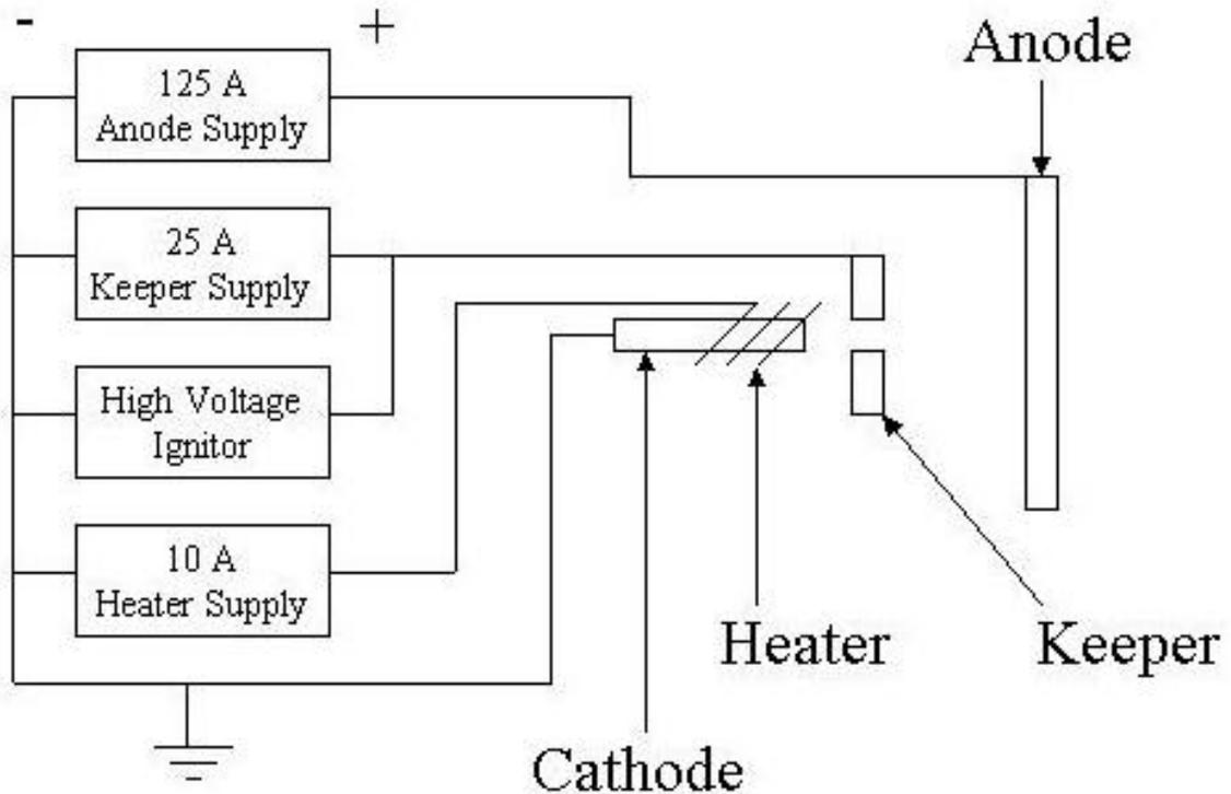
Figure 3 – Electrical wiring diagram of test setup.
