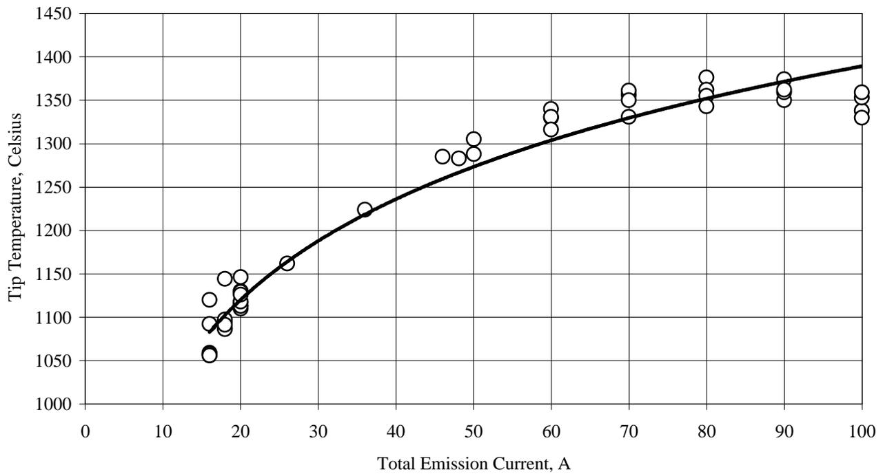
Figure 7 – Cathode tip temperature (Thermocouple 6) as a function of total emission current at 2.0 mg/s.
