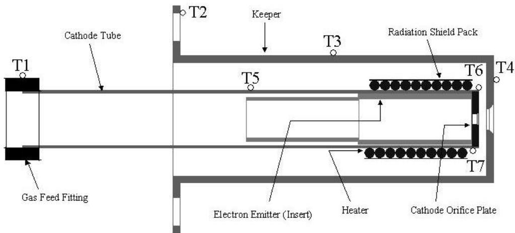
Figure 2 – Thermocouple placement (Drawing not to scale).
