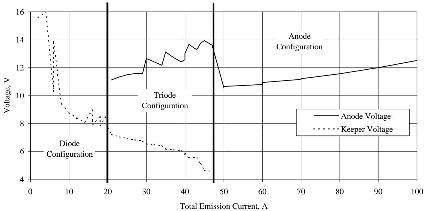
Figure 4 – Voltage as a function of current at 2.0 mg/s xenon flow rate.
