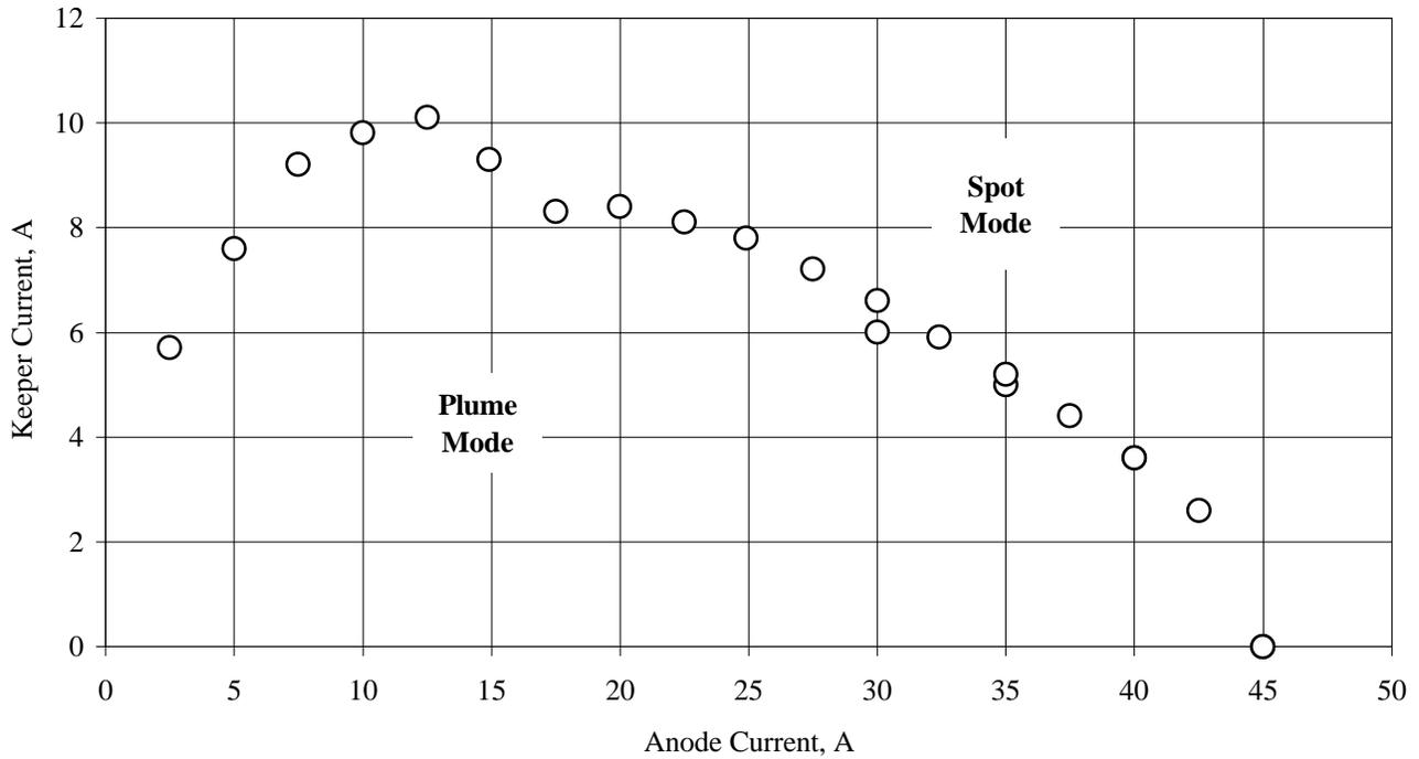
Figure 5 – Keeper current as a function of anode current showing conditions required to maintain spot mode at 2.0 mg/s.
