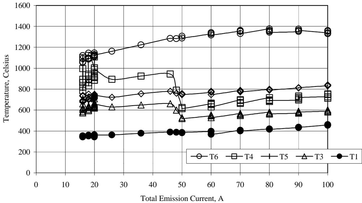
Figure 6 – Temperature as a function of total emission current in triode and anode configurations at 2.0 mg/s.
