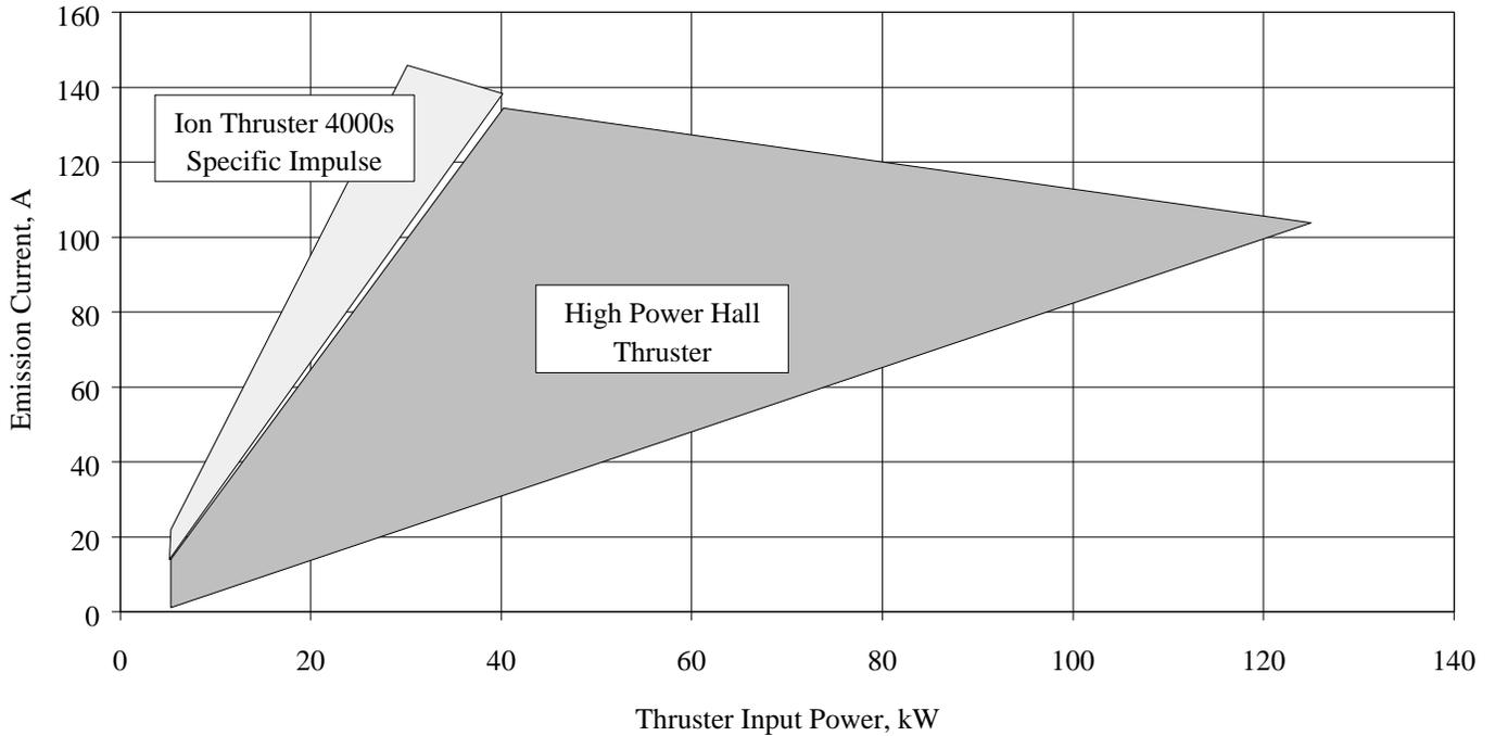
Figure 1 – Cathode emission current requirements as a function of input power for various thrusters using xenon propellant. The line-shaded region corresponds to emission currents required for high power Hall thruster operation. The dot-shaded region corresponds to emission currents required for ion thrusters operating at 4000 seconds specific impulse.
