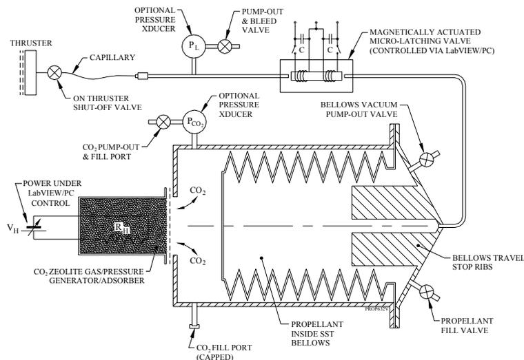
Figure 12 Schematic of the Propellant Storage and Feed System
