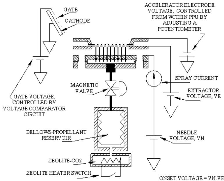
Figure 4 Schematic of the colloid thruster system.
