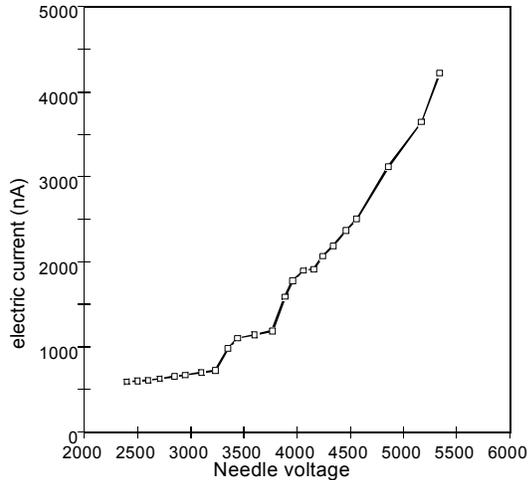
Figure 3 Electric current versus needle voltage for a glycerol solution. Additional cone-jets are generated in the needle rim as the voltage is increased. Formation of a new jet causes a current step and hence a thrust step.
