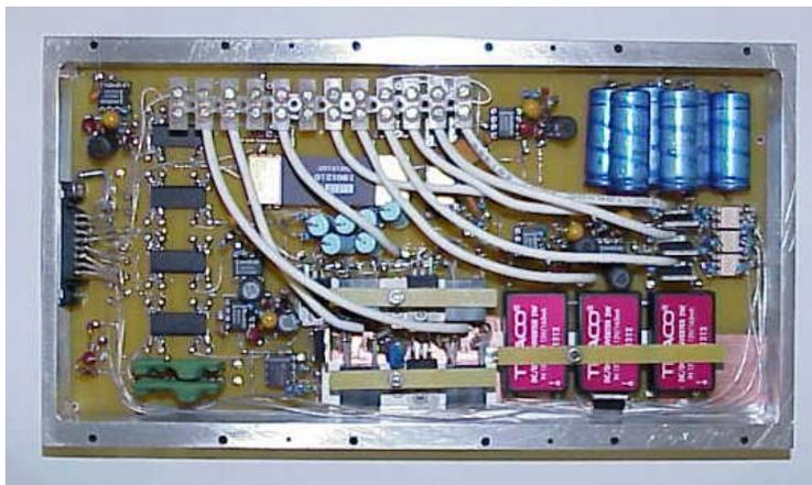
Figure 11 Top view of PPU prototype
