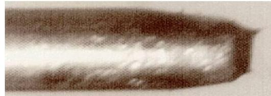
Figure 2c Glycerol in a multi-cone spraying mode. The needle voltage is set at 3600 V. Two off-axis emission points are observed
