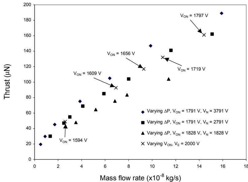
Figure 16 Thrust versus mass flow rate for the electro spray beams of a formamide solution  $K = 0.50$  S/m. The figure presents data for both “pressure controlled  $\dot{m}$ ” (three first series, taken at different acceleration voltages), and “voltage controlled  $\dot{m}$ ” (last data series) strategies
