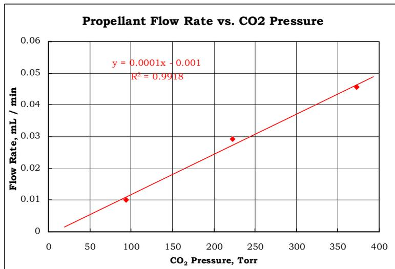
Figure 21 Propellant Flow Rate Versus CO<sub>2</sub> Pressure Measured with our Feed System. The Zero Intercept is at 22 torr which corresponds to the bellows precompression
