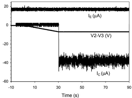
Figure 18 Evolution of the voltage difference between “cathode” and “lab” grounds, and the electro spray and cathode currents as a function time. Continuous electron emission is used to neutralize the electro spray beam
