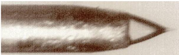
Figure 2a Cone-jet of glycerol. The needle voltage is set at 2600 V. The liquid meniscus ends in one on-axis jet
