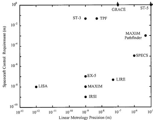
Figure 1 Spacecraft position and metrology requirements for various missions<sup>4</sup>
