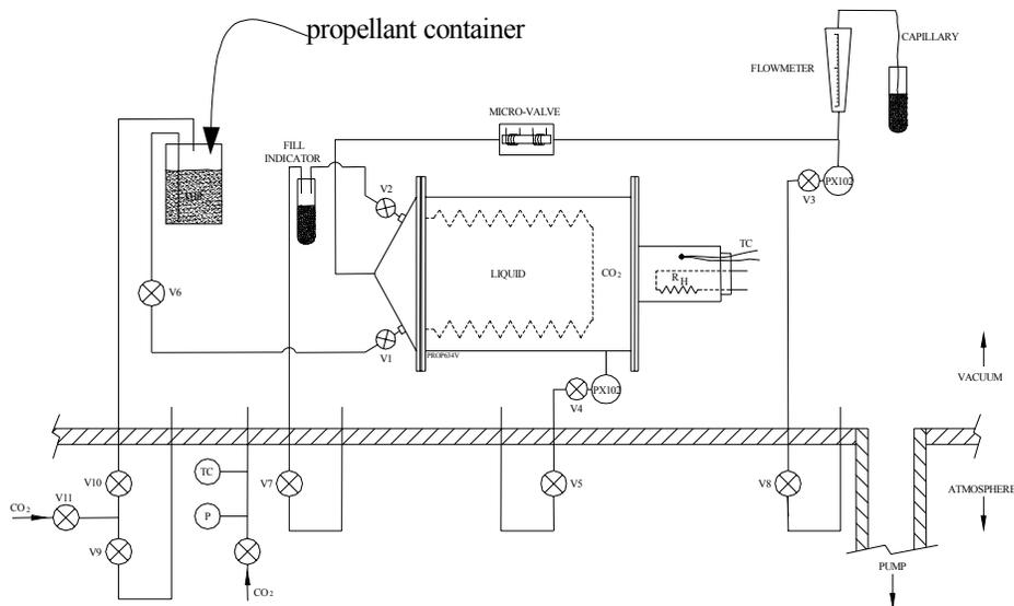
Figure 15 In-vacuum System Fueling Schematic. The Same Set-up with all Shut-off Valves Closed (V1, V2, V3, V4), was Used for Testing of the Feed System.
