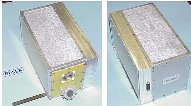
Figure 7 Assembled 20  $\mu$ N thruster system. Electron screen on the top allows rapid pump out. The PPU is inside the solid aluminum frame mounted on the side of the system housing and the thruster with neutralizer are mounted on a dielectric plate. Power and control signals are supplied via the 15 pin D type connector on the back side of the PPU frame
