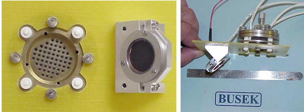
Figure 5 20  $\mu$ N colloid thruster and carbon nanotube (CNT) field emission (FE) neutralizer mounted on a common dielectric base.
