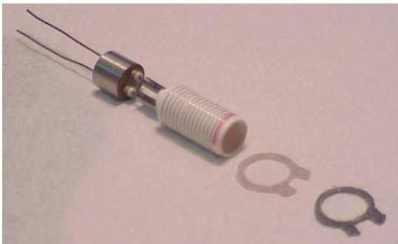
Figure 13 Photograph of the Zeolite Heater Prior to its Installation/Welding into the Zeolite Chamber
