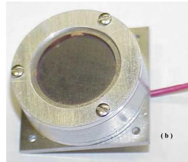
Figure 10 Carbon nanotube field emission neutralizer (a) Components, (b) Assembled neutralizer. The base dimension is approximately 3x3 cm.
