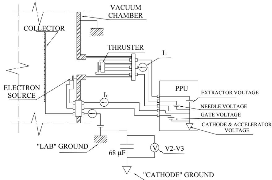
Figure 17 Schematics of the experimental setup used to test the neutralization of the electro spray beam
