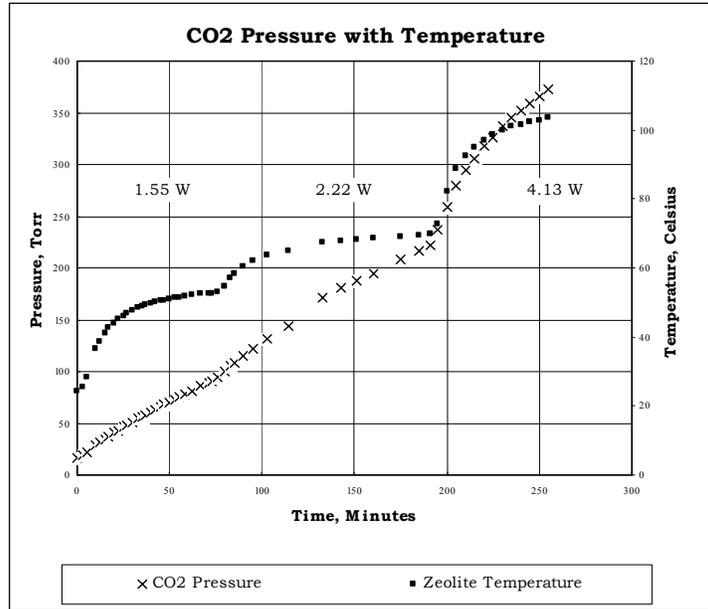
Figure 20 Typical Histogram of Zeolite Temperature and CO<sub>2</sub> Pressure Measured Using our Feed System
