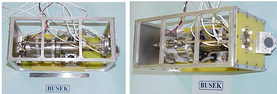
Figure 6 The 20  $\mu$ N colloid thruster system during the thruster, neutralizer and feed system integration
