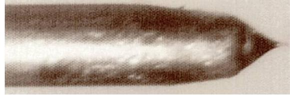
Figure 2b Cone-jet of glycerol. The needle voltage is 3230 V
