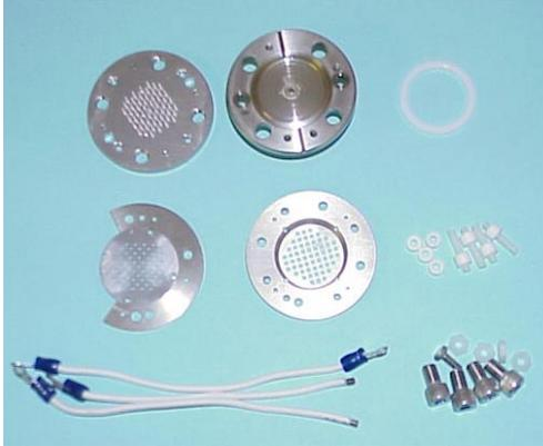
Figure 8 Colloid thruster components conveniently fabricated from standard ConFlat flange.
