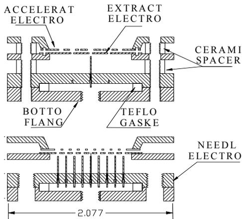
Figure 9 Colloid Thruster Cross-section
