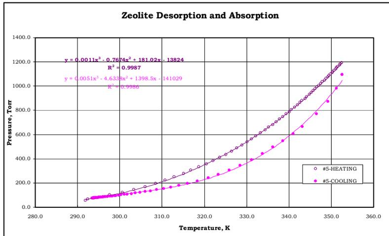
Figure 19 Typical Desorption and Adsorption Curves for CO<sub>2</sub> in Type 4A Zeolite Measured Using our Zeolite Chamber
