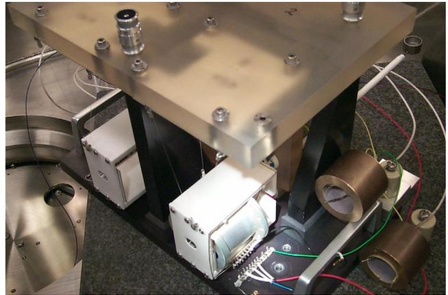
Figure 11 – FEFP-5 installed on the thrust stand
