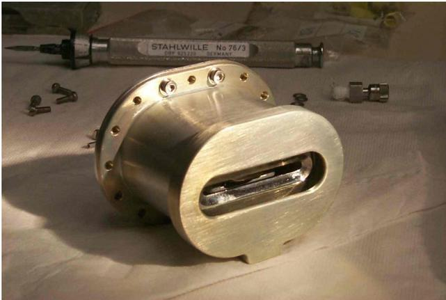
Figure 10 – Alta FEFP-5 model for thrust measurements on the NPL thrust stand
