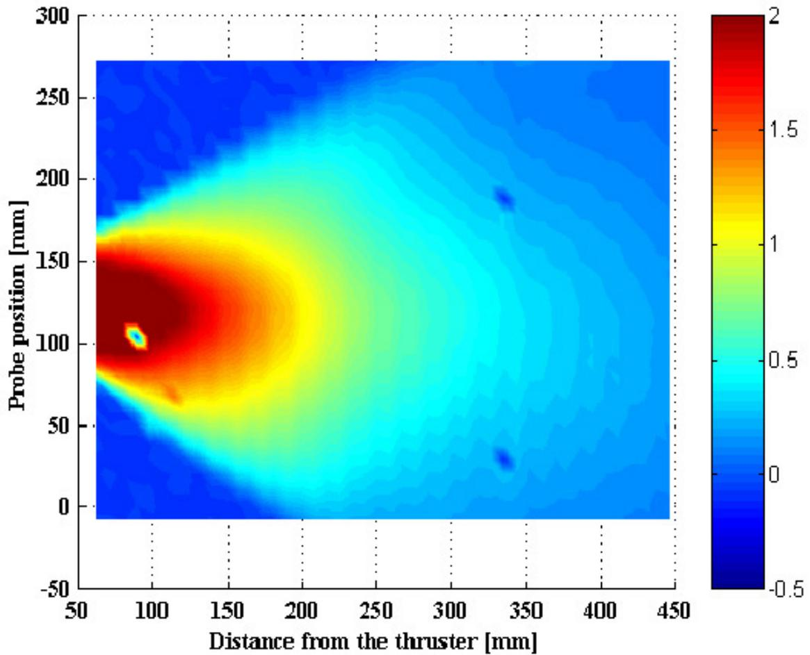
Figure 7 – InFEEP plume scan, top view.
