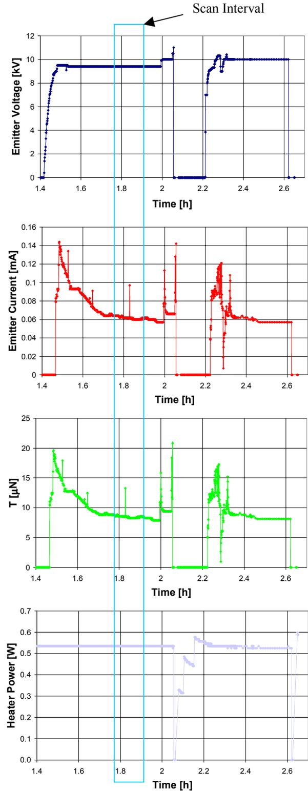
Figure 4 – Scan interval, main operative parameters
