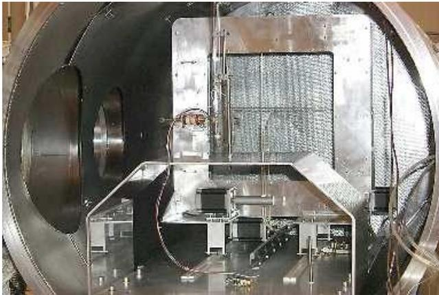
Figure 2 – Diagnostic system installed in the vacuum chamber
