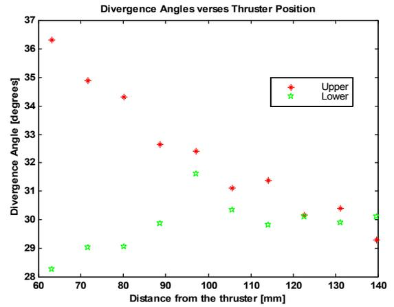
Figure 6 – Beam divergence angle calculation
