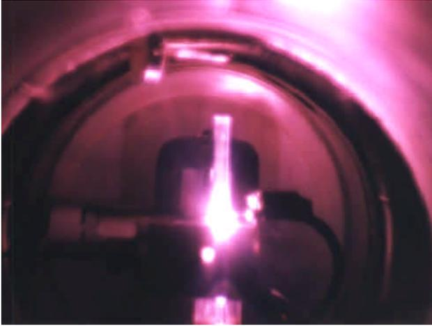
Figure 5 - The atomic oxygen source in operation.
