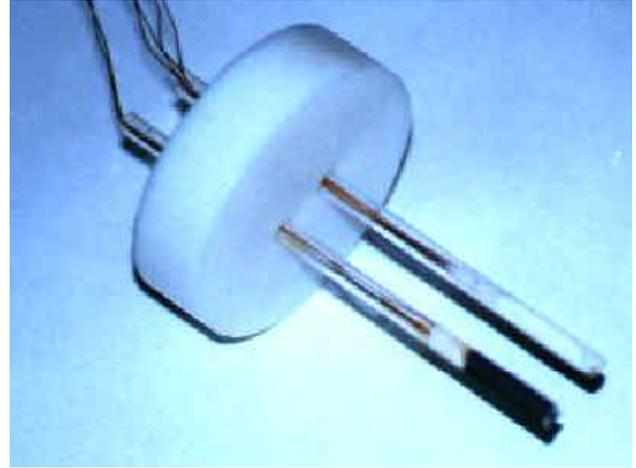
Figure 6 - Atomic oxygen flux measurement probe
