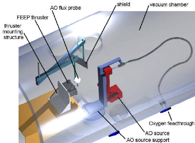
Figure 10 - Schematics of the Atox test setup
