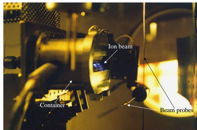
Figure 8 - The 1 mN FEEP thruster firing prior to Atox test
