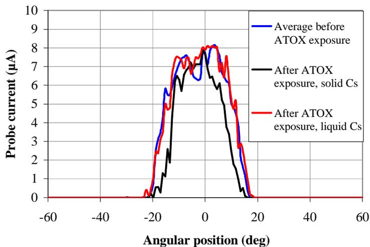
Figure 15 - Comparison of average ion beam profiles before and after exposure to atomic oxygen
