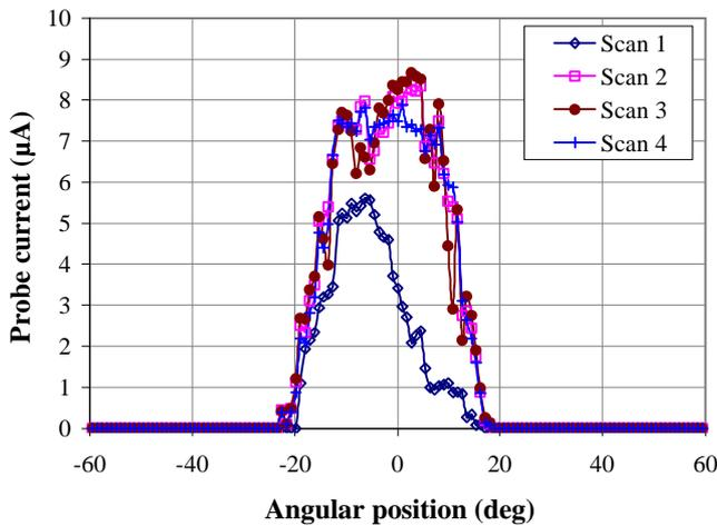
Figure 14 - Ion beam profiles along the slit after the Atox test, second period
