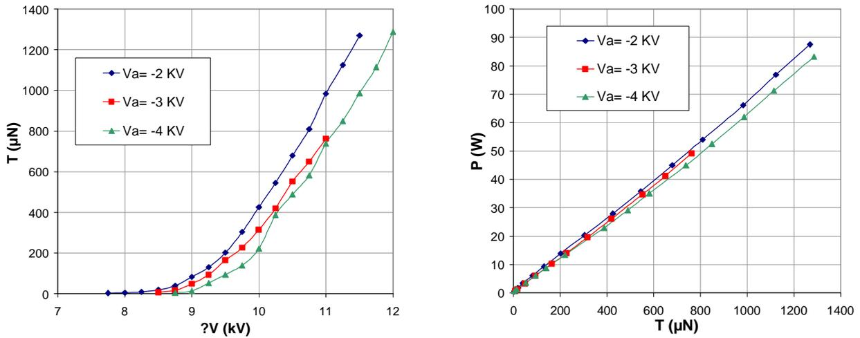
Figure 9 - Thruster performance curves: left, thrust vs. total electrode voltage; right, emitter power consumption vs. thrust.  $V_a$  is the accelerator voltage.
