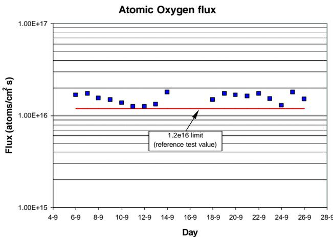
Figure 11 - Measured atomic oxygen flux during the Atox test
