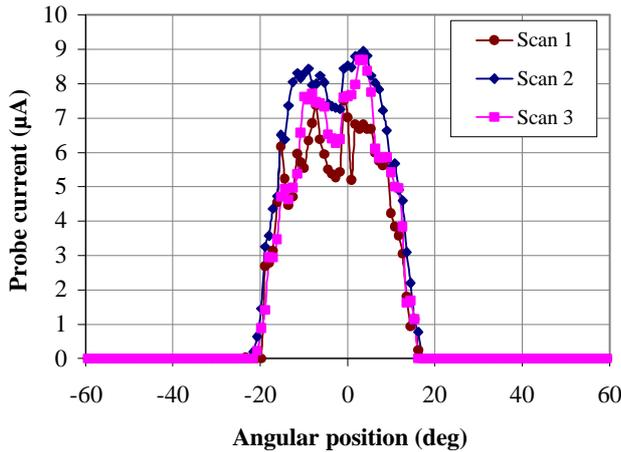
Figure 12 - Ion beam profiles along the slit before the Atox test
