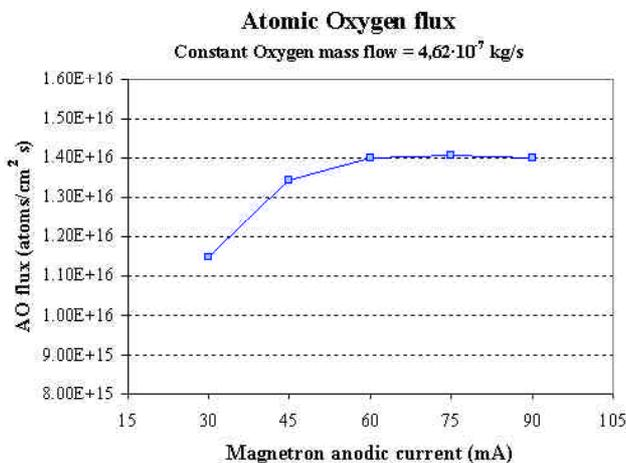
Figure 7 - Atomic Oxygen flux vs. magnetron current
