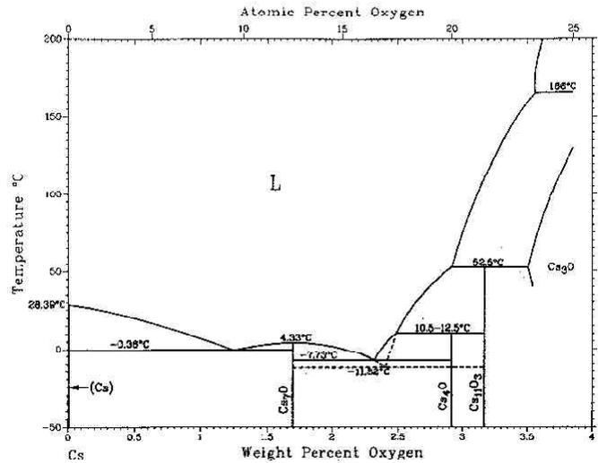
Figure 3 - Cesium-Oxygen phase diagram [4]
