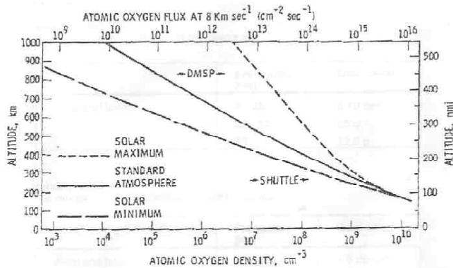
Figure 2 - Atmospheric Atomic Oxygen density in Low Earth Orbit (from [12])
