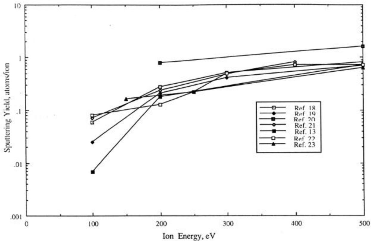
Fig. 1. Compilation of sputtering yields of xenon-molybdenum.
