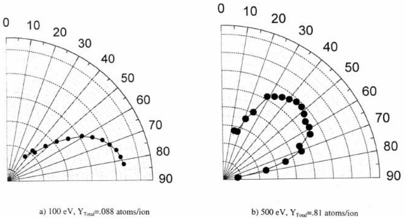
Fig. 4. Polar plot of differential sputtering yields of xenon-tantalum. (Arbitrary scale)
