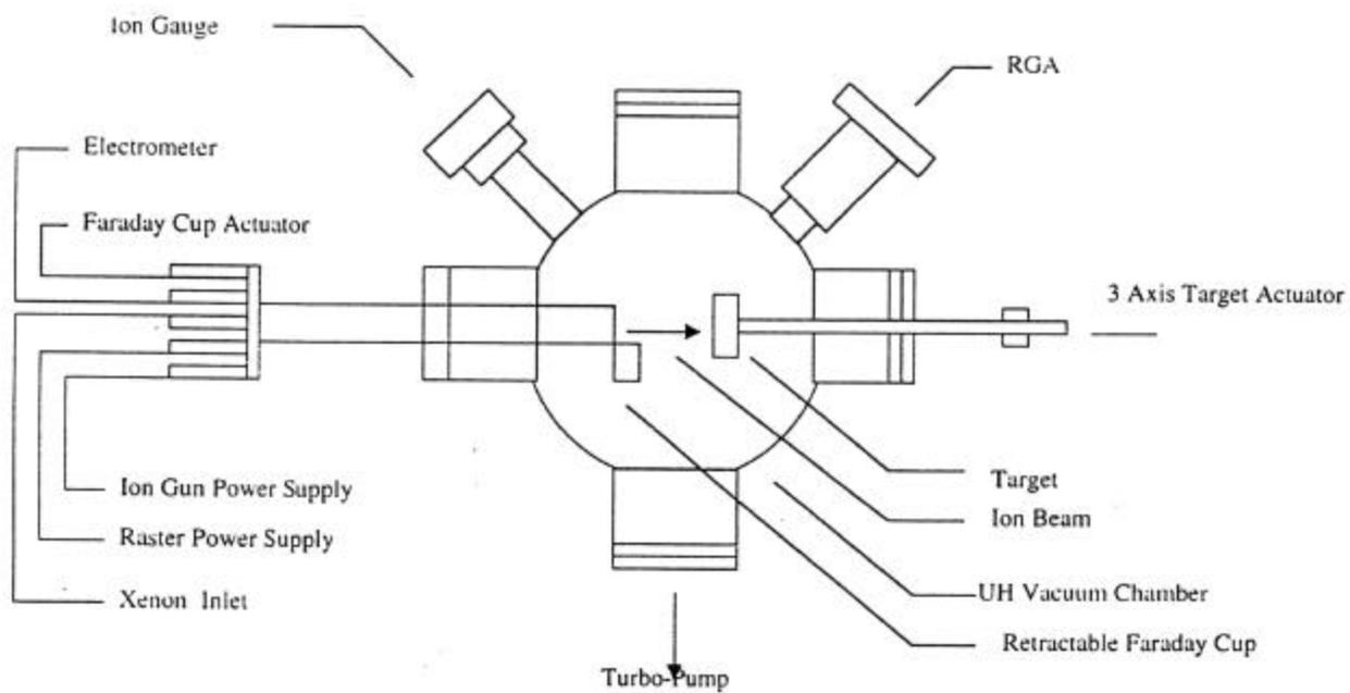
Fig. 2. Schematic of low energy ion sputtering yield measurement apparatus.
