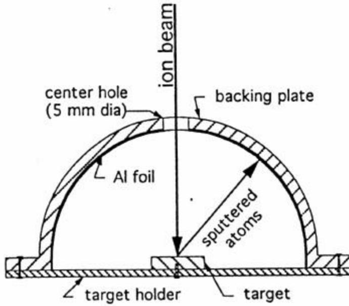
Fig. 3. Schematic of target-collector assembly. (Ref. 13)
