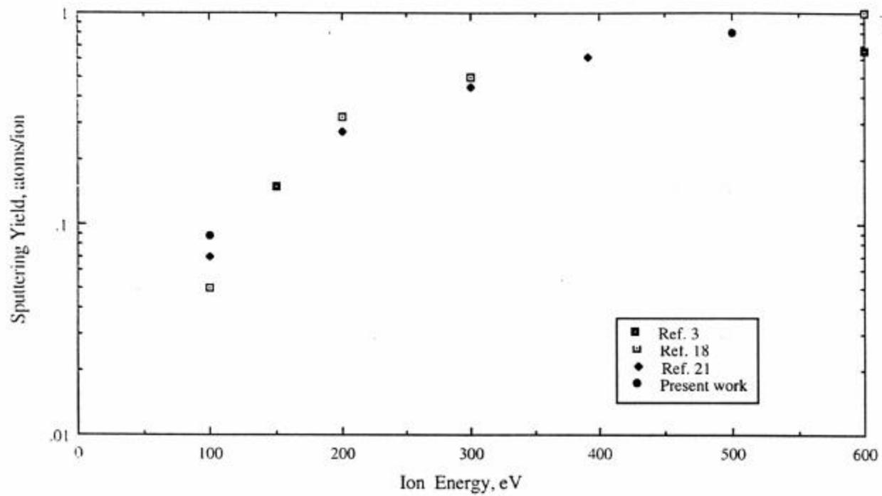
Figure 5. Measured sputtering yield of xenon-tantalum compared to literature data.
