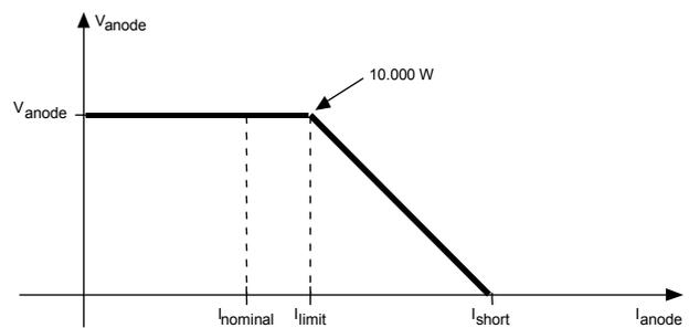
**figure 3 : V – I Anode characteristic**
