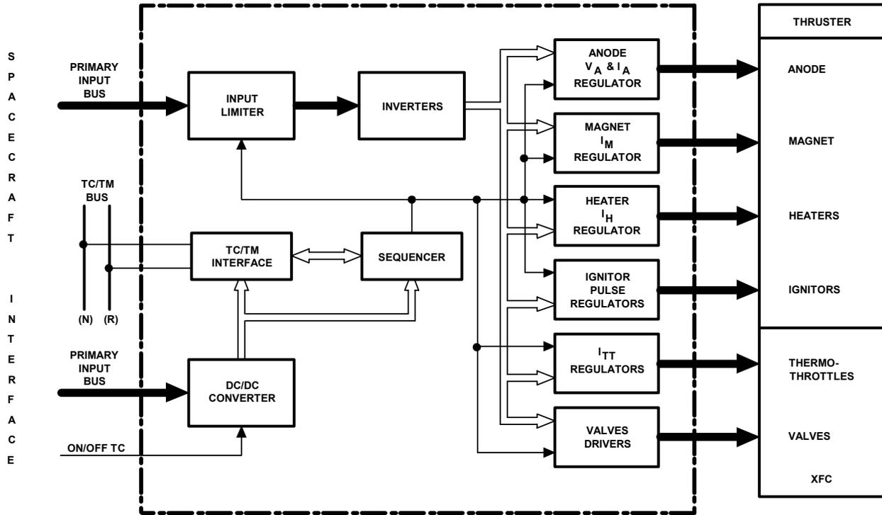
**Figure 1 : PPU functional block**
