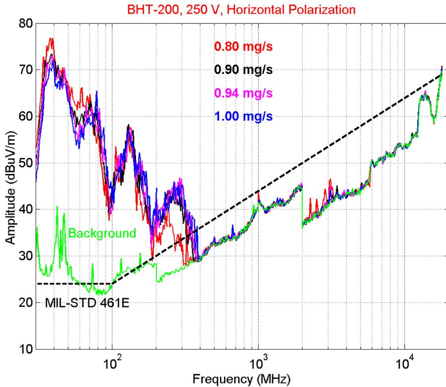
**Figure 9.** BHT-200 radiation at 250 V and four anode flow rates, horizontal polarization.
