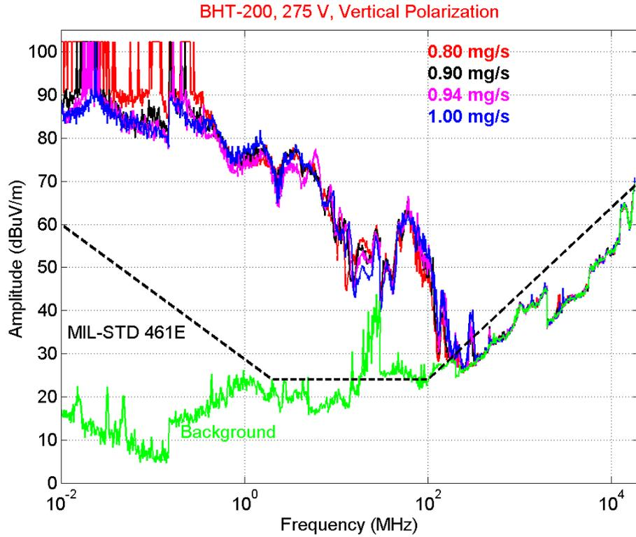
**Figure 6.** BHT-200 radiation at 275 V and four anode flow rates, vertical polarization.
