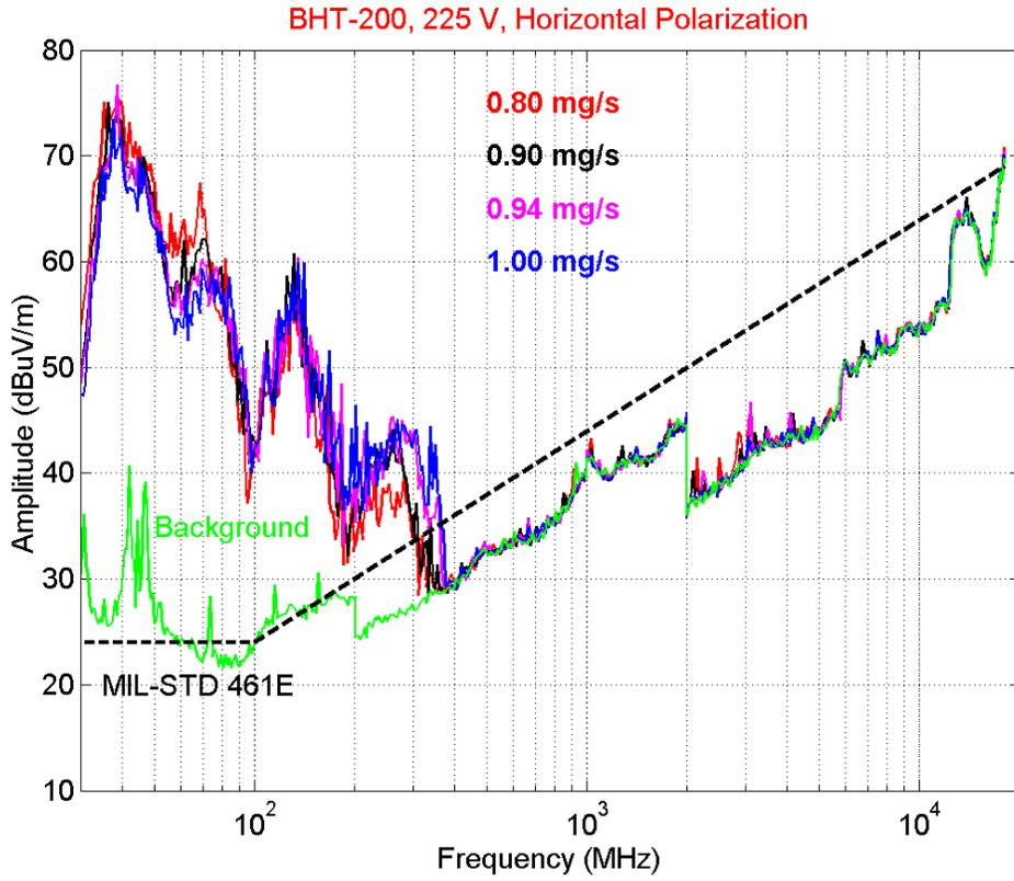
**Figure 8.** BHT-200 radiation at 225 V and four anode flow rates, horizontal polarization.
