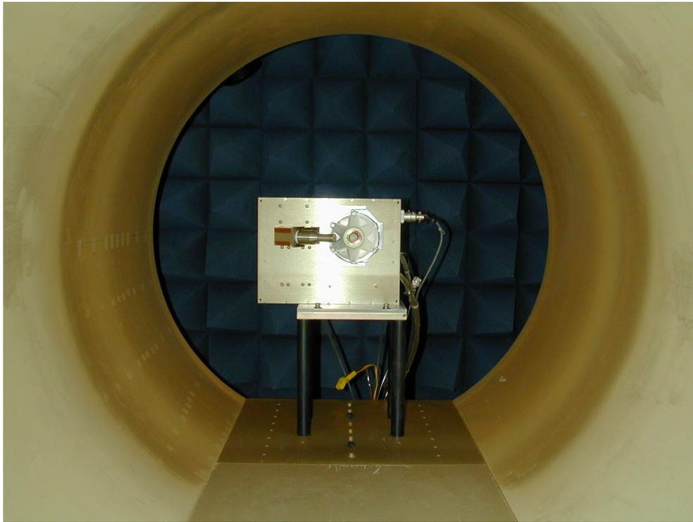
**Figure 2.** BHT-200 on water cooled aluminum mounting plate with filter box behind the thruster. The back of the fiberglass tank is removed allowing the absorbing pyramids in the anechoic room to be seen.
