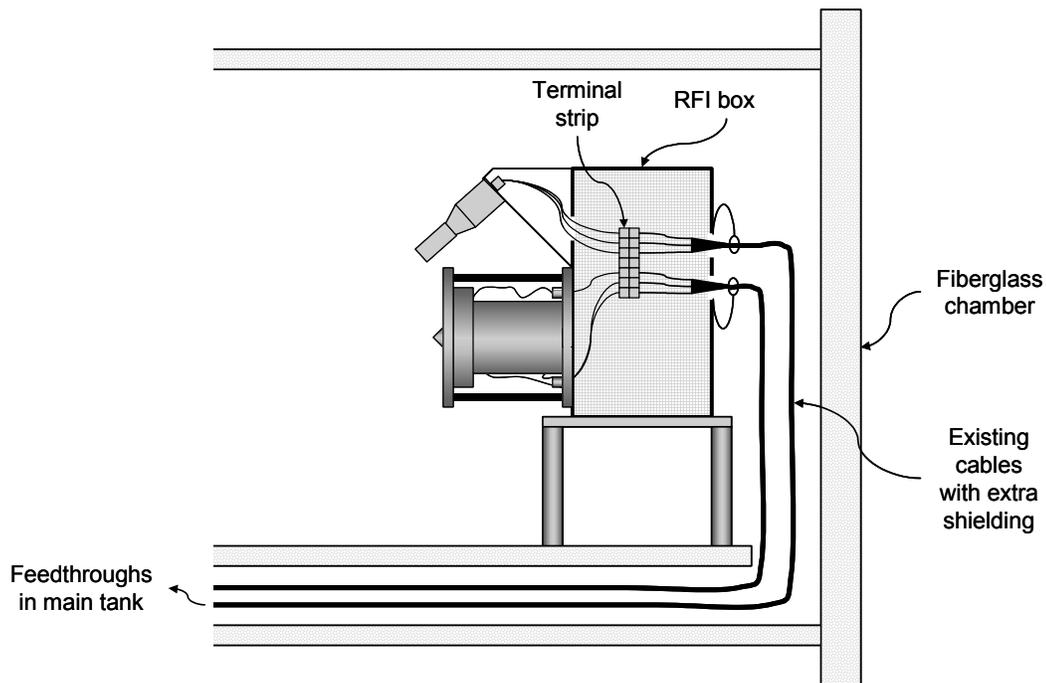
**Figure 3.** Shielding configuration for the BHT-200 tests. Filter components in the RFI box are not shown.
