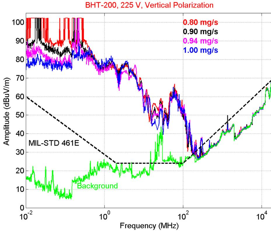
**Figure 4.** BHT-200 radiation at 225 V and four anode flow rates, vertical polarization.
