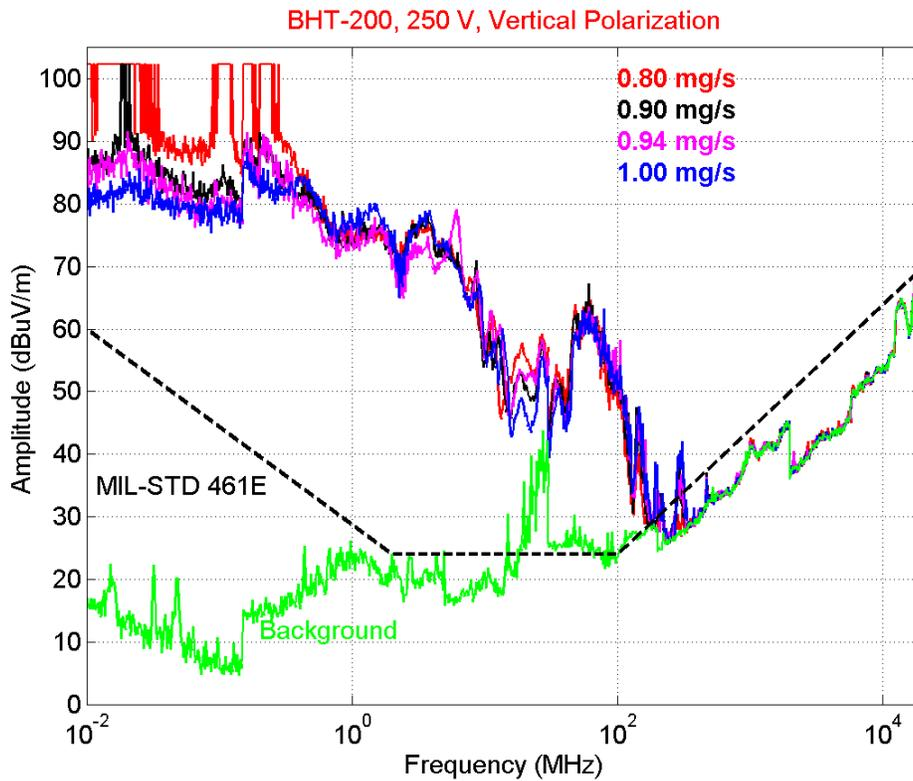
**Figure 5.** BHT-200 radiation at 250 V and anode flow rates, vertical polarization.
