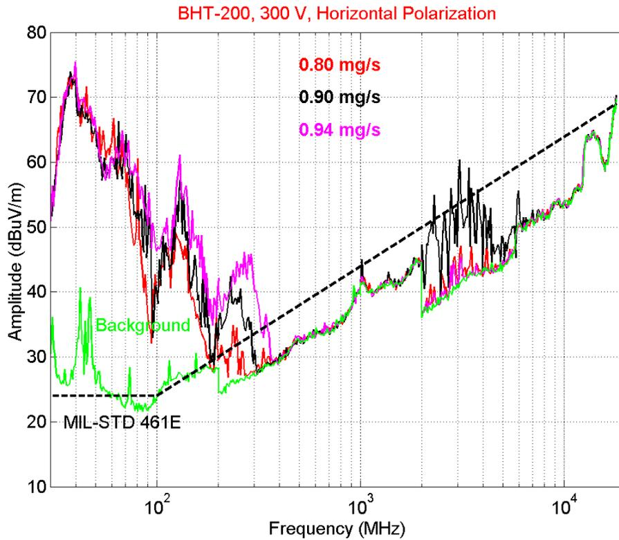
**Figure 11.** BHT-200 radiation at 300 V and four anode flow rates, horizontal polarization.
