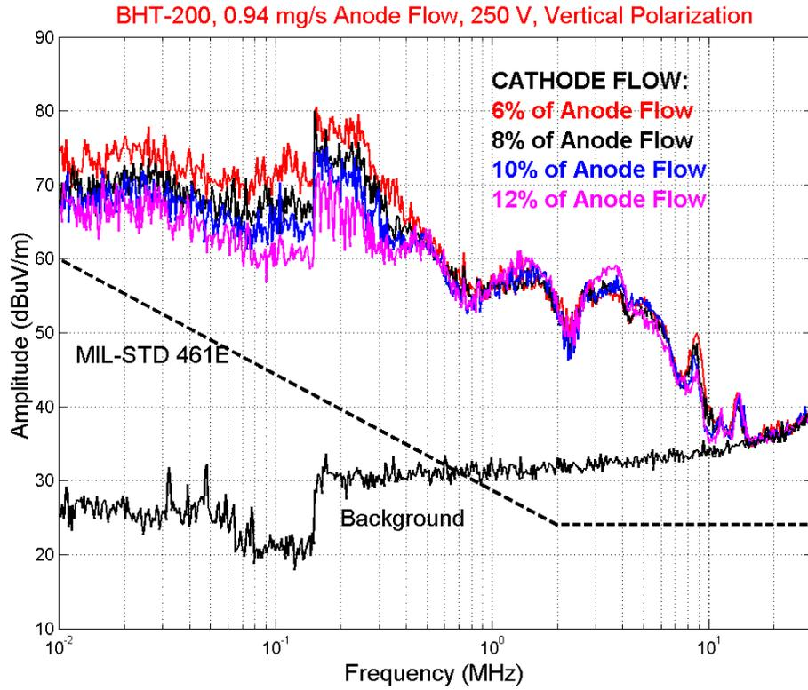
Figure 12. BHT-200 radiation at 250 V and four cathode flow rates, vertical polarization.
