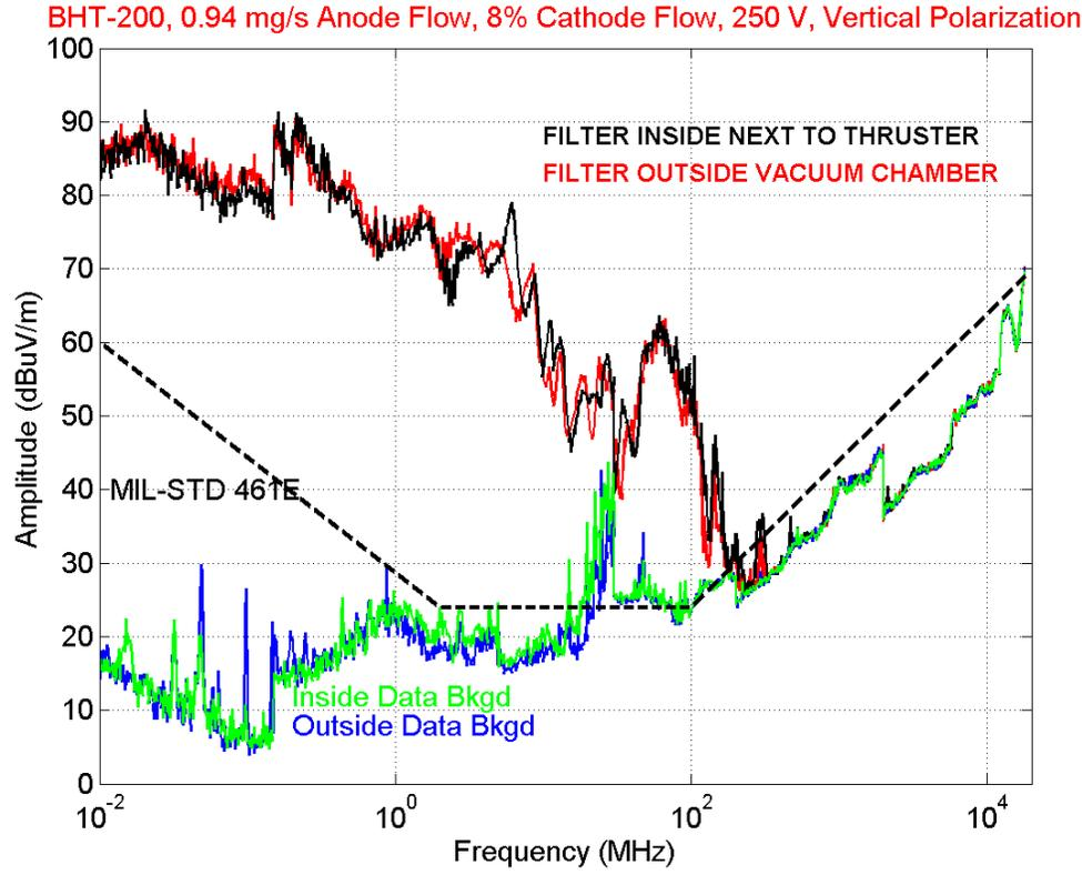
Figure 13. BHT-200 radiation at 250 V for two filter positions, vertical polarization.
