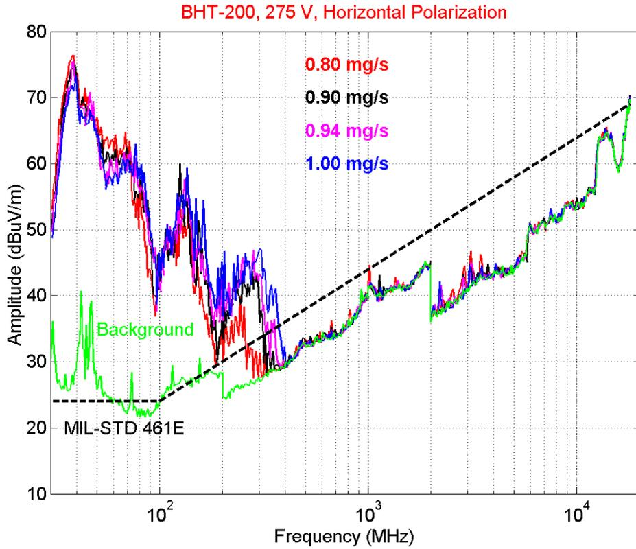
**Figure 10.** BHT-200 radiation at 275 V and four anode flow rates, horizontal polarization.
