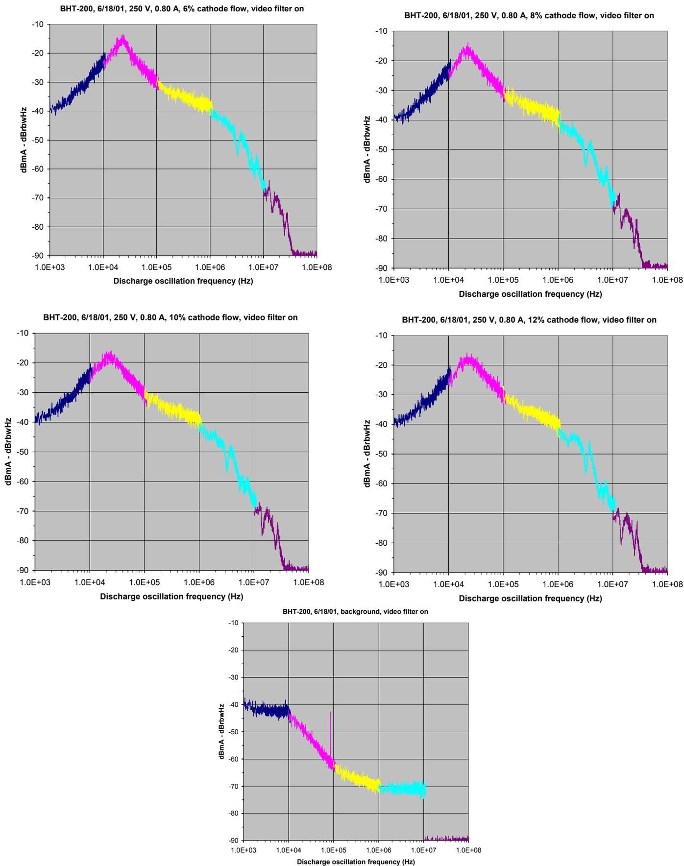
**Figure 20.** Spectra of BHT-200 current oscillations for four cathode flows. Bottom plot is power off background.
