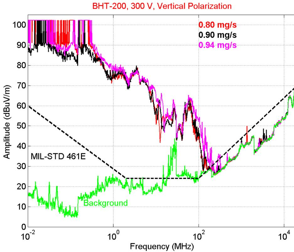
**Figure 7.** BHT-200 radiation at 300 V and four anode flow rates, vertical polarization.
