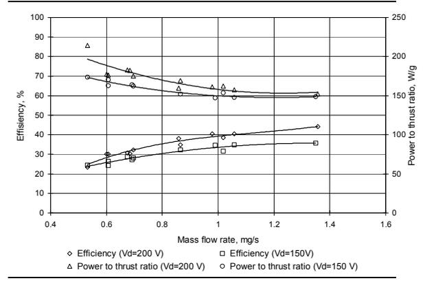
**Fig. 6. Performances of T-27 thruster versus mass flow rate.**
