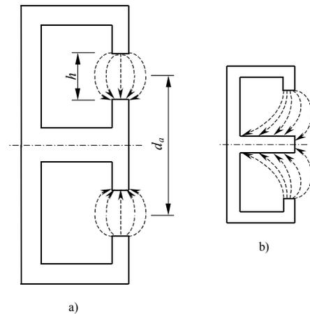
**Fig. 2. Schemes of traditional (a) and microTAL (b) magnetic system.**
