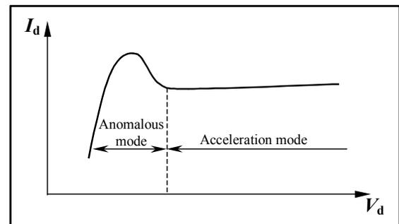
Fig. 1. TAL Volt-Ampere characteristic.
