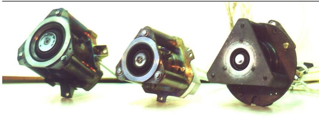
Fig. 5. General view of D-55, D-38, T-27 thrusters (from left to right).
