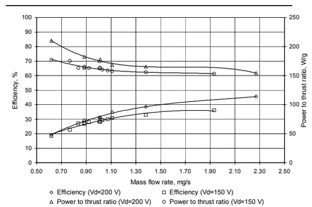
**Fig. 7. Performances of D-38 thruster versus mass flow rate.**
