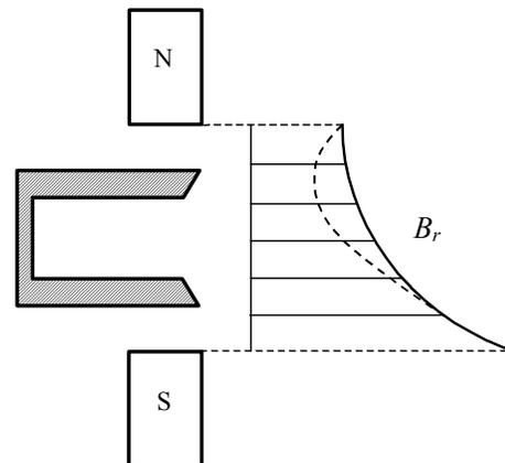
**Fig. 3. Radial distribution of magnetic field.**
