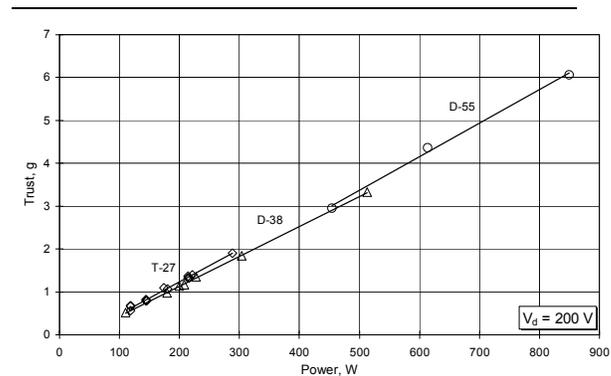
**Fig. 8. Comparable characteristics of T-27, D-38 and D-55 thrusters.**
