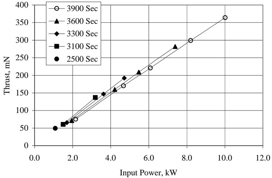
Figure 1 - Estimated thrust and power throttling range for different values of specific impulse.
