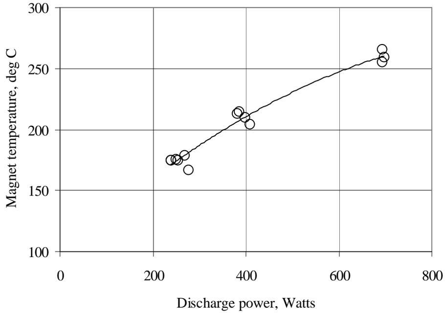
Figure 11 - Magnet temperature versus discharge power.
