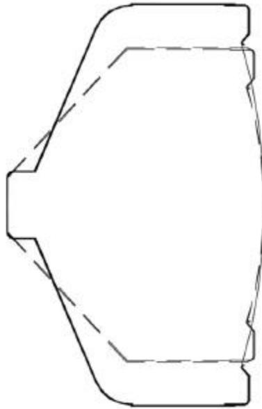
Figure 5 - Superposition of 40 cm engine (solid line) and DS-1 thruster (dashed line) outer mechanical envelope.
