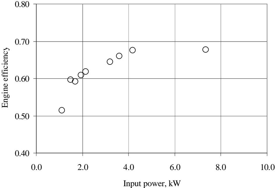
Figure 13 -Engine efficiency versus input power.
