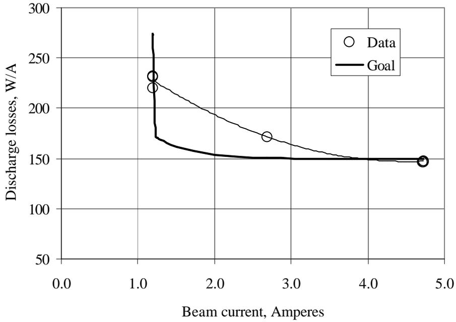
Figure 9 - Discharge losses versus beam current.
