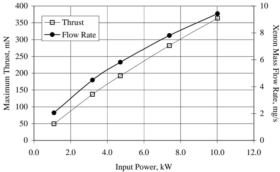
Figure 2 - Estimated thrust and flow rate versus input power to the engine.
