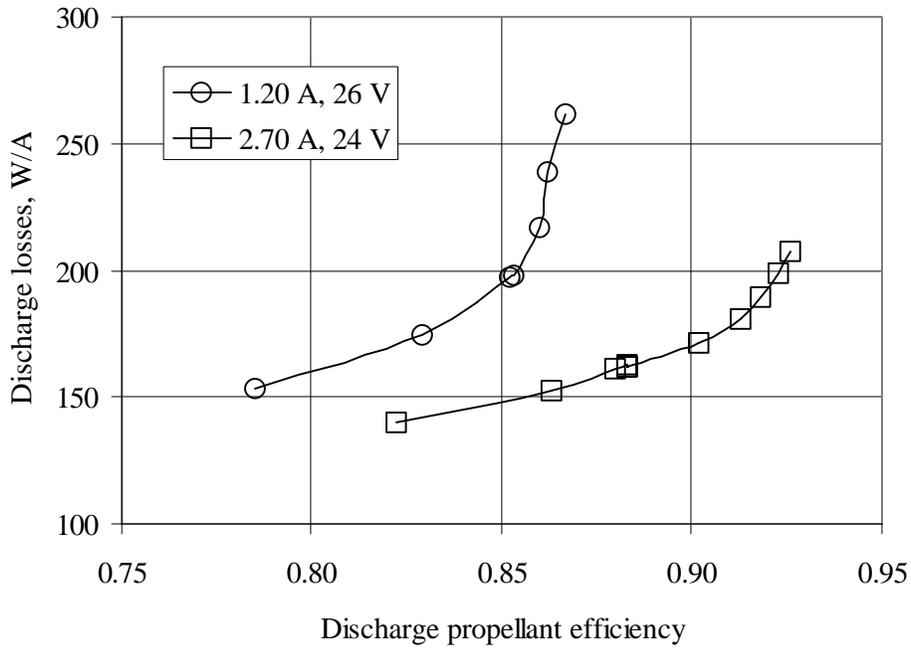
Figure 10 - Discharge losses versus discharge propellant efficiency.
