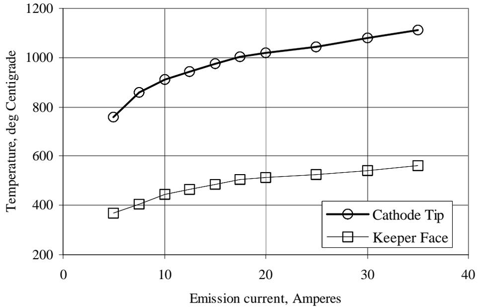
Figure 12 - Cathode temperatures versus emission current; 40 cm thruster discharge cathode.
