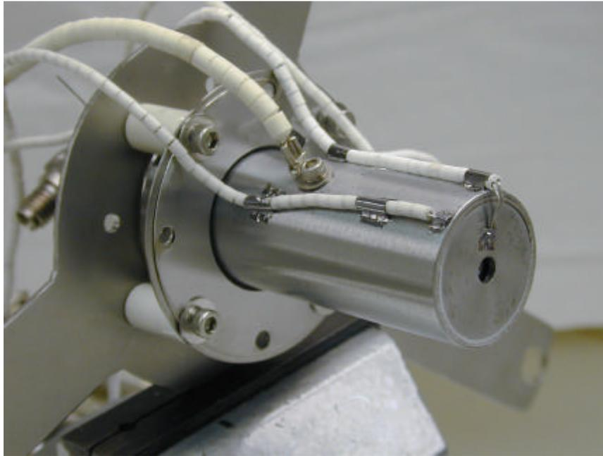
Figure 7 - Prototype discharge cathode assembly for 40 cm engine.
