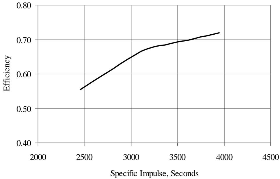
Figure 3 - Estimated thruster efficiency versus specific impulse at maximum thrust.
