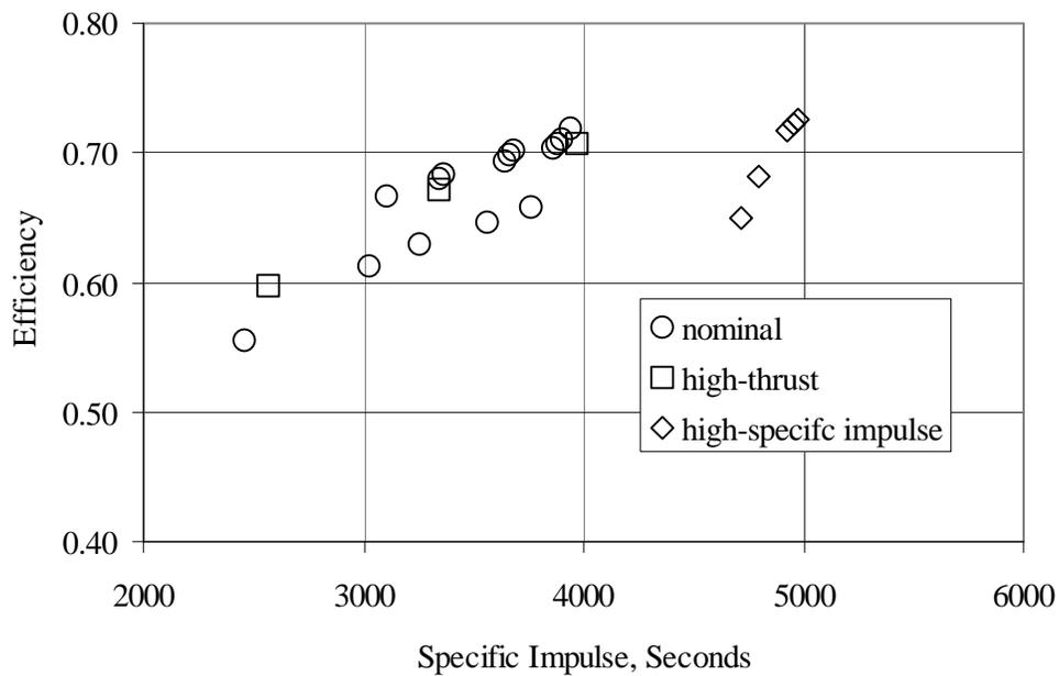
Figure 4. - Thruster efficiency versus specific impulse for various throttling strategies.
