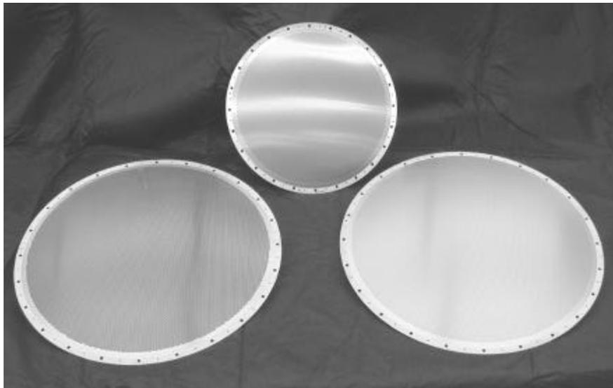
Figure 8 - Photograph of 40 cm screen grid (left foreground) and 40 cm accelerator grid (right foreground) with a 30 cm accelerator grid (center background) for comparison.
