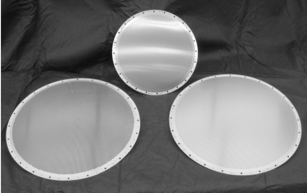
Fig. 7. Photograph of 40 cm screen grid (left foreground) and 40 cm accelerator grid (right foreground) with a 30 cm accelerator grid (center background) for comparison.
