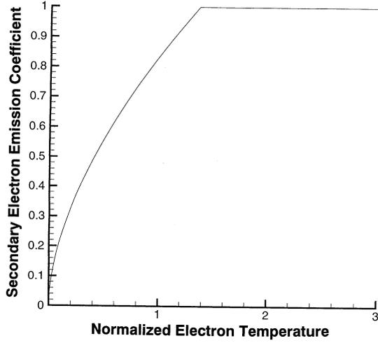
(a) Secondary electron emission coefficient.
