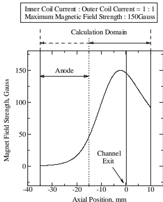
Fig.5 Axial variation in magnetic field strength in acceleration channel of THT-IV Hall thruster.
