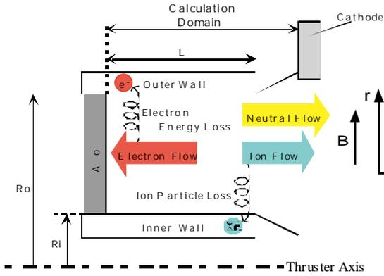
Fig.1 Calculation model of one-dimensional Hall thruster flowfield.
