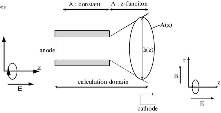
Fig.2 Calculation model of quasi-one-dimensional exhaust plasma plume.
