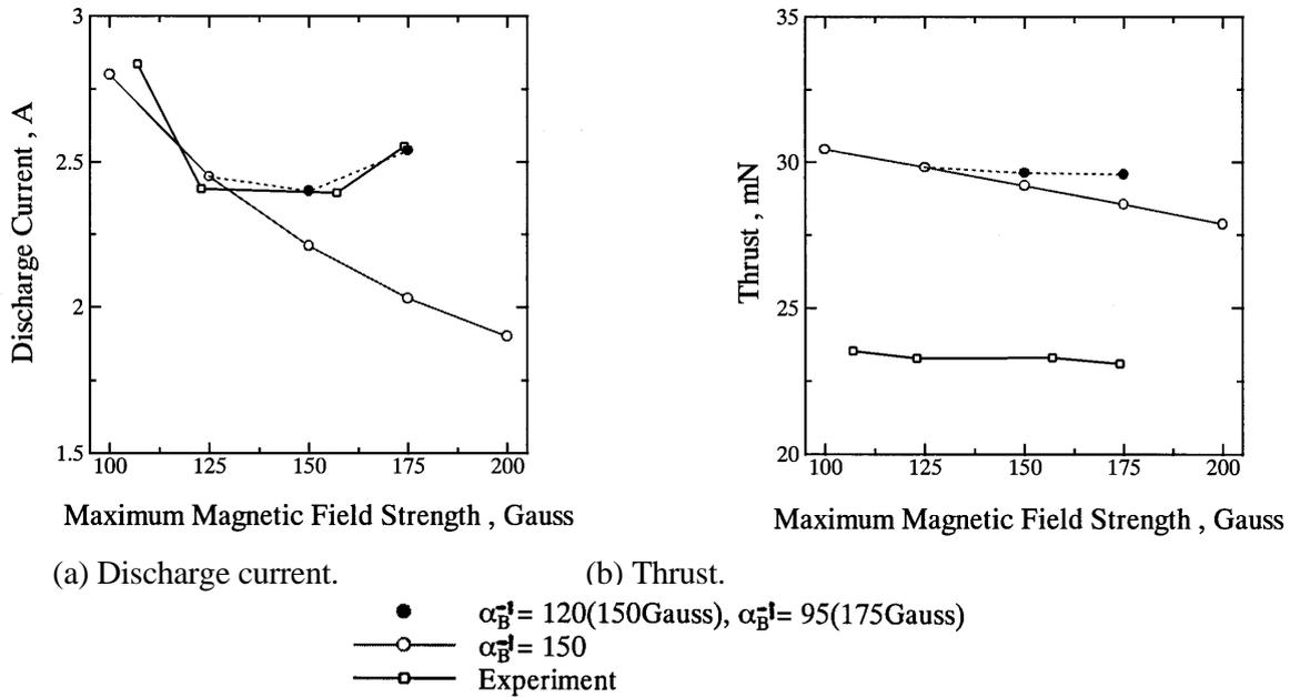
Fig.14 Comparison between calculated and measured operational characteristics as varying Bohm diffusion coefficient with acceleration channel length of 30 mm at discharge voltage of 200 V and corresponding mass flow rate of 2 mg/s.
