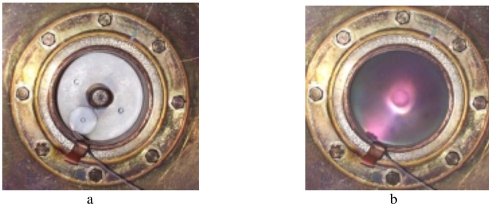
Figure 1. Coaxial APPT. a- face view, b – photo of the discharge in the APPT.
