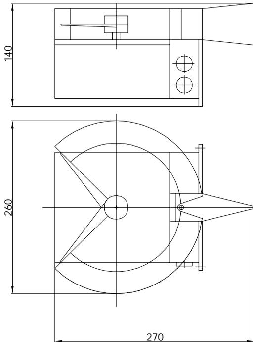
The OCPS consisting of 4 thrusters will have mass close on 21 kg at dry mass near 17 kg. In Figure 4 the dimensional scheme of APPT-150 for SSC orbit maintenance is presented.
