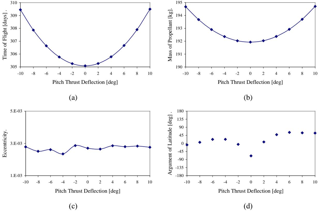
Figure 4. Mission performances for thrust misalignment in pitch axis
