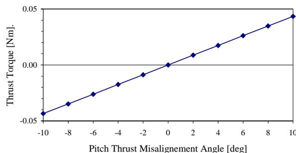
Figure 3. Thrust torque for a range of thrust misalignment angle in pitch
