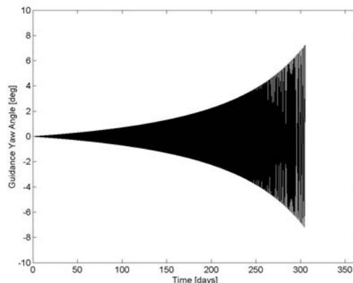
Figure 1. Guidance profile of the Constant/Cosine guidance method
