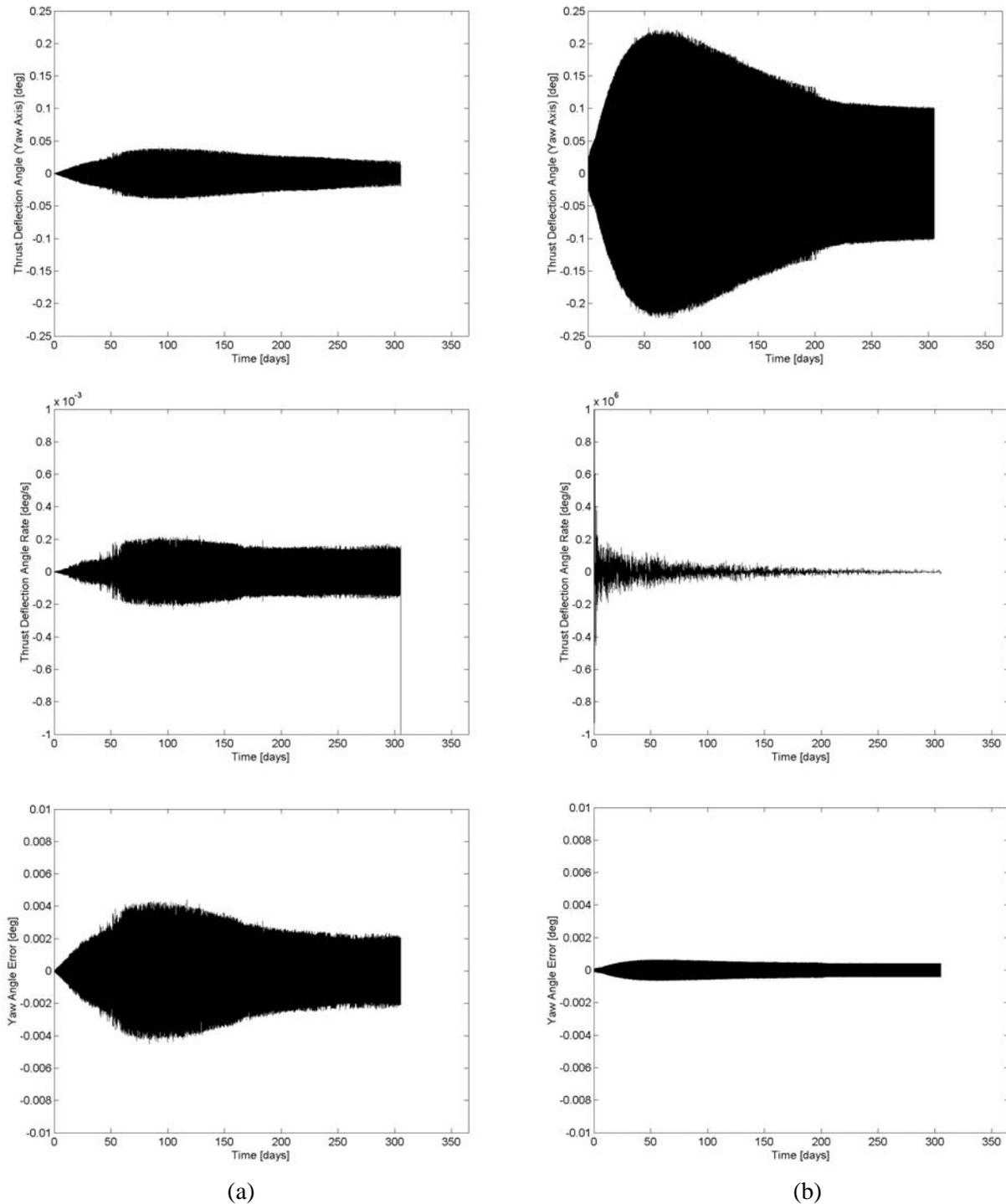
Figure 5. History of Thrust Deflection Angle, Deflection Angle Rate and Attitude Error for (a) the Cosine Guidance and (b) the ICE Guidance
