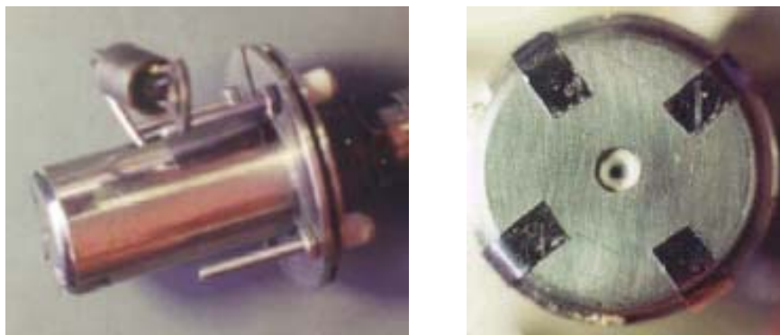
Fig. 2 Cathode and keeper assembly with close-up view of keeper and cathode orifices.
