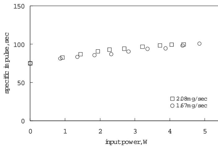
Fig.5 Input power vs specific impulse.
