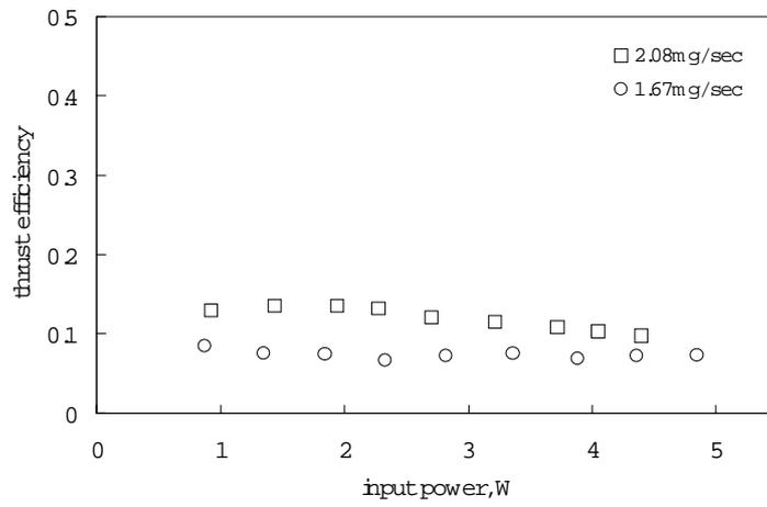
Fig.6 Input power vs thrust efficiency.
