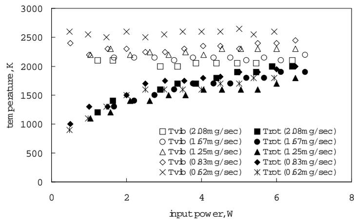
Fig.8 Input power vs heavy particle temperature.
