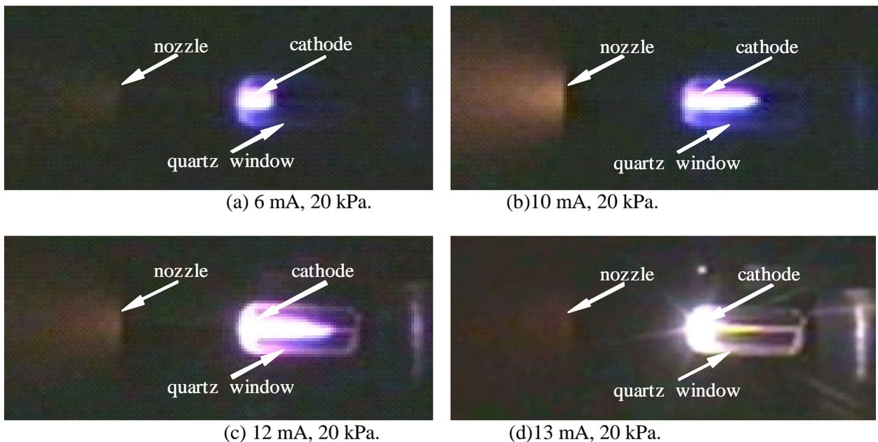
Fig.2 Photos of discharging plasmas in thruster.
