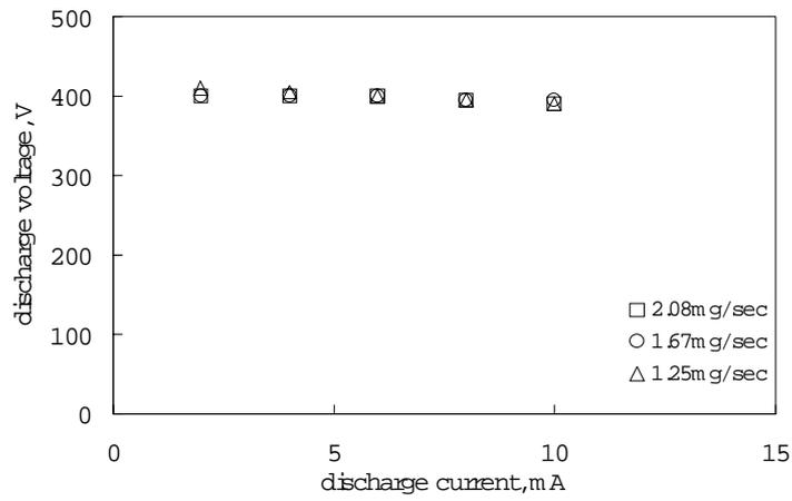
Fig.3 Discharge current-voltage characteristics.
