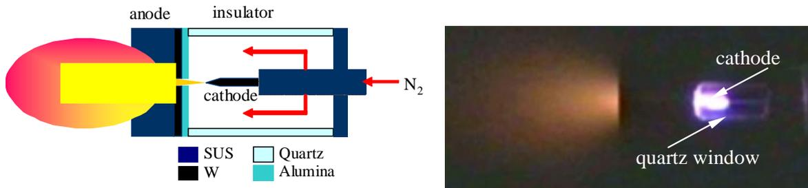
(a) Schematic of an arcjet thruster. (b) Photo of an arcjet thruster in operation.
