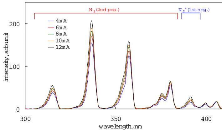
Fig.7 Typical spontaneous emission spectra from interior plasma of arcjet.
