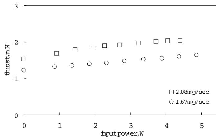
Fig.4 Input power vs thrust.
