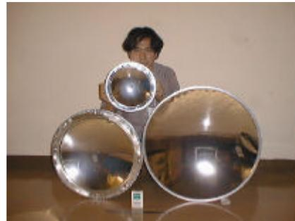
**Fig. 2** EMCs of 220 mm, 430 mm, and 640 mm in diameter
