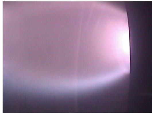
**Fig. 2: ATTILA operating with superposed induction heating**
