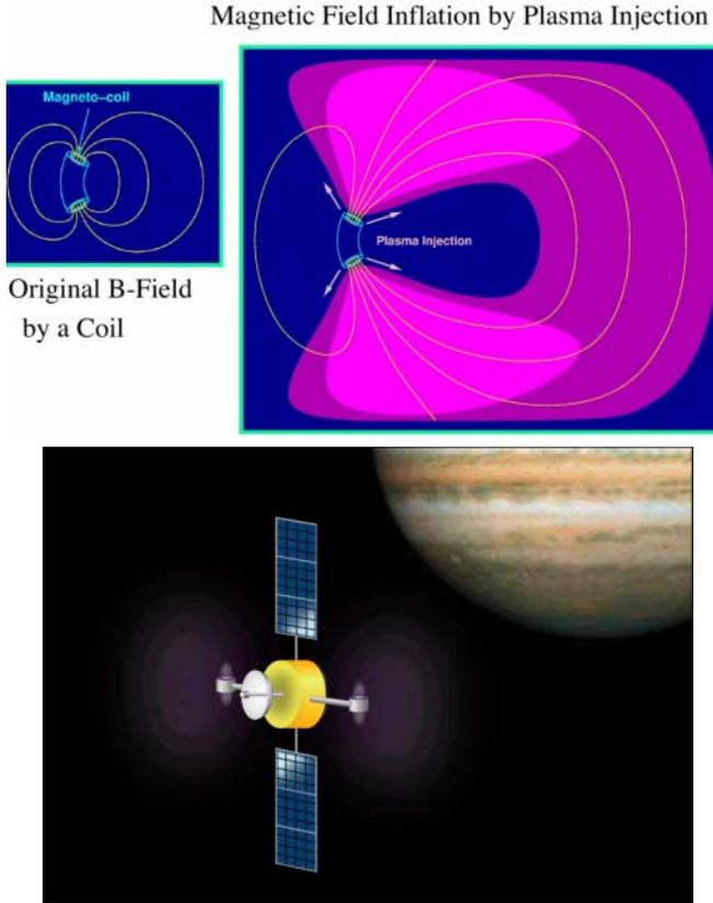
Fig. 2 Principle of magnetoplasma sail and image of a spacecraft propelled by magnetoplasma sail.
