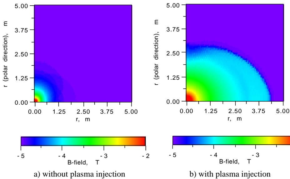
Fig.6 Inflation of magnetic field; magnetic flux density distribution at  $t=0.22\text{ms}$  after plasma injection; logarithmic scale.
