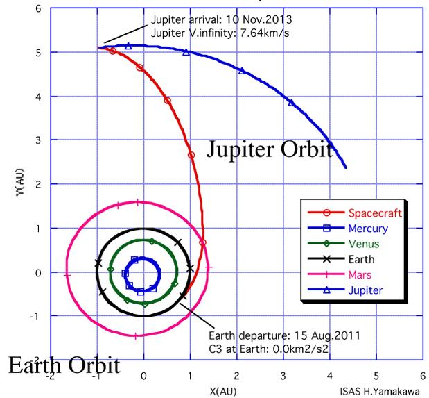
**Fig. 9 Application of a magnetoplasma sail to a deep space mission; trajectory to Jupiter.**
