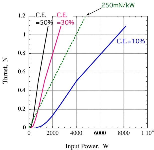
Fig. 3 Thrust to power ratio of magnetoplasma sail obtained from the electric power required to expanded the magnetic field.
