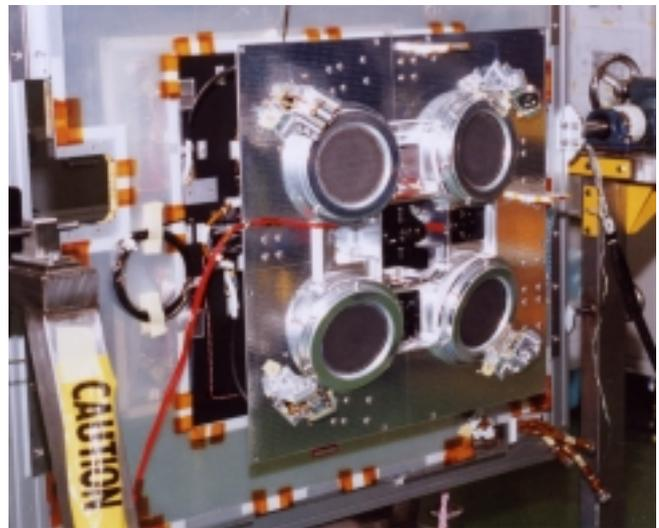
Fig. 11 FM ion thrusters mounted on a gymbal plate.
