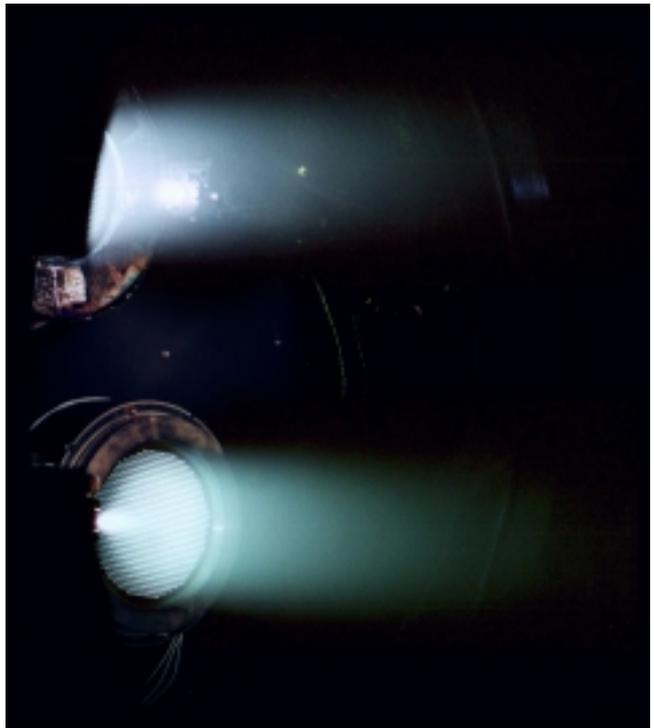
Fig. 4 Simultaneous operation of 2 microwave ECR ion engines inside a vacuum chamber.
