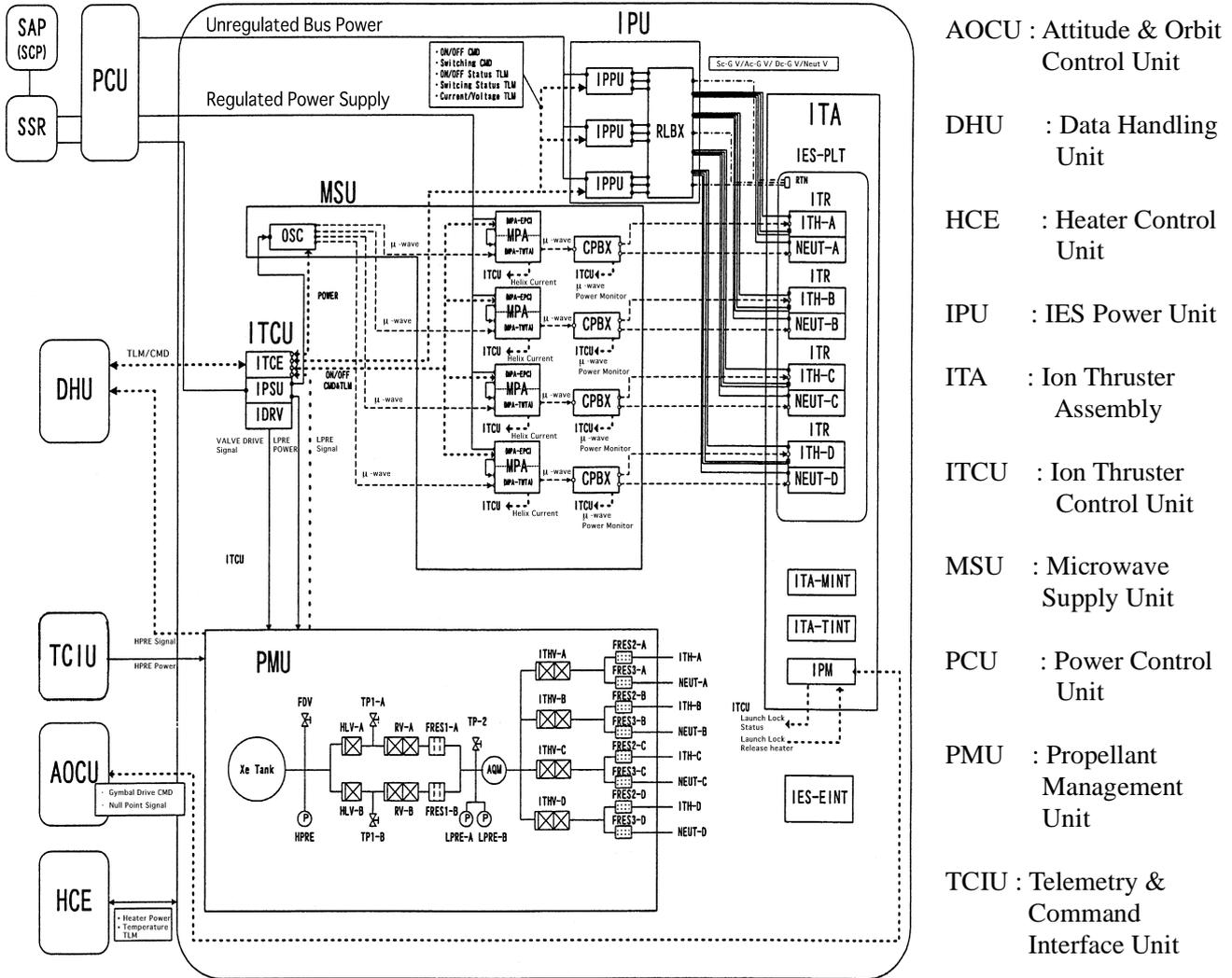
Fig. 5 IES system block diagram.
