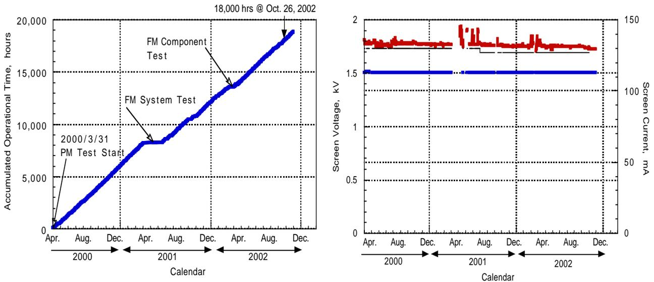
Fig. 9 PM-phase endurance test history (Left: Accumulated operation time vs. calendar, Right: Screen voltage & current vs. calendar).
