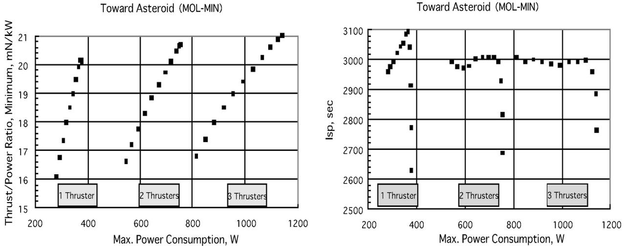
Fig. 8 Thrust performance required from the orbit planning (Left: Thrust/Power ratio, Right: Specific Impulse vs. power consumption for 1 – 3 thrusters simultaneous operation) at MOL.
