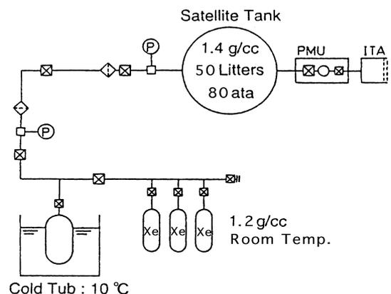
Fig. 12 Xe loading unit (Left) and schematic of liquefaction loading (Right).
