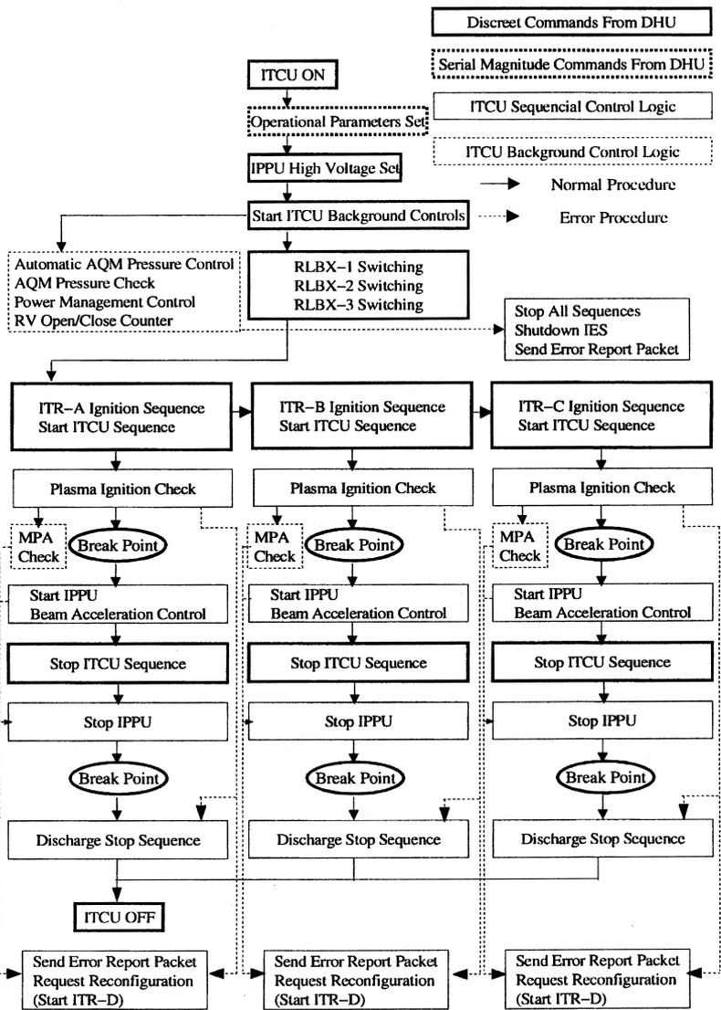
Fig. 6 IES operational command sequence and hardware logic.
