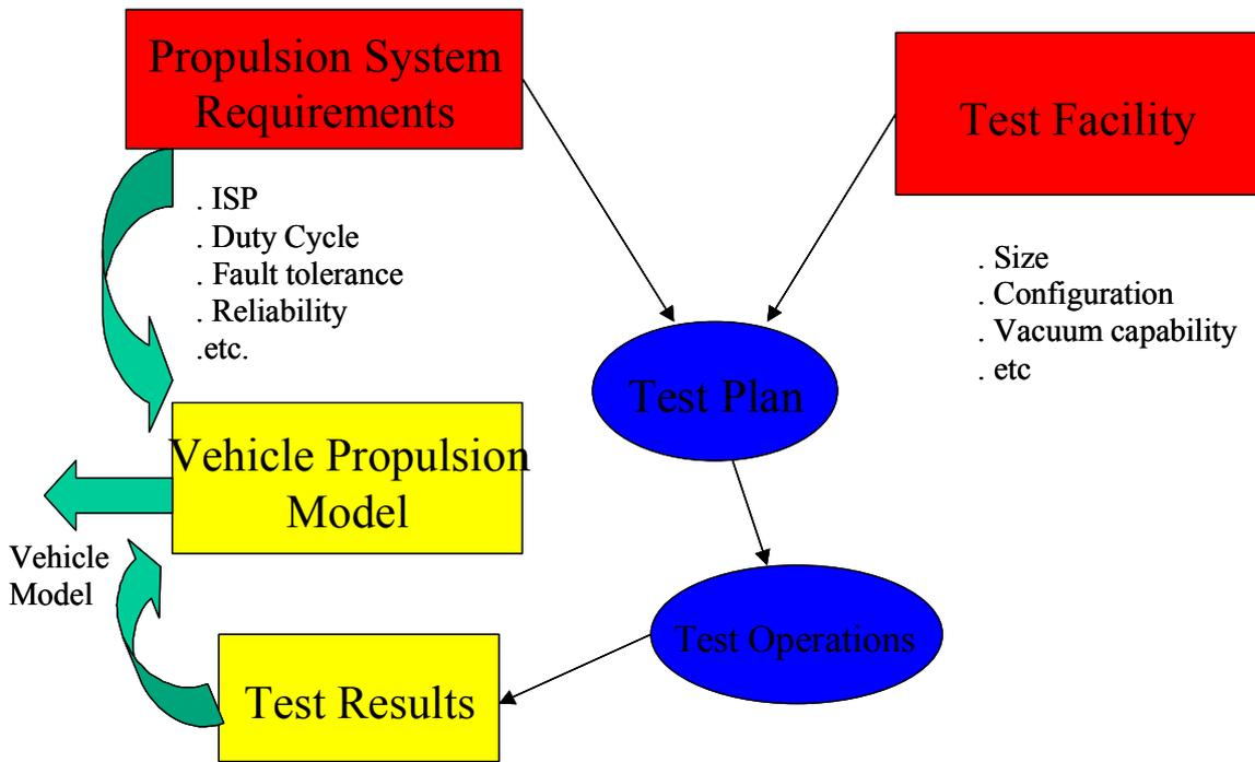
**Figure 5 Ground Test Flow**
