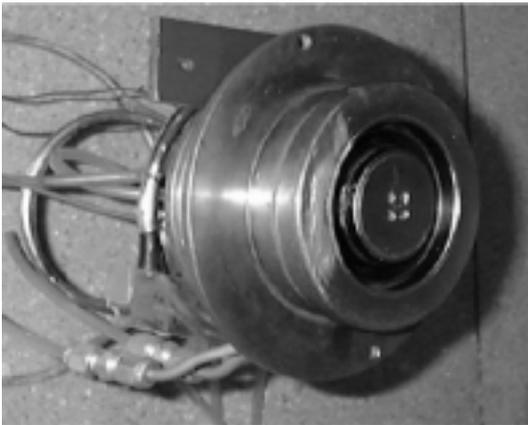
Fig. 3 A 1kW class anode-layer Hall Thruster.
