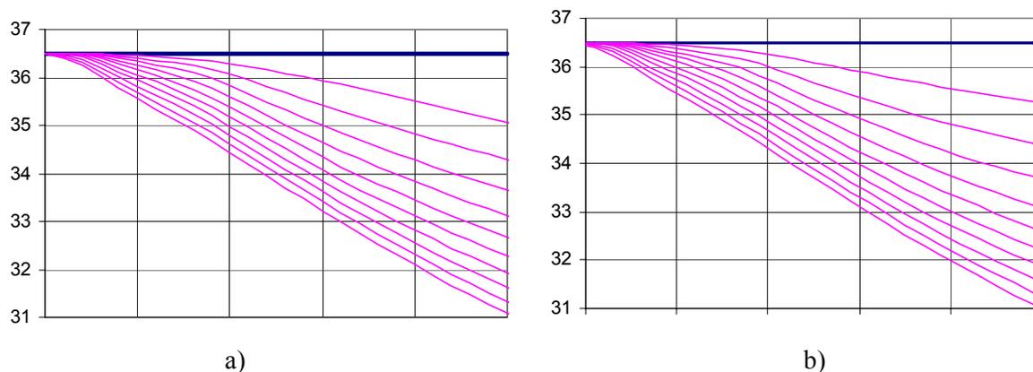
Fig. 2. The forecast of the X-85M inner insulator profile changing during 1000 hours (profiles are shown with 100 hours timestep) at discharge voltage a) 300 V, b) 670 V.
