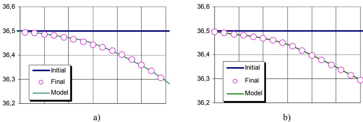
Fig. 1. X-85M inner insulator profile changing after 25 hours of operation at discharge voltage a) 300 V, b) 670 V.
