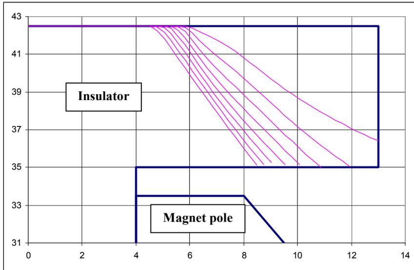
Fig 3. The forecast of KM-100 inner insulator profile changing during 8000 hours (profiles are shown with 1000 hours timestep).
