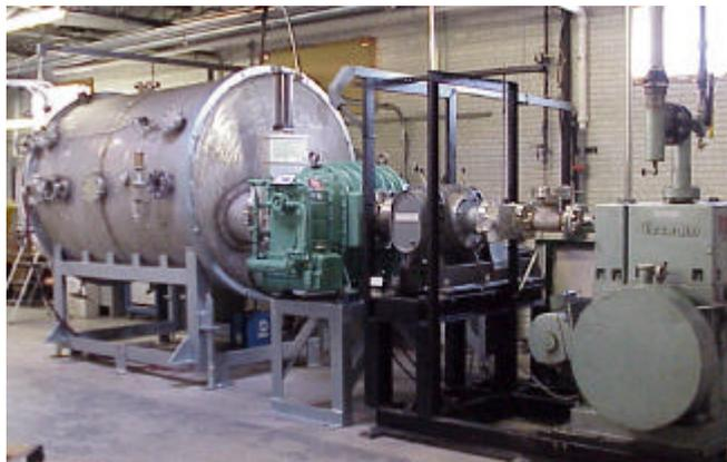
**Figure 2 Busek's arcjet facility showing pumping system.**
