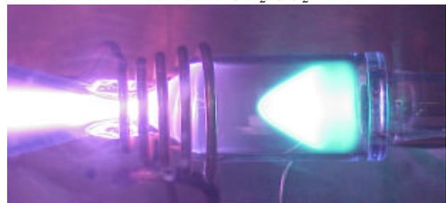
**Figure 18 Simulated MMH/NTO laboratory RF Arcjet, coil at throat.**
