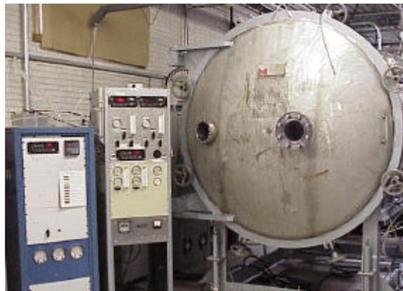
**Figure 3 Front view of arcjet facility & control cabinets.**
